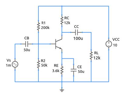
Shown in the figure is a common-emitter amplifier. We are interested in computing the mid-band gain of the amplifier. Assume that the BJT is working in the active mode.
