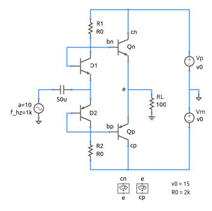
Shown in the figure is a Class AB amplifier which has higher efficiency than a Class A amplifier. Furthermore, it does not exhibit cross-over distortion, which is a drawback of a Class B amplifier. The input to this amplifier is  $V_i = V_m \sin \omega t$ , and the BJTs have  $\beta = 50$ . The transistors marked as D1 and D2 are used as diodes and can be assumed to have a voltage drop of 0.7 V when conducting.
