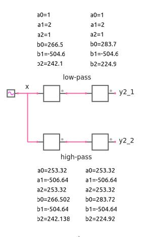
Shown in the figure are  $4^{\text{th}}$ -order low-pass and  $4^{\text{th}}$ -order high-pass digital Butterworth filters. Starting with the analog normalised filter function, the z-domain digital filter function can be obtained as follows.
