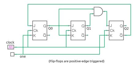
We are interested in the sequence produced by the synchronous counter shown in the figure, starting with the initial state  $Q_2Q_1Q_0 = 000$ . For this purpose, we can prepare a table in the following format:
