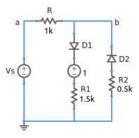
Shown in the figure is a diode circuit example to illustrate the basic operation of diode clipping circuits. Assume the turn-on voltage of the diodes to be 0.7 V.
