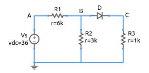
For the diode circuit shown in the figure, assume the turn-on voltage of the diode to be 0.7 V. Exercise Set
