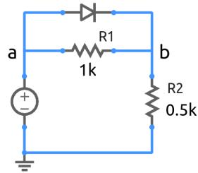
For the diode circuit shown in the figure, assume the turn-on voltage of the diode to be  $0.7\text{ V}$ .
