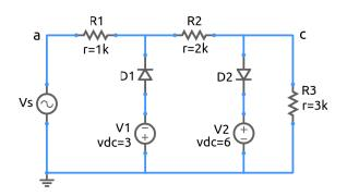
For the circuit shown in the figure, assume the diodes to have a turn-on voltage of 0.7 V. Exercise Set
