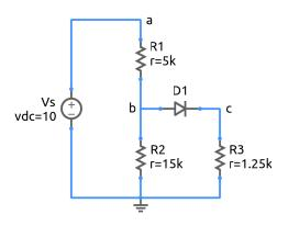
For the diode circuit shown in the figure, assume the turn-on voltage of the diode to be 0.7V. Exercise Set
