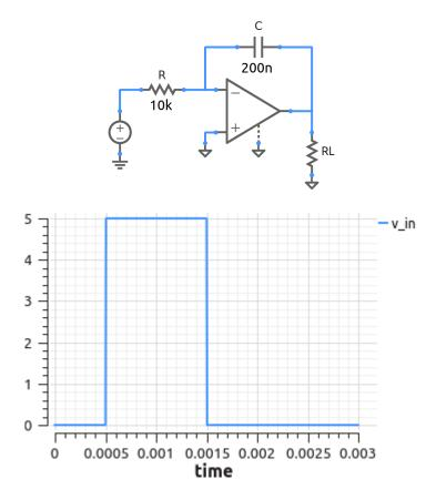
The purpose of this simulation exercise is to understand the response of an Op Amp integrator to an input voltage pulse (as shown in the figure).
