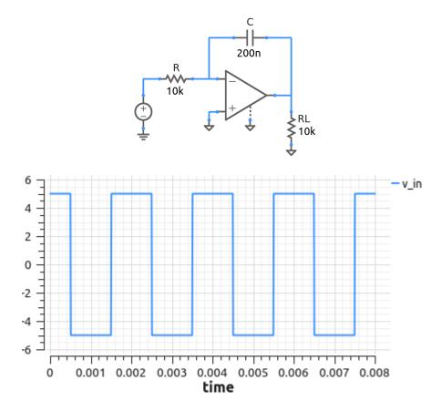
The purpose of this simulation exercise is to understand the response of an Op Amp integrator to a square wave input (as shown in the figure).
