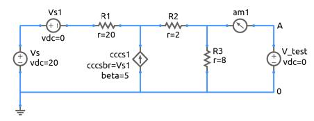
In the circuit shown in the figure, the current through the CCCS is given by  $\beta I_{Vs1}$ . We are interested in finding the Thevenin equivalent circuit as seen from the port A-0.
