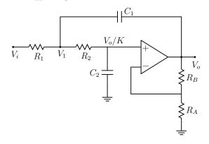
A second-order low-pass filter can be described by [1]  $H(j\omega) = H_{0LP}H_{LP}(j\omega)$ , where  $H_{0LP}$  is a constant, and
