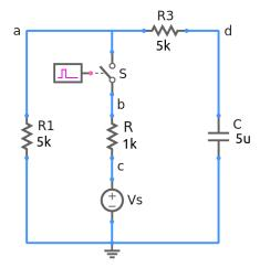
In the RC circuit shown in the figure, the switch has been closed for a long time and is opened at t=0.
