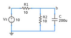
In the *RC* circuit shown in the figure, the initial capacitor voltage (at t = 0) is 0 V. Exercise Set
