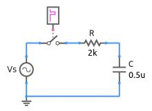
In the *RC* circuit shown in the figure, the switch has been open for a long time and is closed at t = 0. The initial capacitor voltage  $V_C(0^-)$  is 0 V. The source voltage is given by  $V_s = V_m \sin \omega t$ , with  $V_m = 1$  V and a frequency of 1 kHz. We are interested in the solution of the circuit equations for t > 0.
