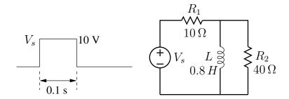
Shown in the figure is an RL circuit driven by a voltage pulse. Assume that the initial inductor current is zero.
