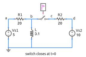
In the RL circuit shown in the figure, the switch has been open for a long time and is closed at t=0.
