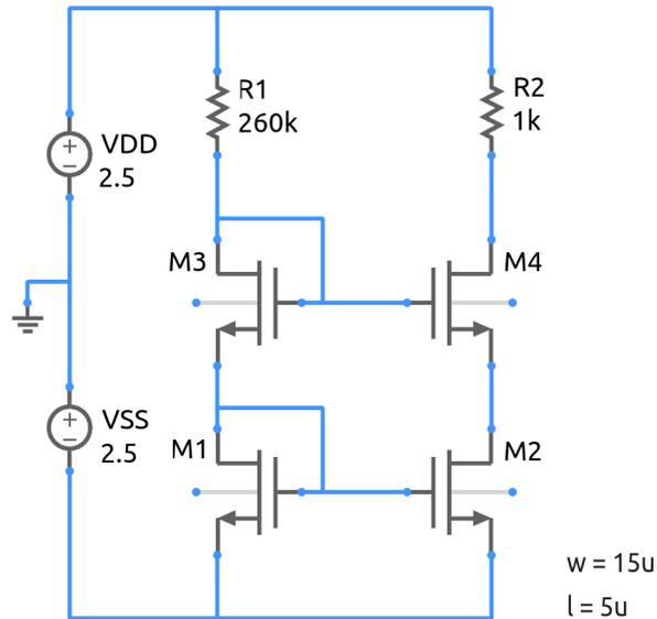
A cascode current source, which gives a significantly larger output resistance than the simple current source of `mos_mirror_1.sqproj`, is shown in the figure. It has been designed for an output current of  $10\mu\text{A}$ , with transistors  $M_1$ ,  $M_2$ ,  $M_3$ ,  $M_4$  having the same  $W/L$  ratios and other parameters.
