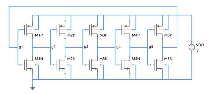
A ring oscillator with five CMOS inverters is shown in the figure. The oscillation frequency is given by
