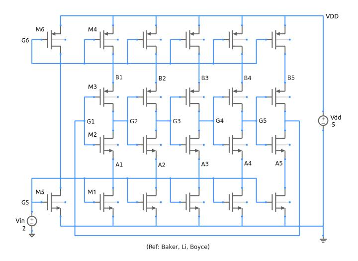
A voltage-controlled oscillator (VCO) with a five-stage ring oscillator is shown in the figure. Transistor pairs such as  $M_2$ - $M_3$  make up the inverters. In addition, we have transistors (e.g.,  $M_1, M_4$ ) which control the current available during switching.
