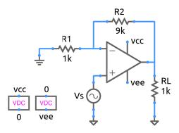
Shown in the figure is an Op Amp based non-inverting amplifier. In this circuit, the Op Amp operates in the linear regime, which guarantees that the inverting and non-inverting terminals of the Op Amp are approximately at the same potential, i.e.,
