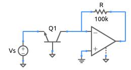
In a BJT operating in the active mode, the collector current  $I_C$  is an exponential function of the base-emitter voltage  $V_{BE}$ , given by
