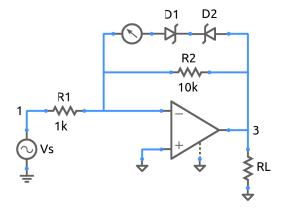
Shown in the figure is an Op Amp amplifier with the feature of limiting the output voltage to  $\pm (V_Z + V_D)$ , where  $V_Z$  is the Zener voltage and  $V_D$  is the forward turn-on voltage of the Zener diodes.
