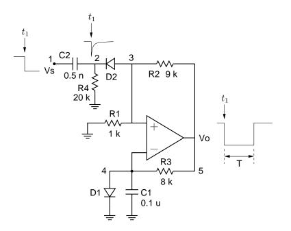
The purpose of a monostable circuit is to produce an output pulse when a transition is applied at the input. In the above circuit, a negative-going (i.e., high to low) transition works as a trigger, producing a negative pulse at the output, as shown in the figure. The operation of the circuit can be understood as follows [1]:
