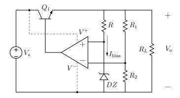
The purpose of a voltage regulator is to provide a constant DC voltage to the load in spite of variations in the input DC voltage or in the load. In the circuit shown in the figure, the "control element"  $(Q_1)$  is in series with the load  $R_L$ , and this configuration is therefore called a "series mode regulator." The Zener diode provides a reference voltage. The resistor R is selected in order to bias the Zener diode:
