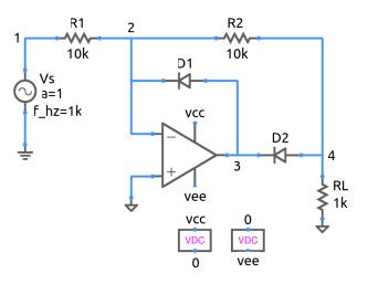
A precision half wave rectifier circuit is shown in the figure. In this circuit, the feedback loop is closed either with  $D_1$  conducting or  $D_2$  conducting, and the Op Amp operates in the linear regime (which is a desirable feature since the Op Amp does not need to come out of saturation when the input voltage changes sign). The inverting terminal of the Op Amp is therefore at virtual ground.
