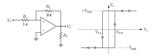
The Schmitt trigger circuit shown in the figure works on the basis of positive feedback, which makes the gain very high. As a result of the high gain, the Op Amp operates in the saturation region, i.e.,  $V_o = \pm V_{\text{sat}}$ . Let us consider these two cases:
