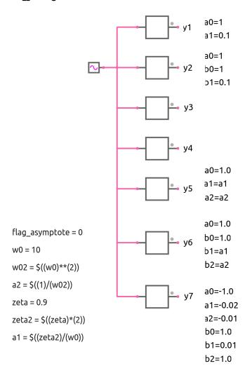
Shown in the figure are several filters with a common input signal.
