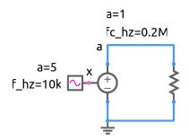
The purpose of the simulation set-up shown in the figure is to demonstrate frequency modulation. x(t) is the modulating signal, and  $V_a(t)$  is the output of the FM source.
