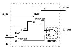
Architecture better of FullAdder is Component HalfAdder is port(a, b: in bit; s, cybar: out bit); End Component HalfAdder: signal s1, c1b, c2b: bit; begin HA1: Component HalfAdder portmap(a,b,s1,c1b); HA2: Component HalfAdder portmap(s1,c1b,sum,c2b); Cmbn: Component NAND2in portmap(c1b, c2b, C\_out); end Architecture better:
