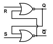
Entity RS\_Latch is Port(R,S: IN BIT; Q, Qbar: OUT BIT); End Entity RS\_Latch; Architecture trouble of RS\_Latch is Begin  $Q \leq R$  NOR Qbar;
