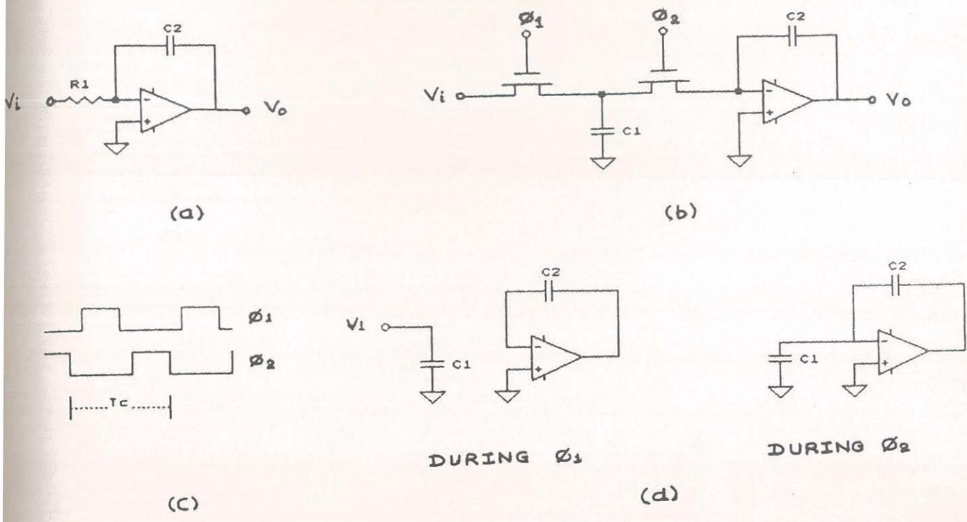
Fig. 3.3. Basic principle of the switched capacitor filter technique for an inverting integrator : (a) active-RC integrator, (b) switched capacitor integrator, (c) two-phase clock (nonoverlapping), (d) during  $\phi_1$ ,  $C_1$  charges up to the current value of  $V_i$  and then, during  $\phi_2$ , discharges into  $C_2$ .
