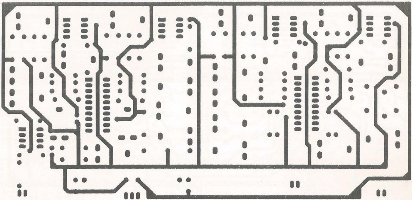
2. Component side layout of filter PCB.
