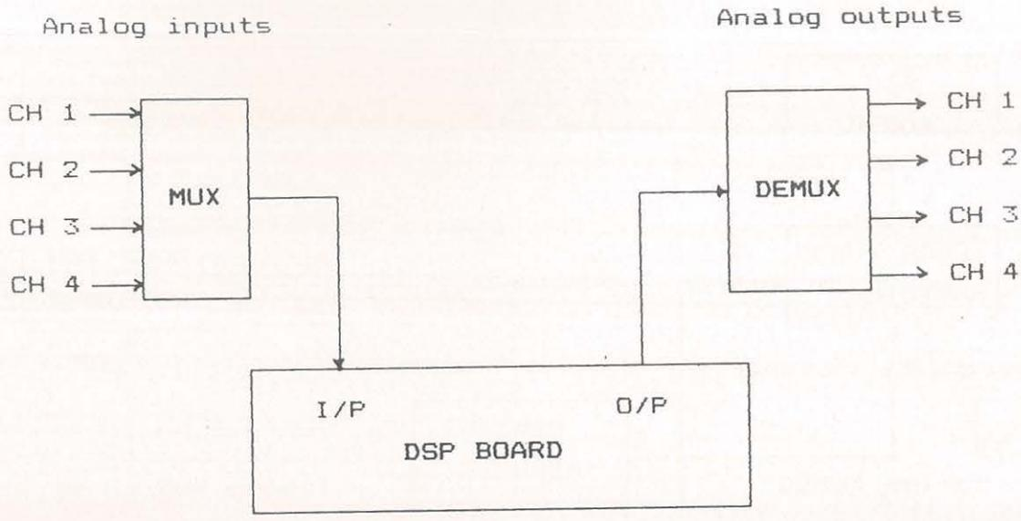
Fig. 4.1 Block diagram of I/O expansion with multiplexer and demultiplexer.
