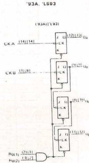
The J and K inputs shown without connection are for reference only and are functionally at a high level. Pin numbers shown in ( ) are for the 'LS93 and '93A and pin numbers shown in [ ] are for the 54LS93.
