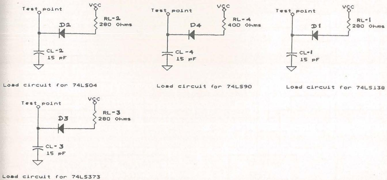
Fig. 4.5. Loading circuits for TTL ICs used on the I/O expansion unit.
