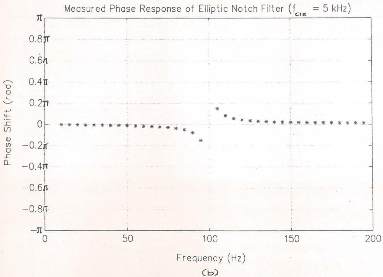
Fig. 3.12. Measured frequency response of second order elliptic notch filter. (a) magnitude response, (b) phase response.
