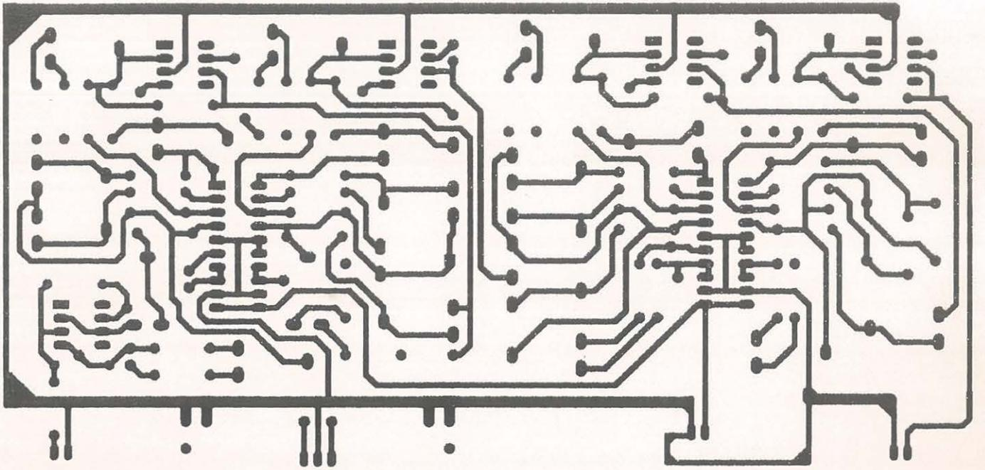
3. Solder side layout of filter PCB.
