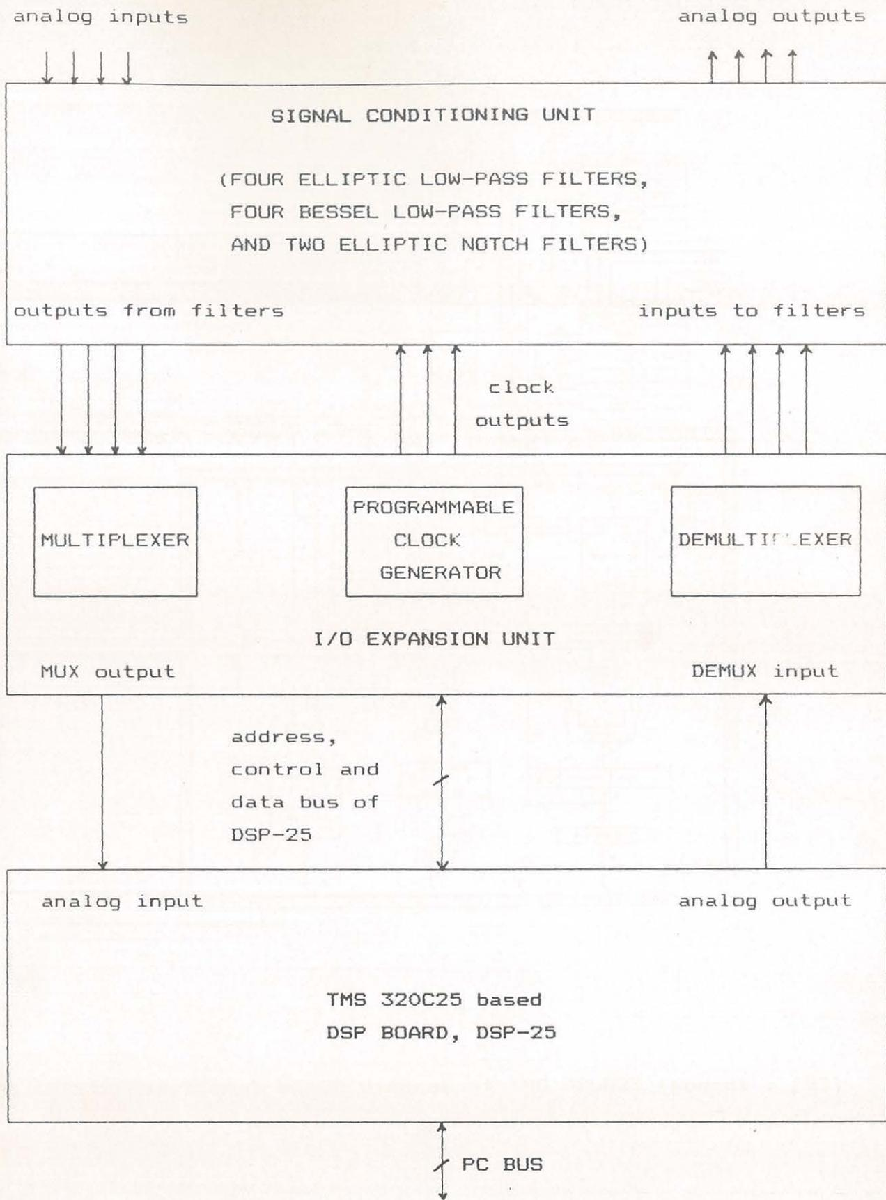
Fig. 2.1 Block diagram of data acquisition system.
