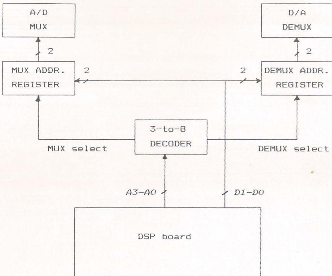
Fig. 4.2. Block diagram of the I/O expansion scheme.
