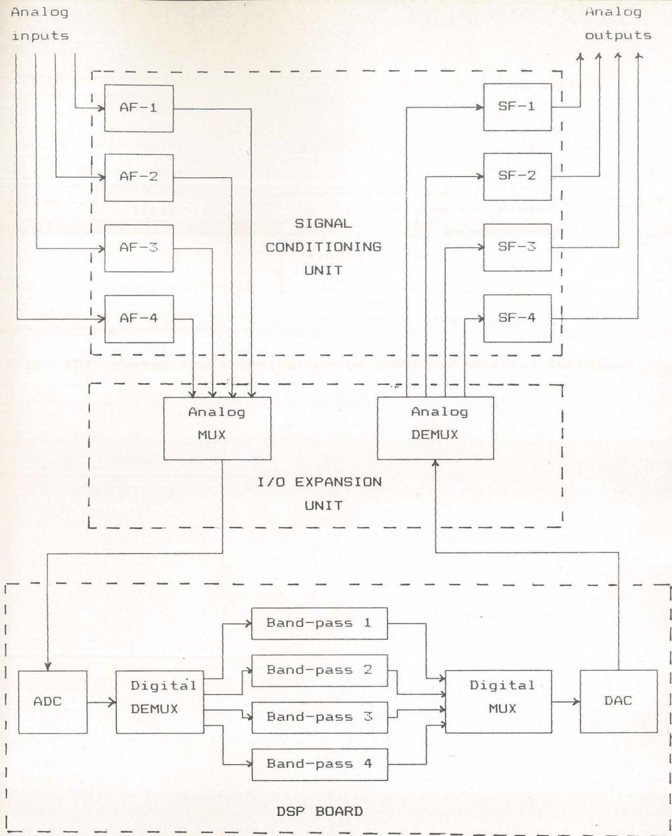
Fig. 5.1 Block diagram of band-pass filter for four channels.
