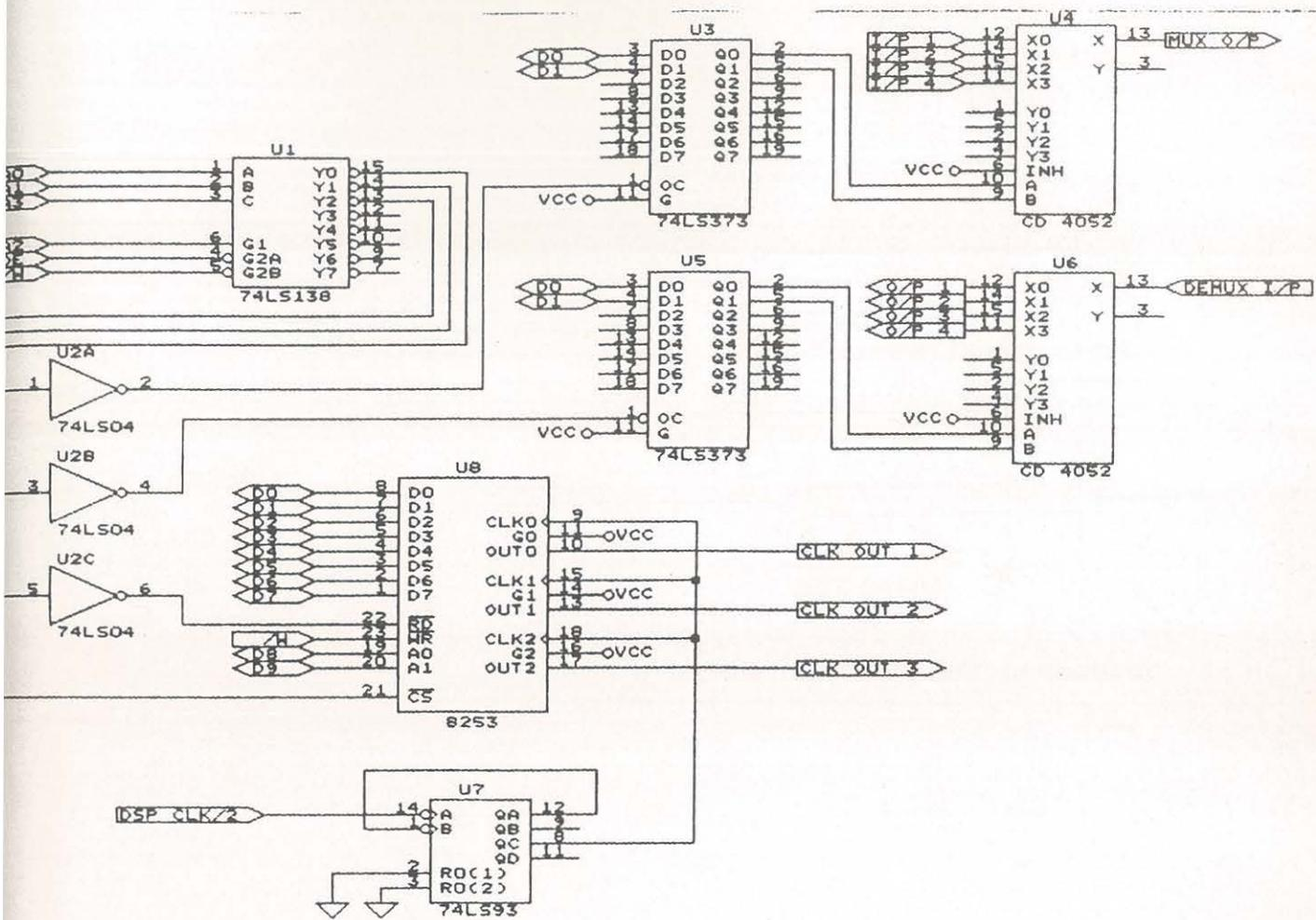
Fig. 4.3. Circuit schematic of the I/O expansion unit.
