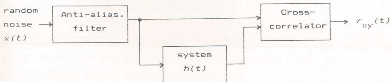
Fig. 5.2 System characterization by cross-correlation technique.
