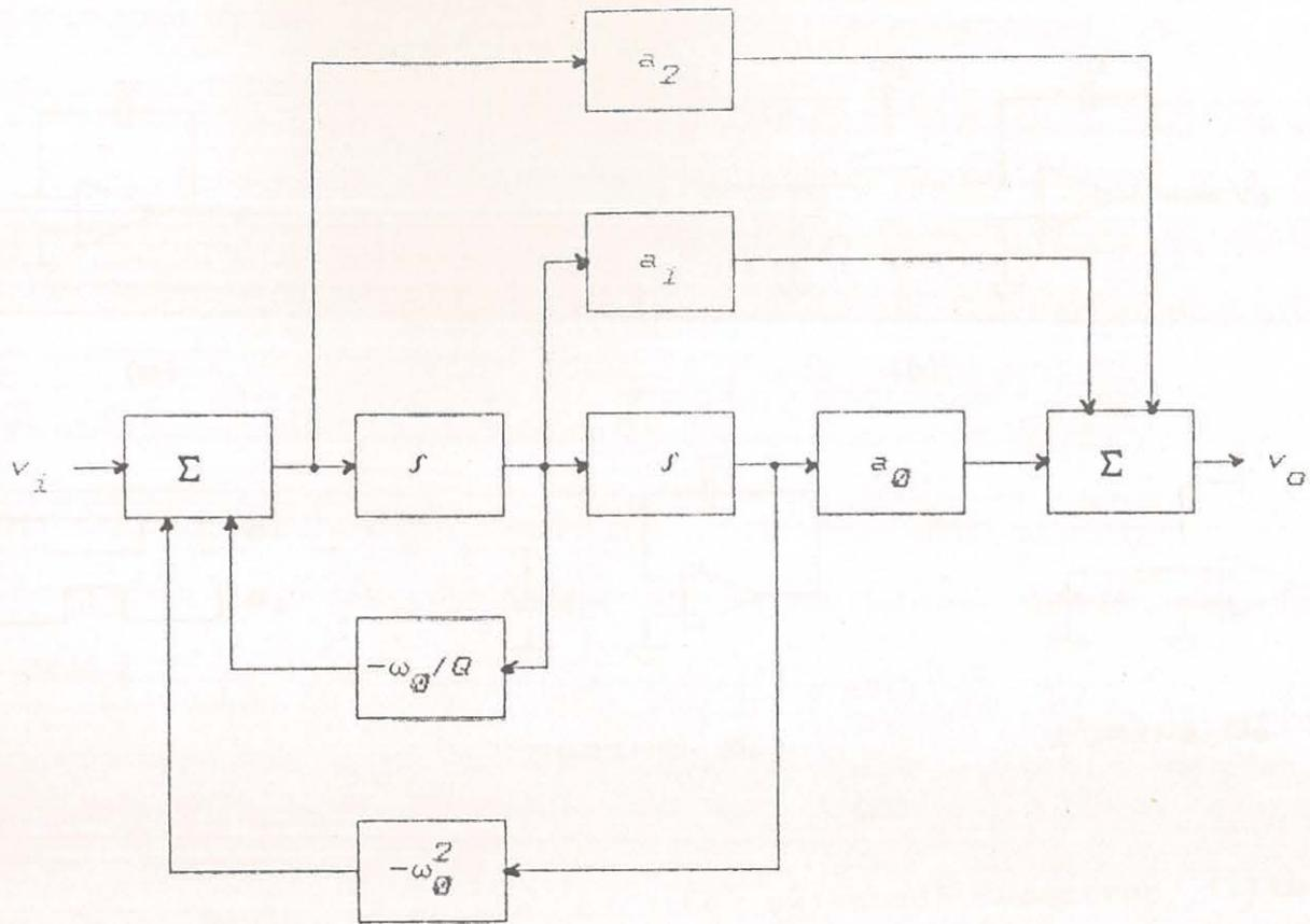
Fig. 3.2. Realization of a pole-zero biquad section using state variable feedback.
