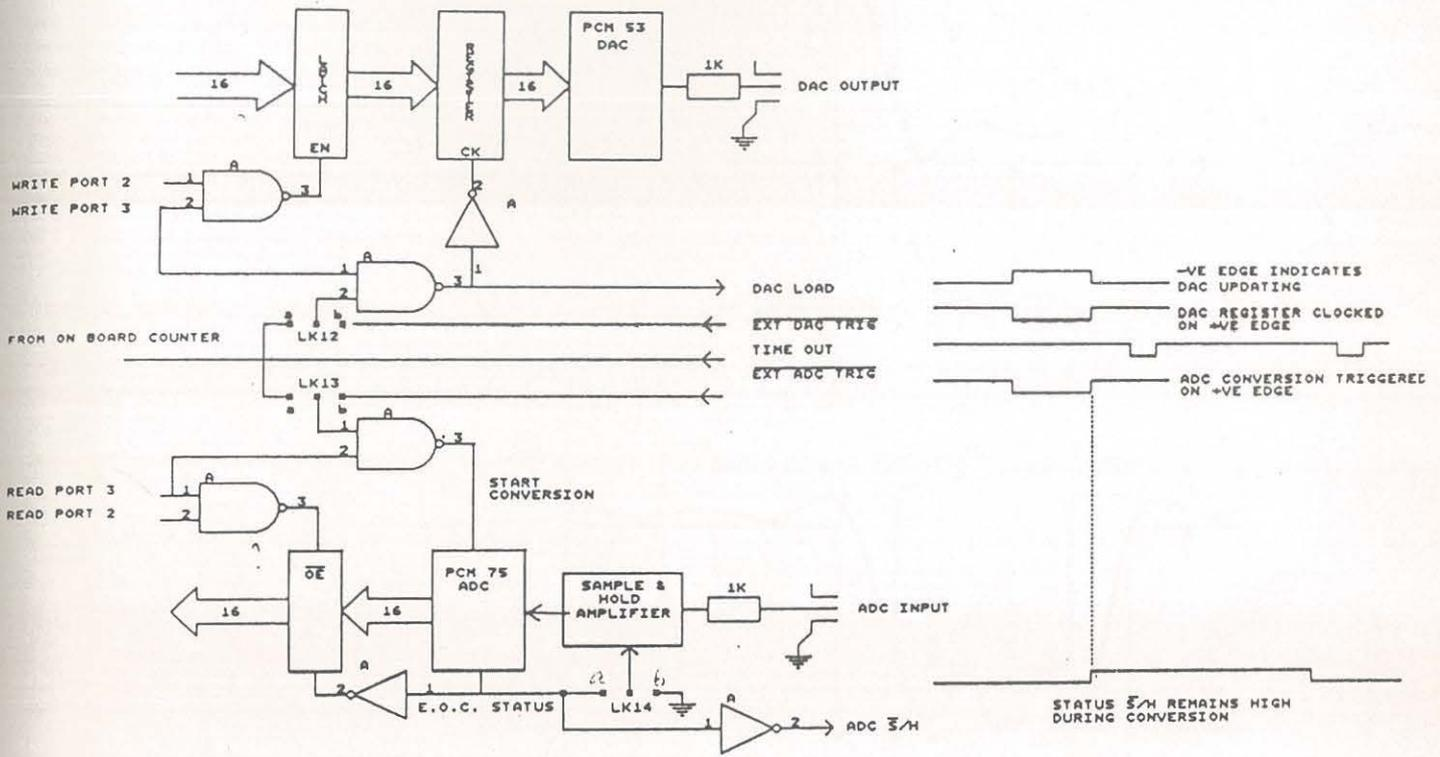
Fig. 2.4. Schematic of analog I/O interface on the DSP board PCL-DSP25 (source : [9]).
