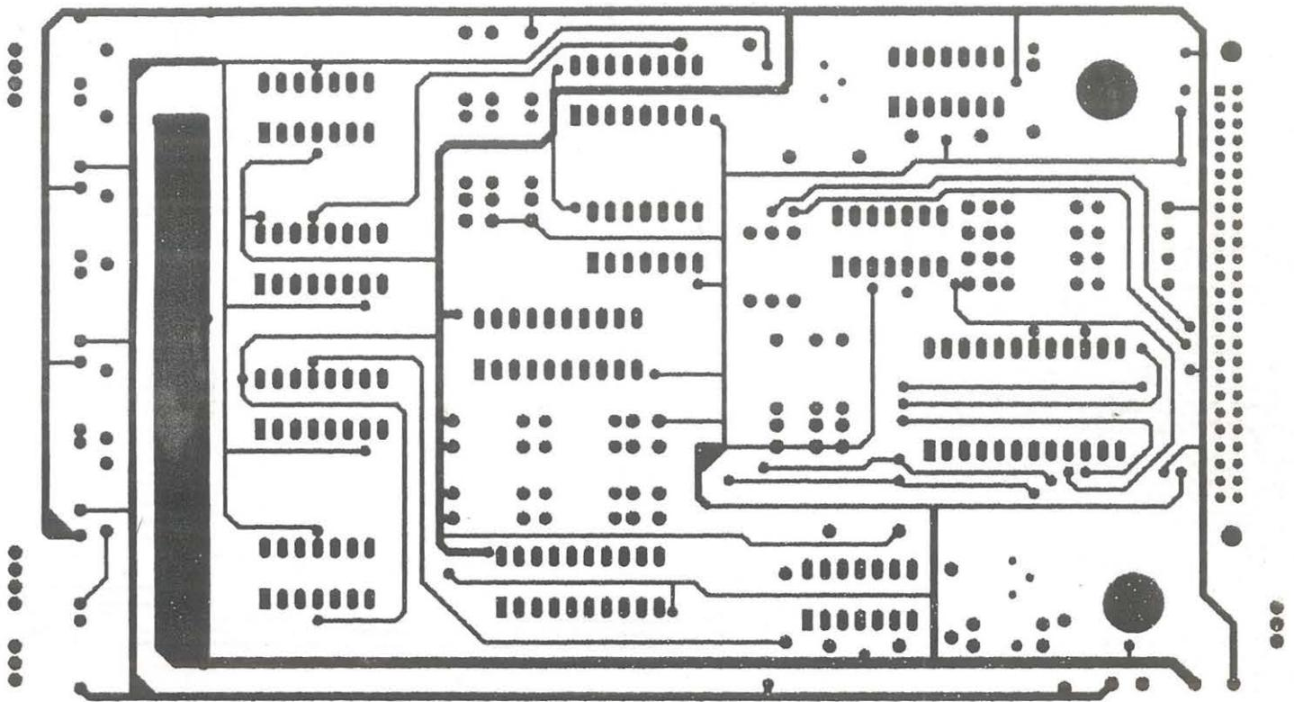
2. Component side layout of PCB of I/O expansion unit.
