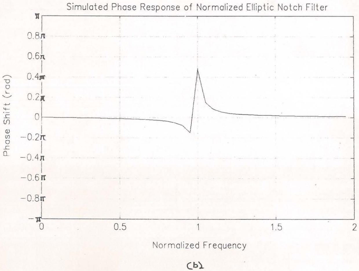
Fig. 2.8. Frequency response of second order elliptic notch filter : (a) magnitude response, (b) phase response.
