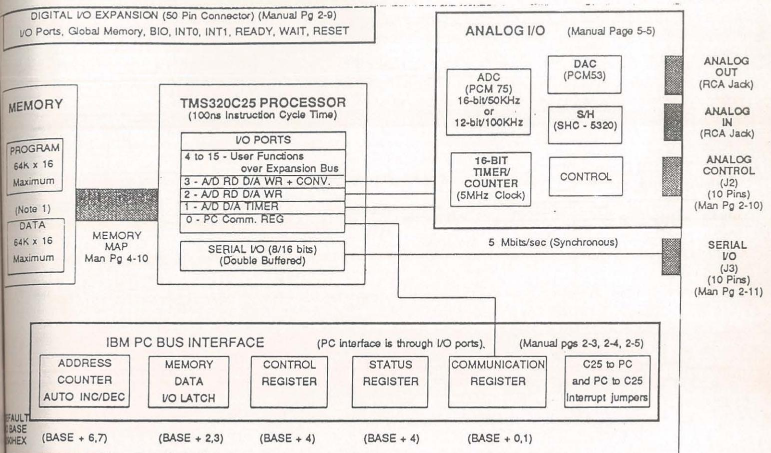
Fig. 2.3. Block diagram of the DSP board PCL-DSP25 (source : [9])
