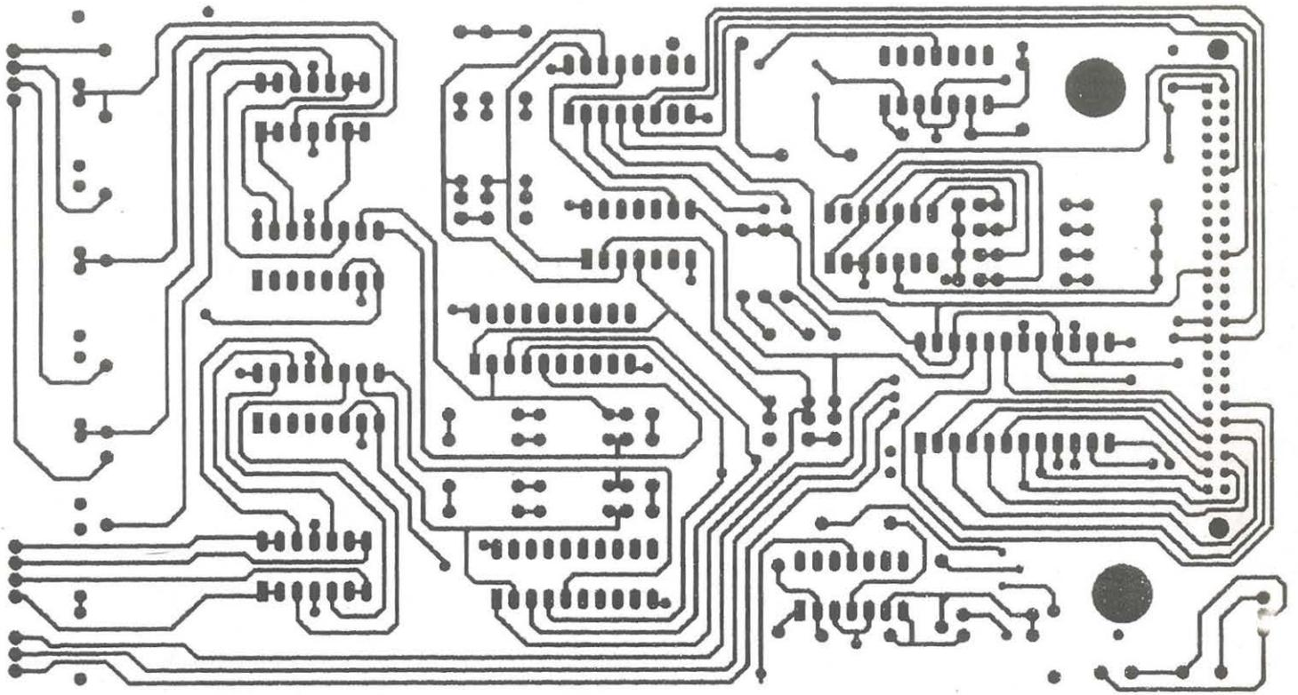
5. Solder side layout of PCB of I/O expansion unit.
