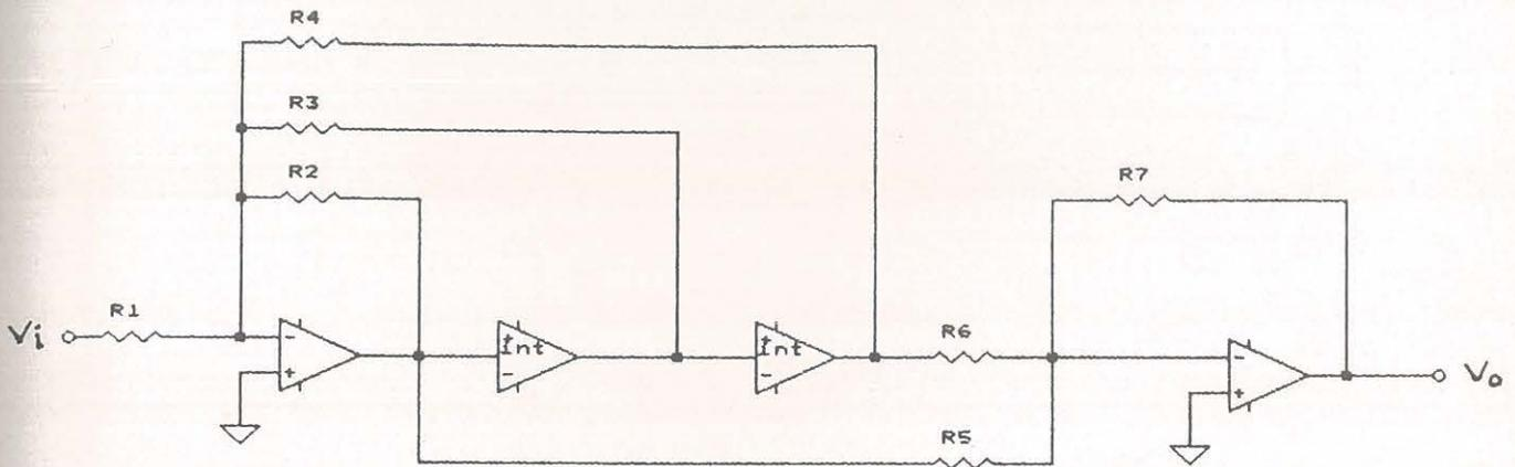
Fig. 3.6. Biquad realization using switched capacitor filter IC MF 10.
