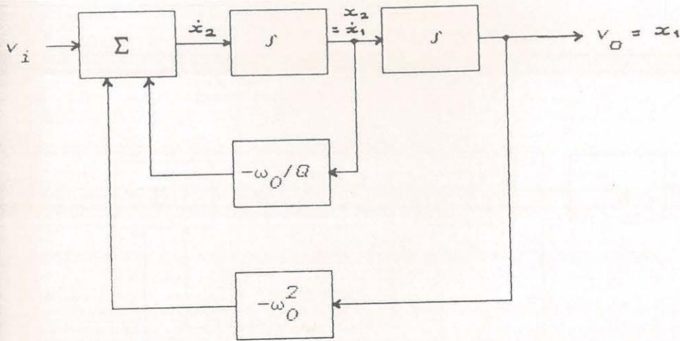
Fig. 3.1 Realization of an all-pole biquad section using state variable feedback.
