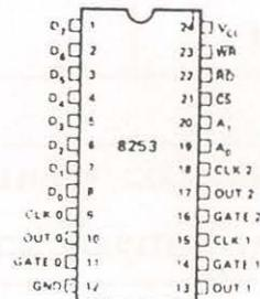
Figure 2. Pin Configuration
