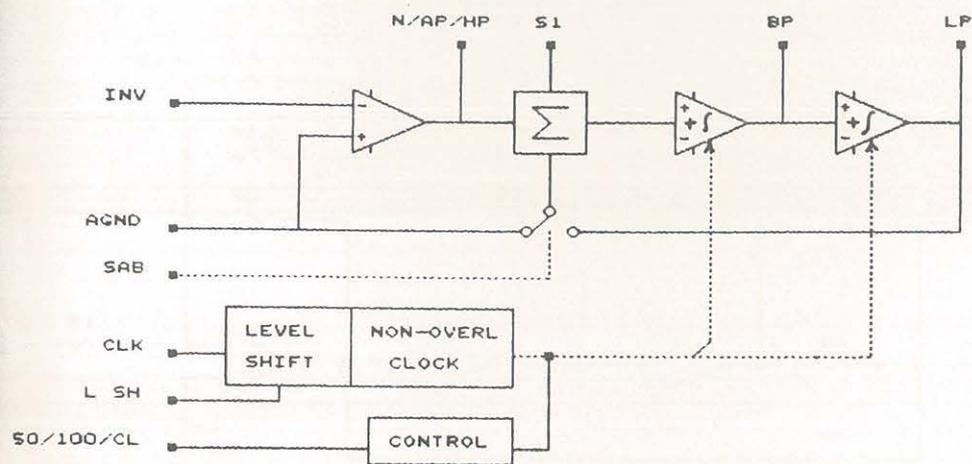
Fig. 3.5. Functional block diagram of the switched capacitor filter IC MF10 (source : [16]).
