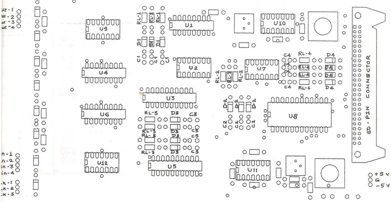
1. Component placement on PCB of I/O expansion unit.
