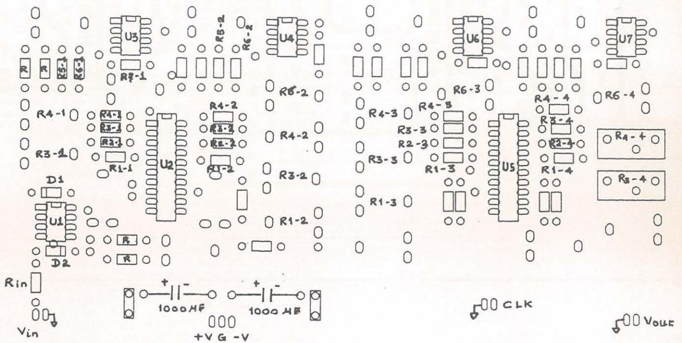
1. Component placement on the filter PCB.
