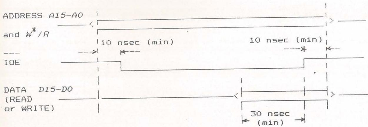
Fig 4.4. Timing diagram of OUT instruction for DSP processor TMS 320C25.
