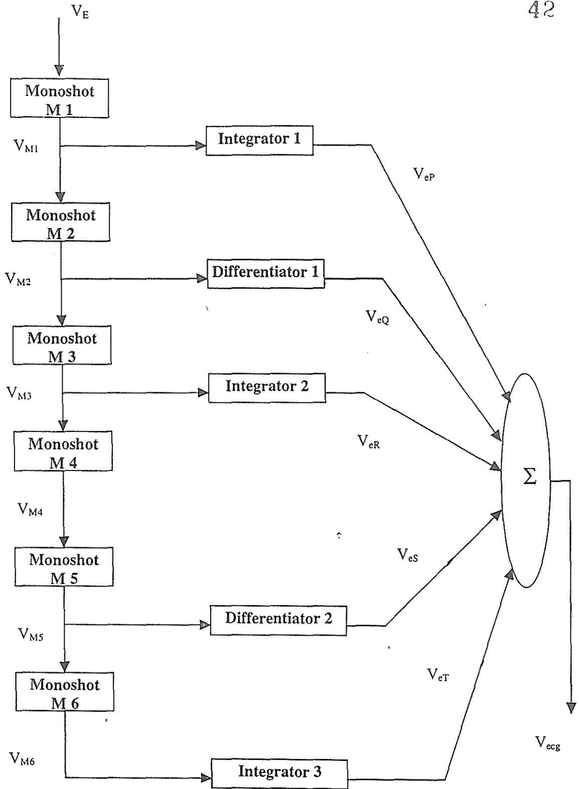
Fig. 4.4 Block diagram of ECG waveform Simulator
