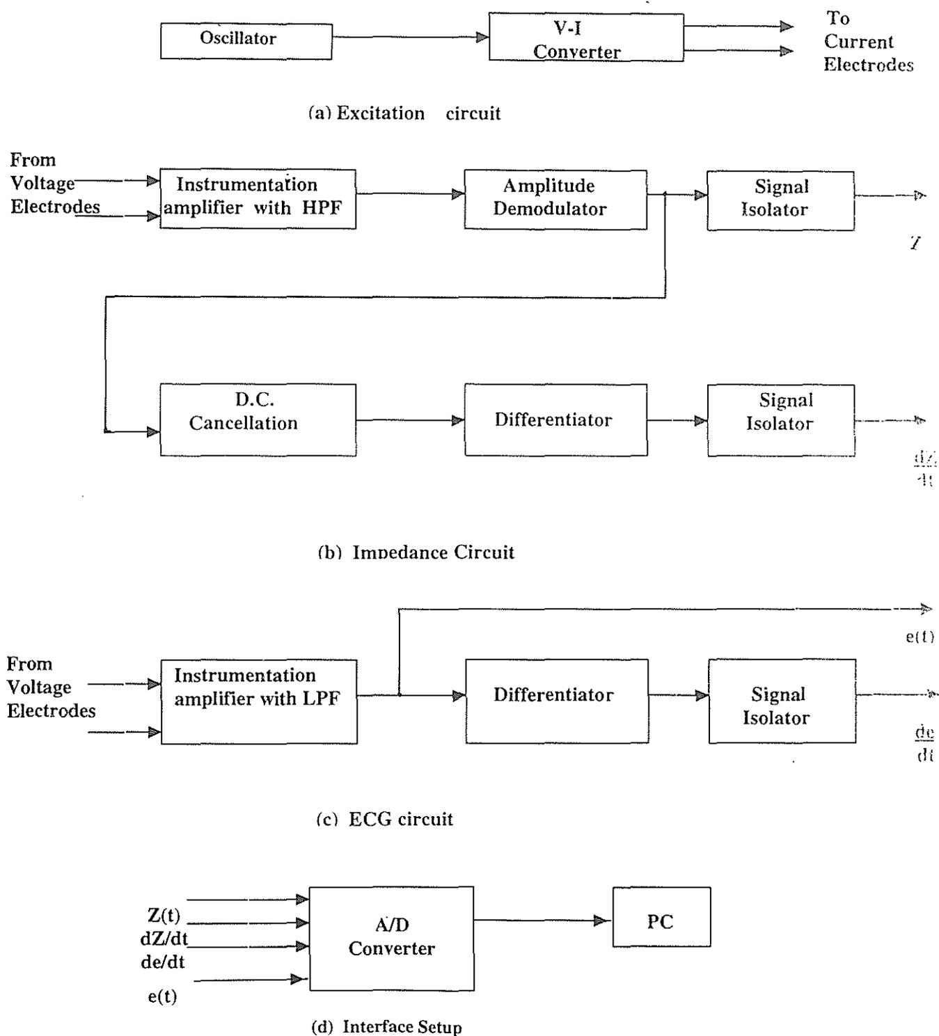
Fig. 3.1 Block diagram of impedance cardiograph developed by Joshi [2].
