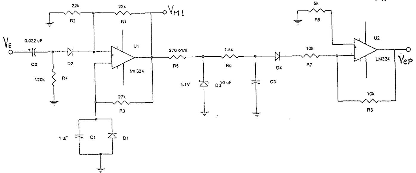
Fig. 4.7 Circuit diagram for generation of P wave
