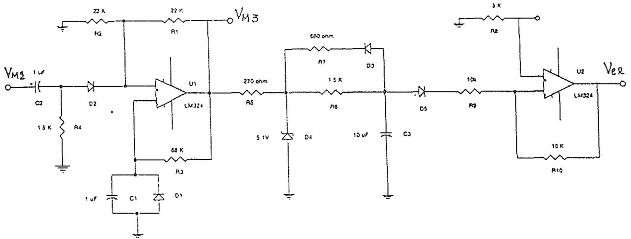
Fig. 4.9 Circuit diagram for generation of R wave
