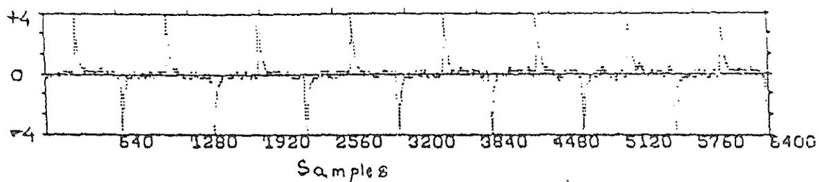
Fig. 4.15 Derivative of impedance,  $dz/dt$ , obtained from simulator
