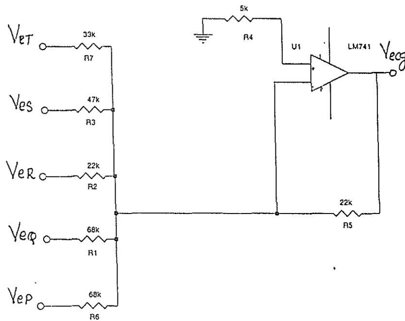
Fig. 4.12 Circuit diagram for generation of adder
