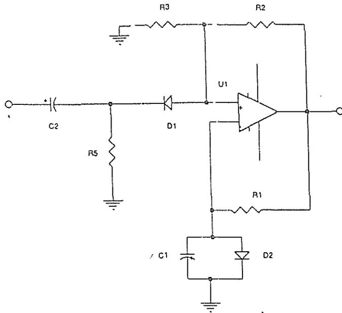
Fig. 4.5 Monostable multivibrator
