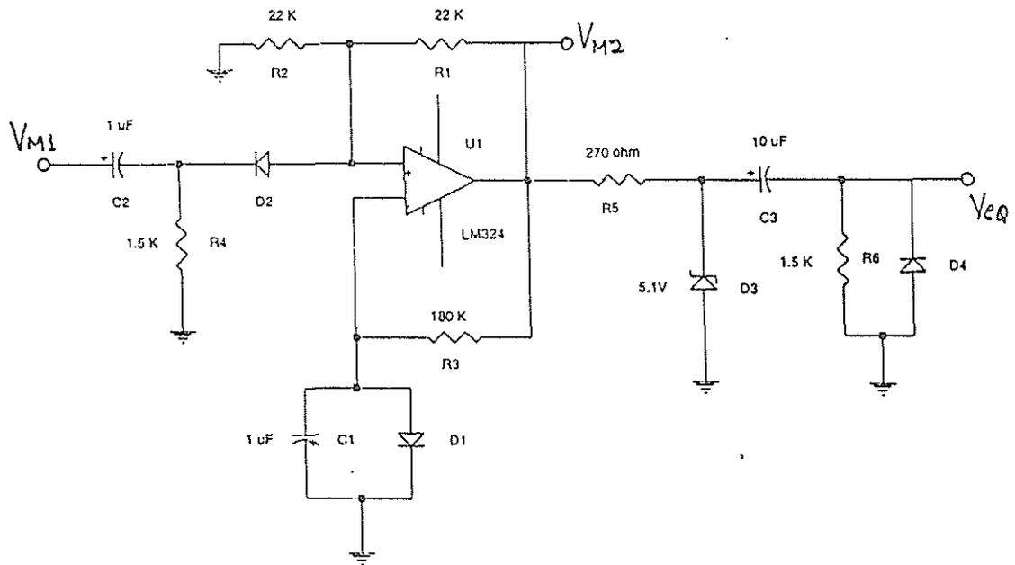
Fig. 4.8 Circuit diagram for generation of Q wave
