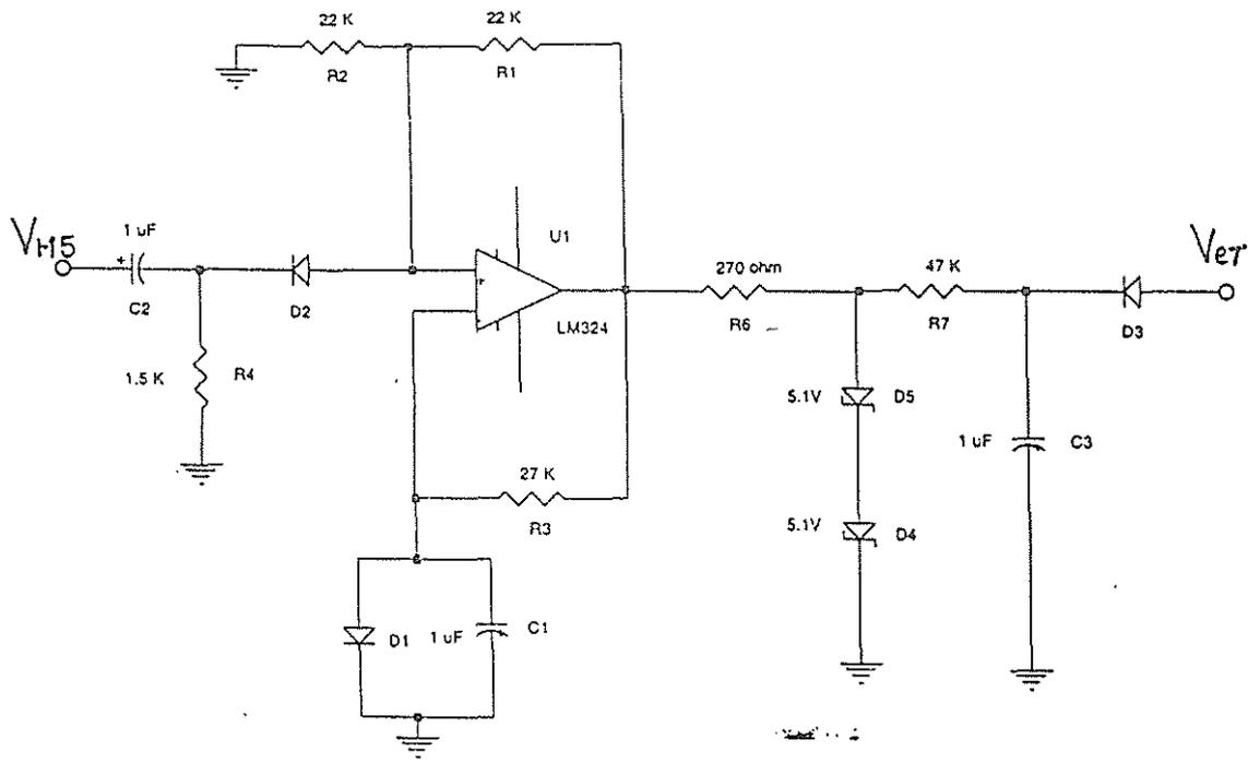
Fig. 4.11 Circuit diagram for generation of T wave
