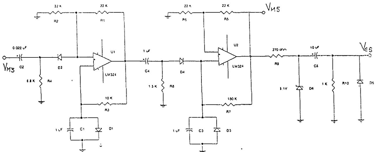
Fig. 4.10 Circuit diagram for generation of S wave
