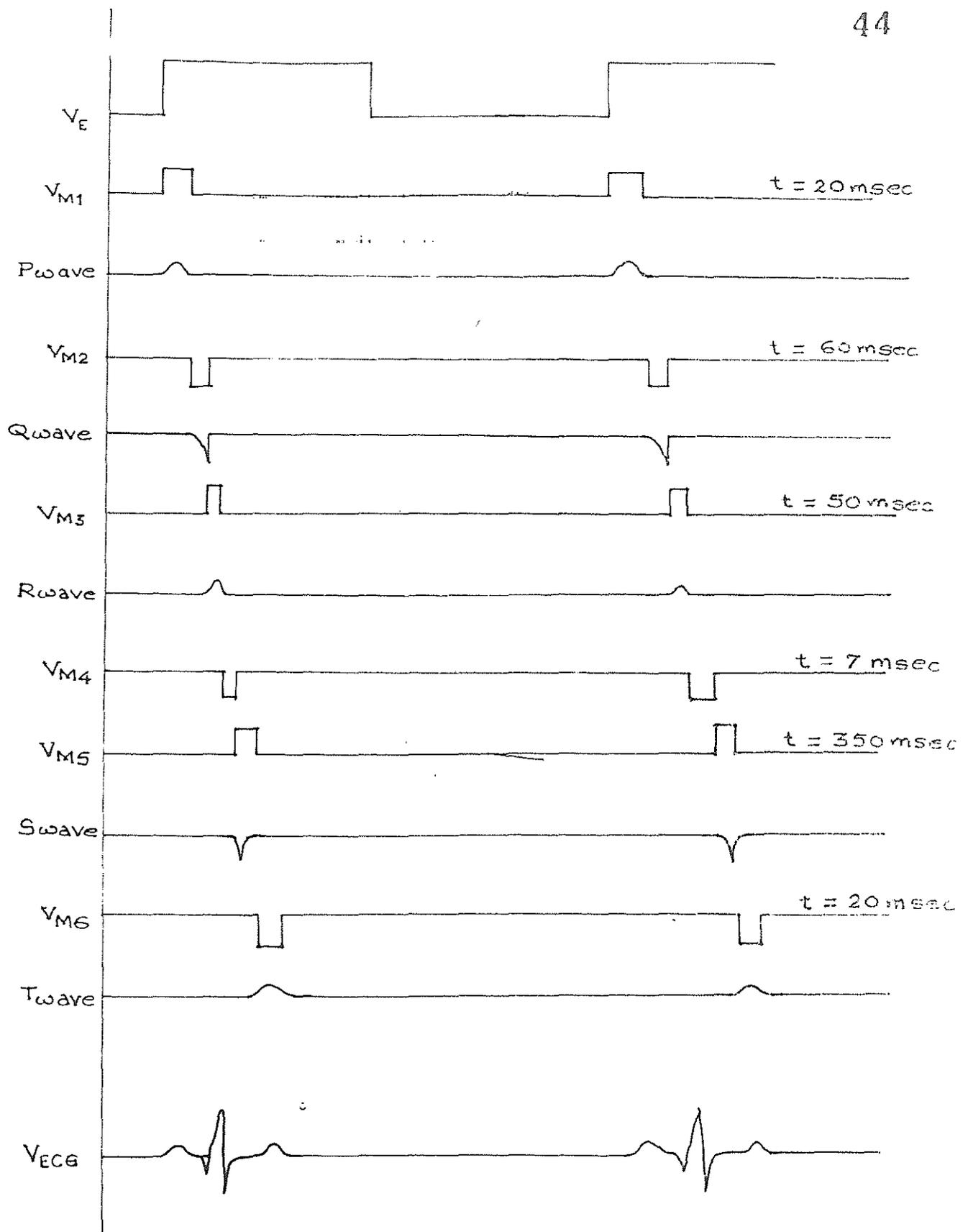
Fig. 4.6 Timing diagram for generation of ECG waveform
