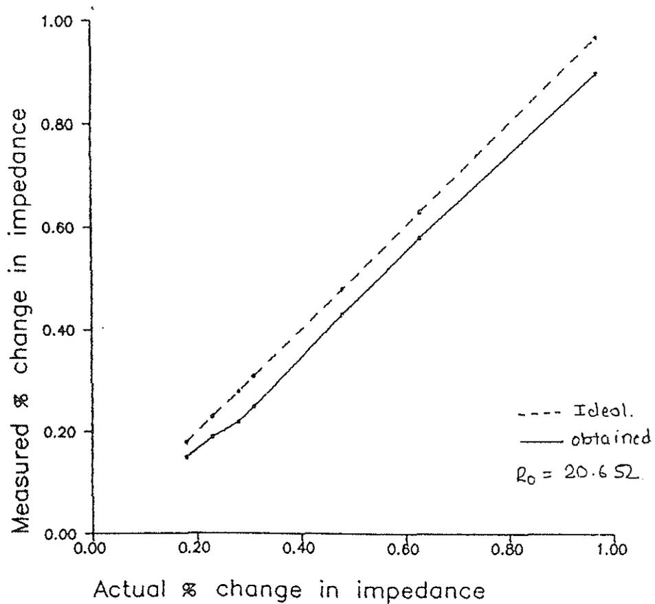
Fig. 6.1 Graph of actual % change in impedance v/s measured % change in impedance
