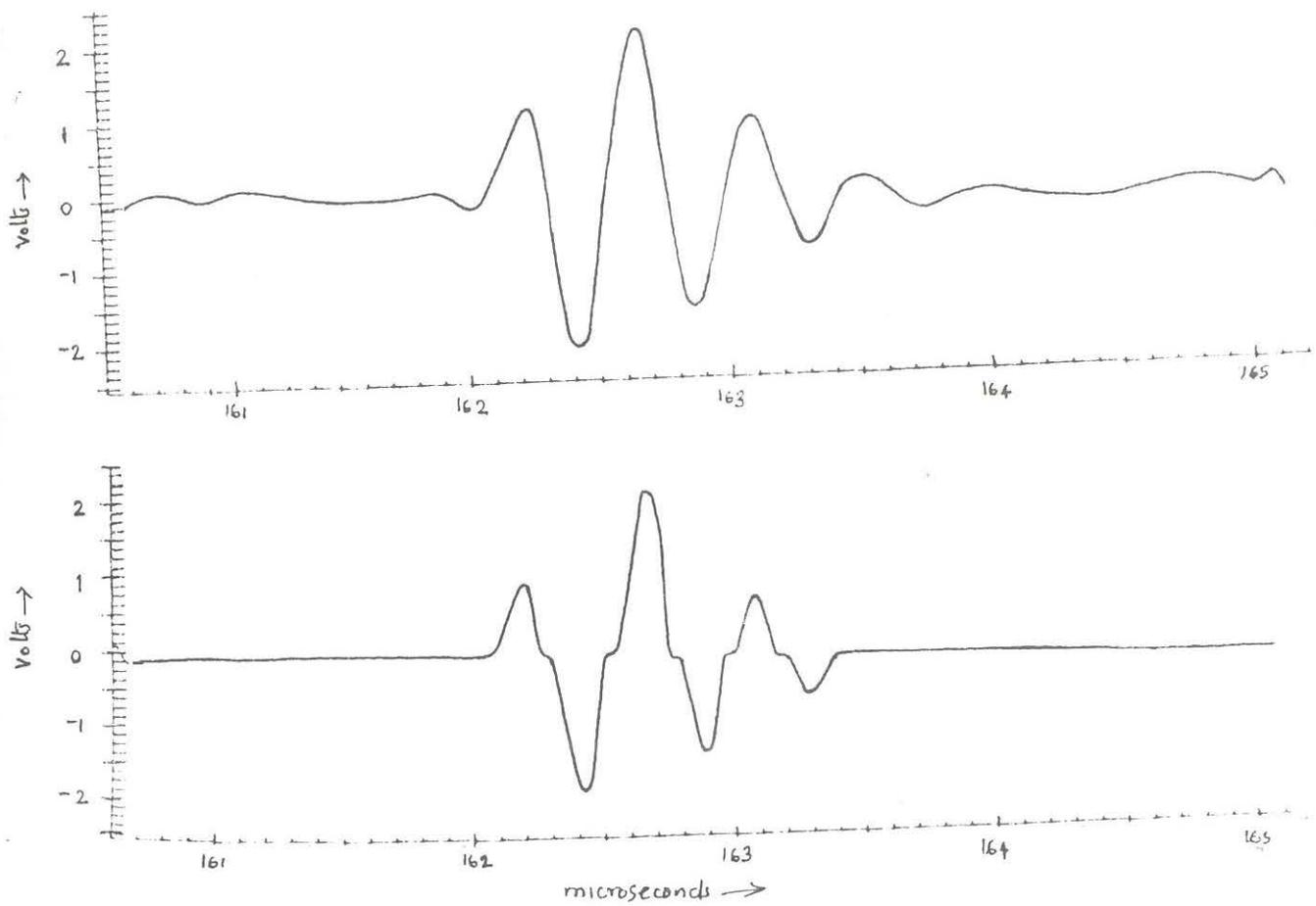
Fig. 4.4. Typical waveforms before and after the centre-clipping circuit.
