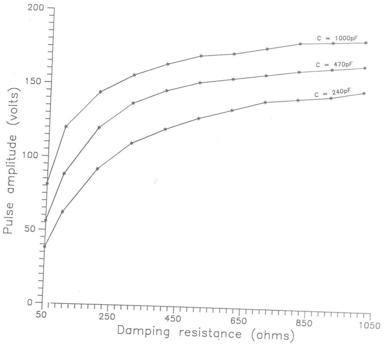
Fig. 4.9 Pulse amplitude vs damping resistance characteristics of the transmitter
