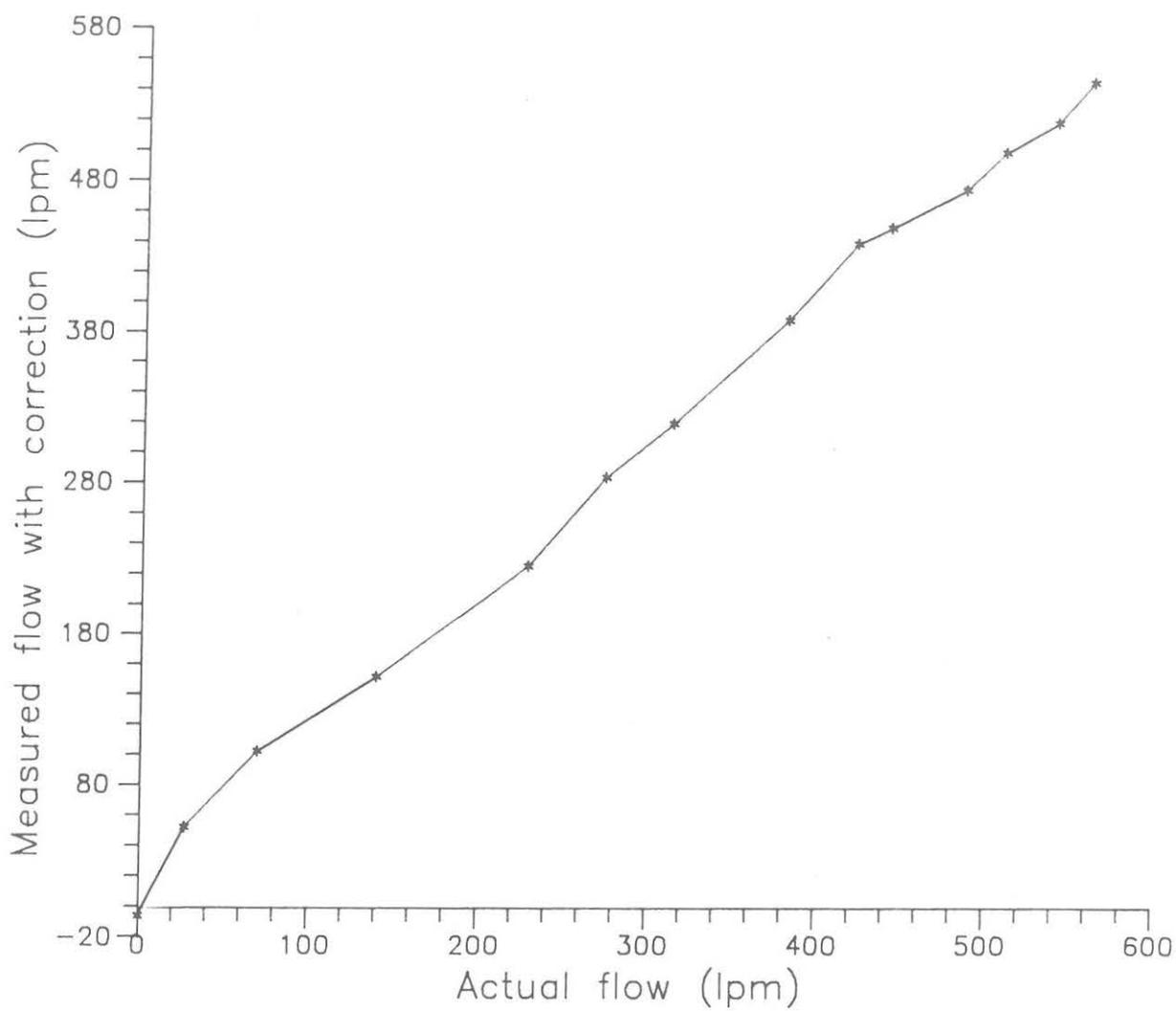
Fig. 5.7. Measured flow rate, with correction vs actual flow rate
