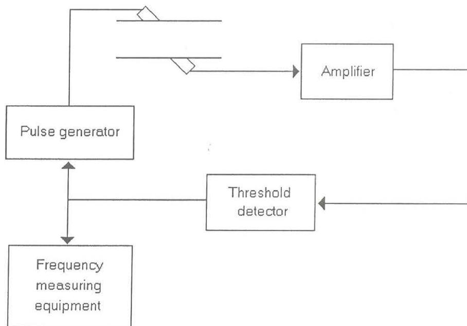
Fig. 2.4. Block diagram showing sing-around principle
