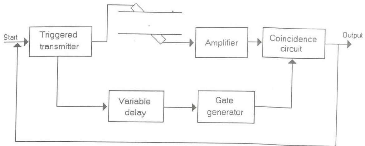
Fig. 2.5. Sing-around system developed by *Forgacs*
