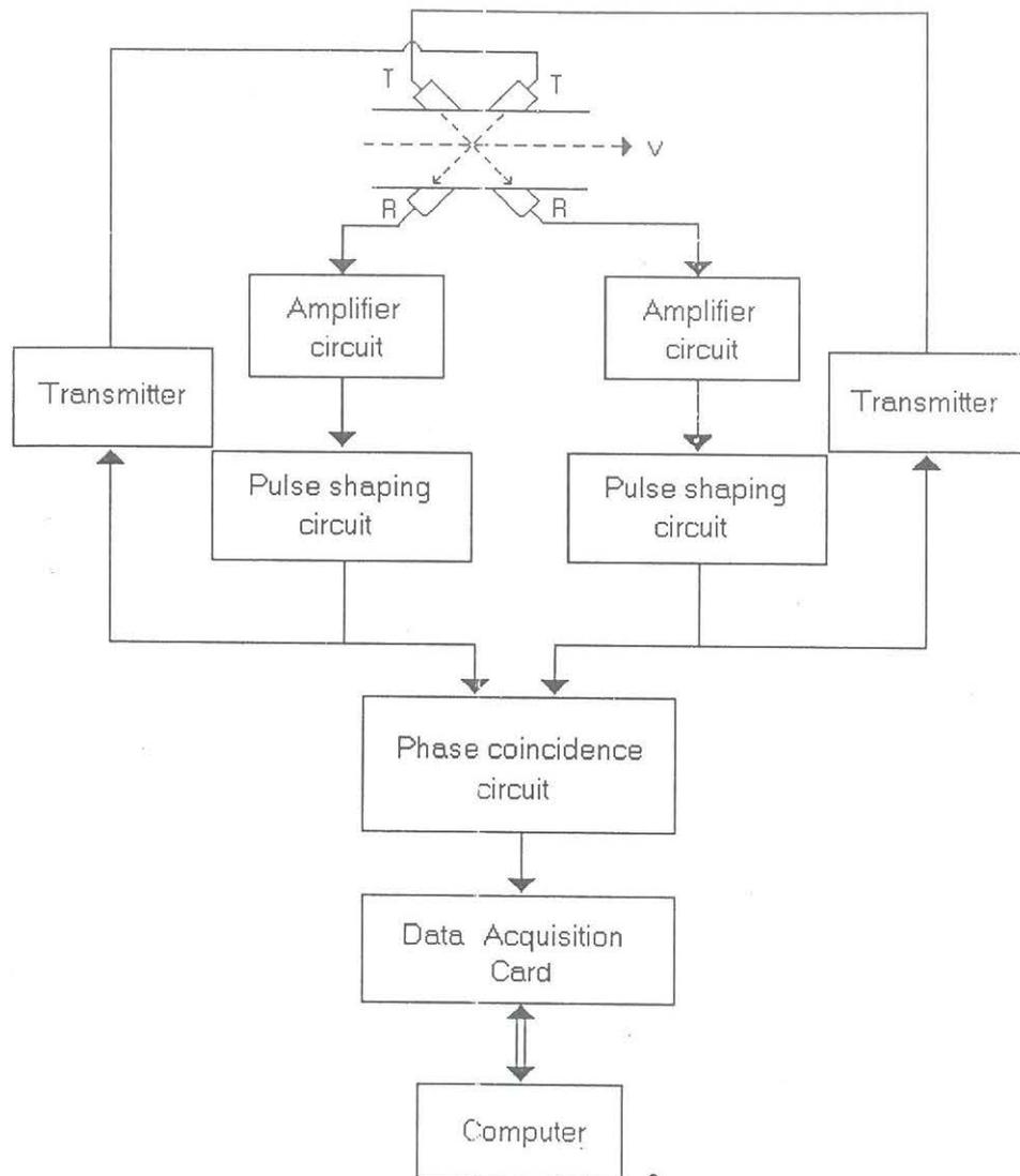
Fig. 3.1. Block diagram of SAF-1
