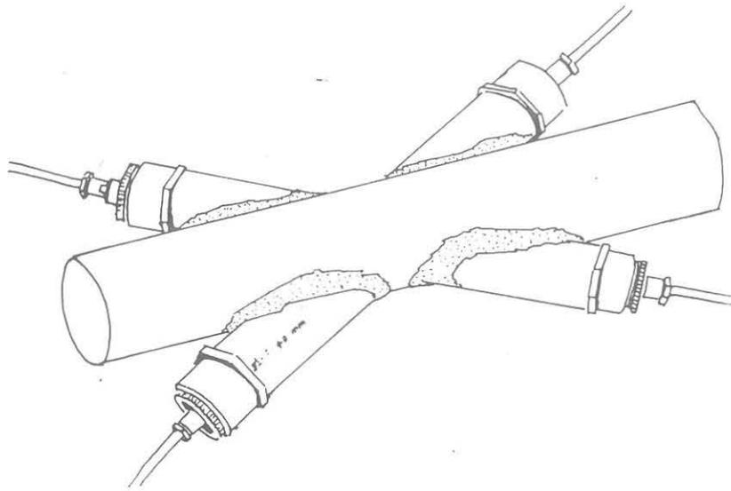
Fig. 5.1. Transducer assembly
