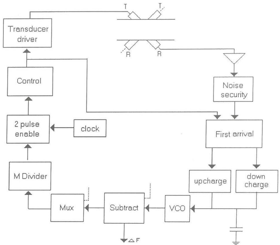
Fig. 2.7. Two pulse phase comparison method
