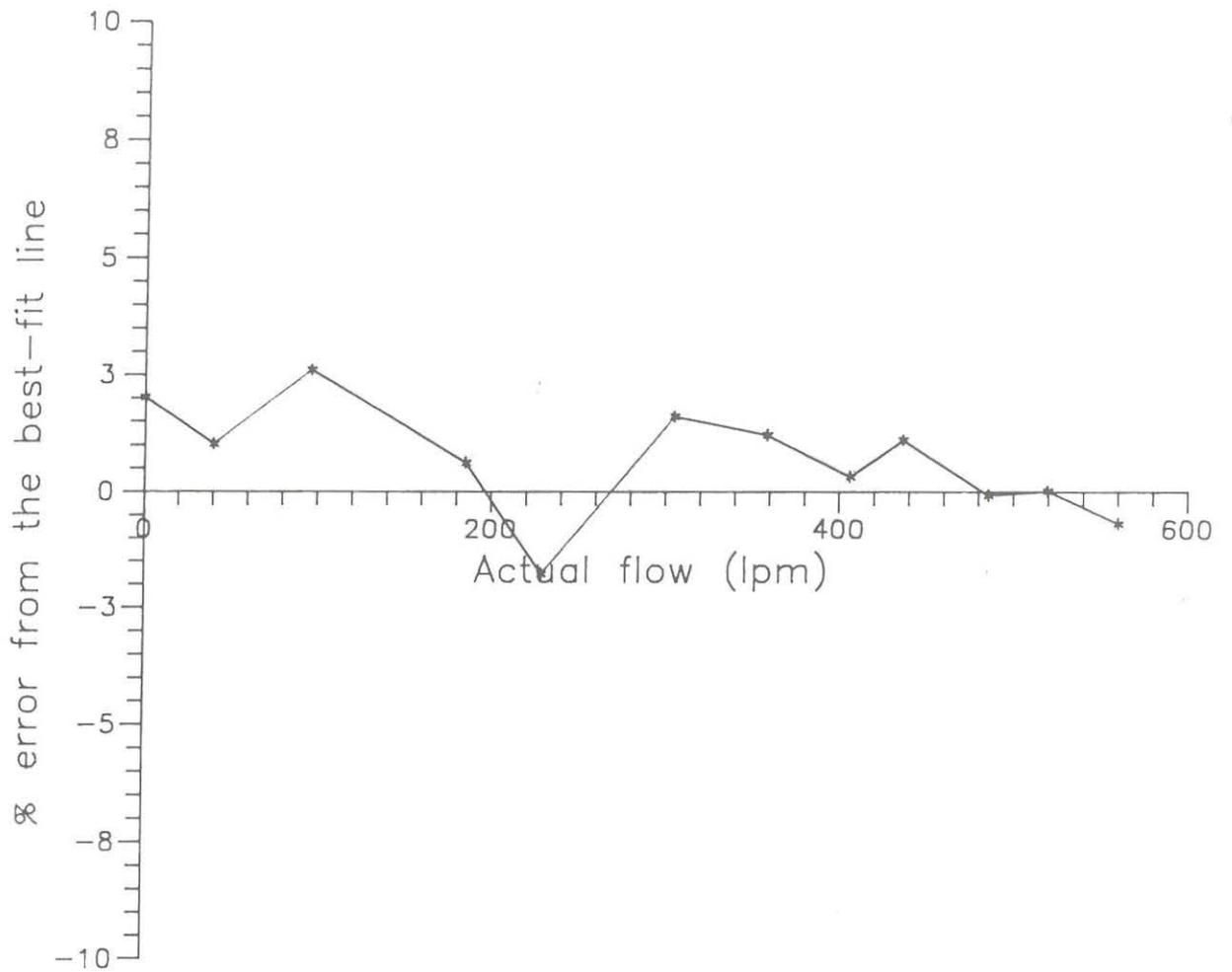
Fig. 5.6. Percentage error in the flow rate measured, from the best-fit line vs actual flow rate
