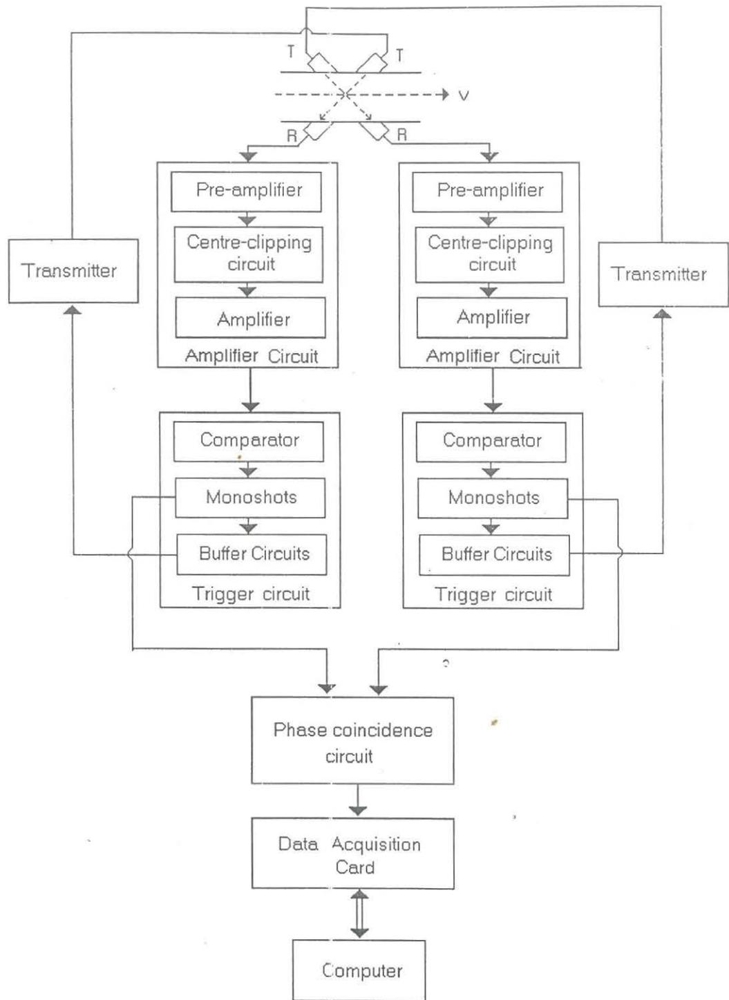
Fig. 4.1. Block diagram of SAF-2
