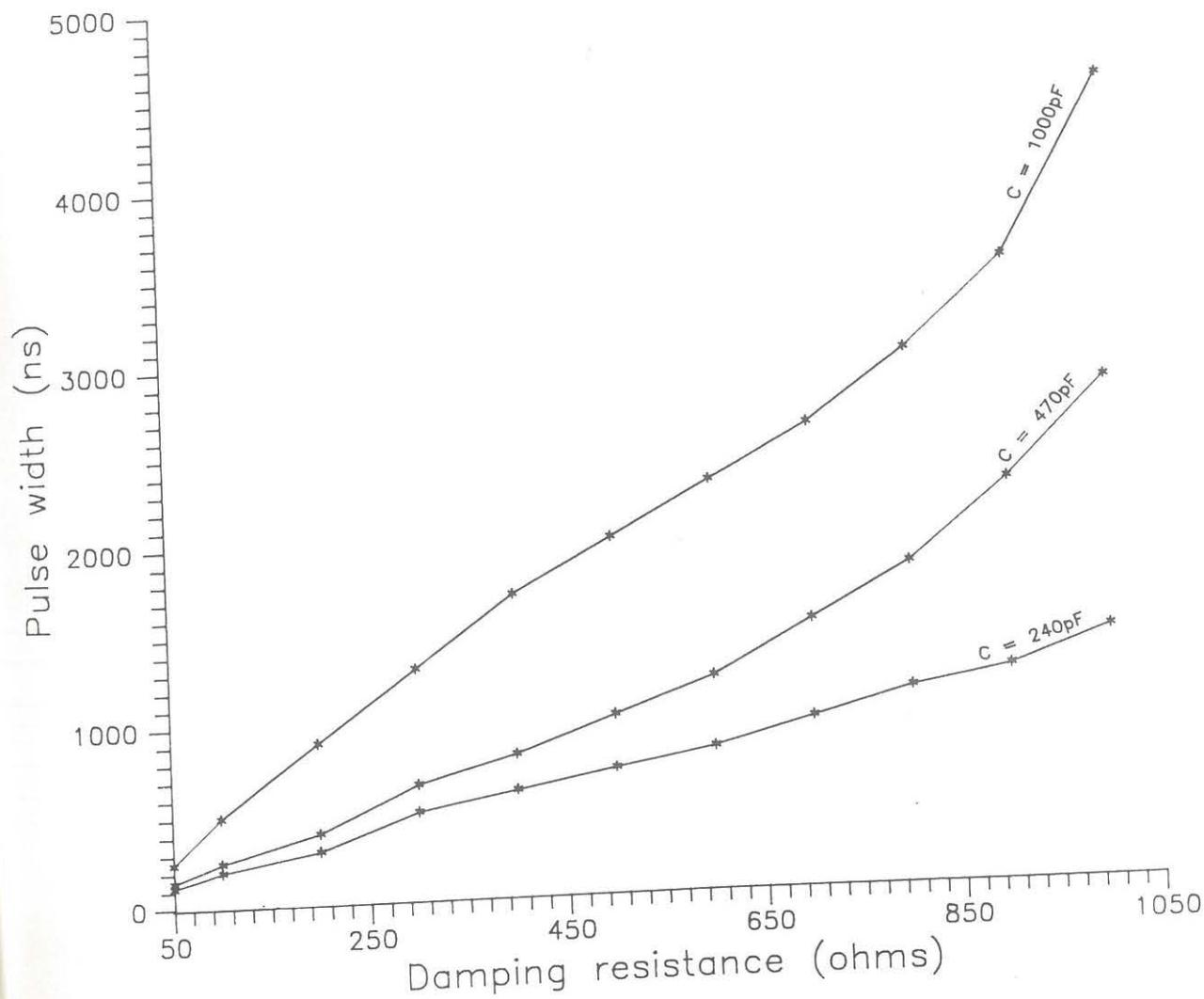
Fig. 4.8. Pulse width vs damping resistance characteristics of the transmitter
