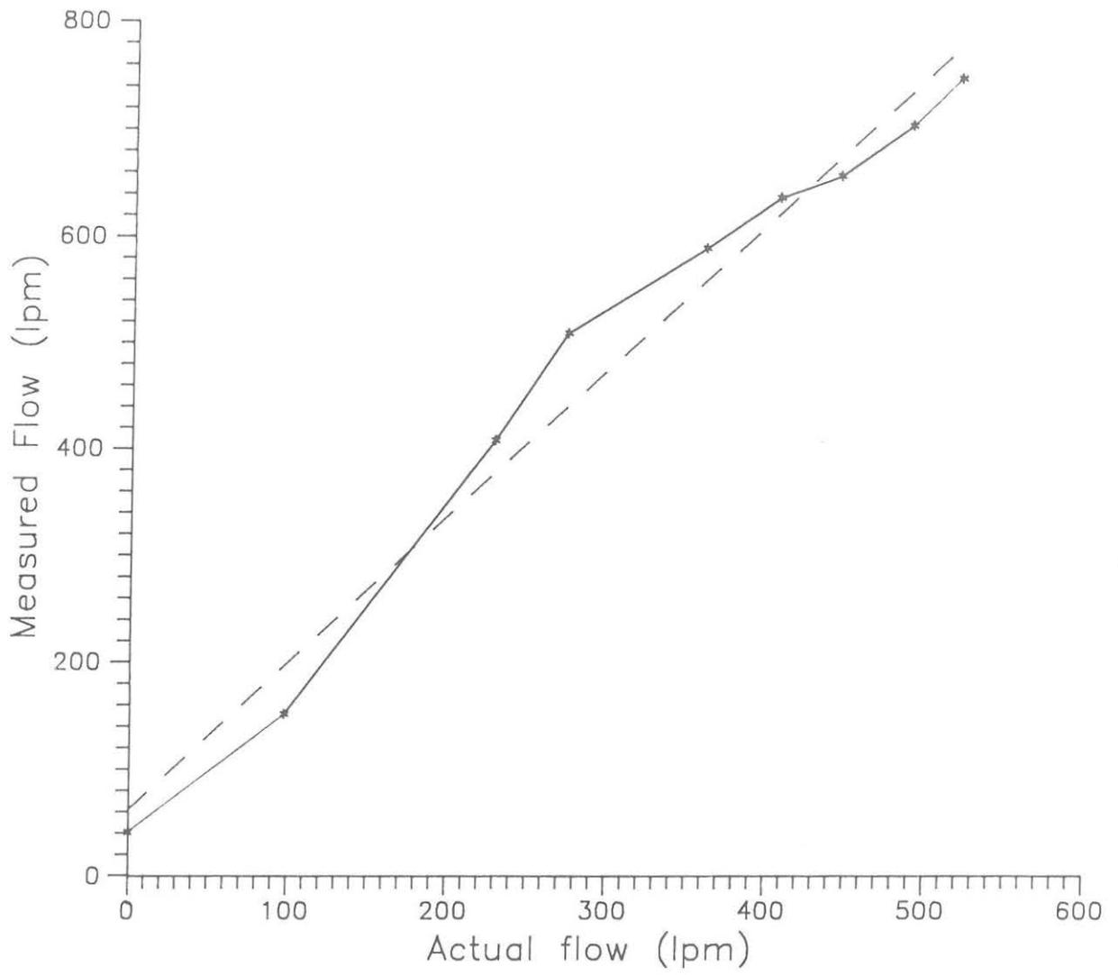
Fig. 5.3. Flow rate measured using single path transmission vs actual flow
