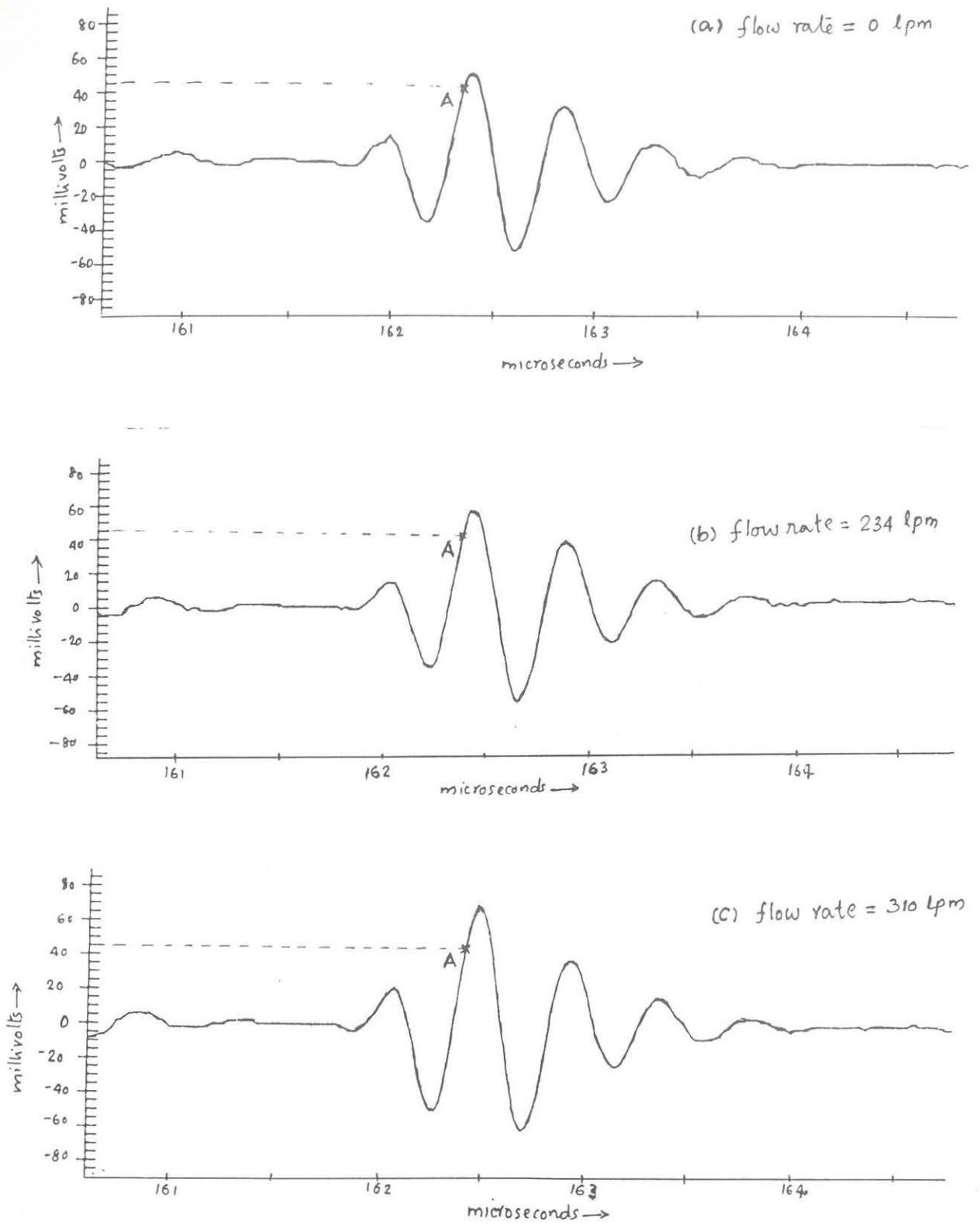
Fig. 3.2. Ultrasonic signal received at the transducer, at different flow rates
