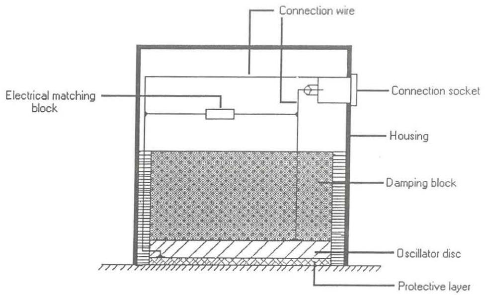
Fig. 4.10. Schematic of an ultrasonic transducer
