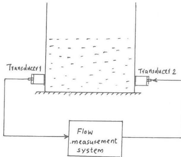
Fig. 5.2. Test bench for measurement of  $c$
