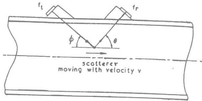
Fig. 2.1. Principle of doppler frequency shift flowmeter
