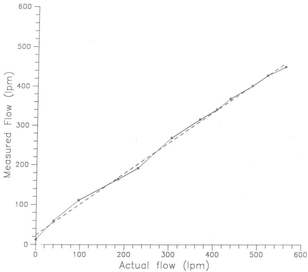
Fig. 5.5. Flow rate measured using dual path transmission vs actual flow rate
