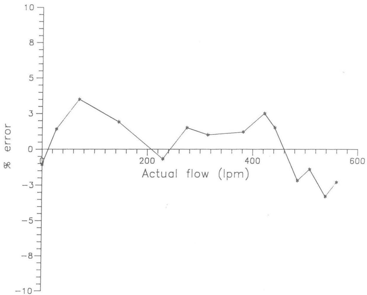
Fig. 5.8. Percentage error in the measured flow rate, with correction vs actual flow rate
