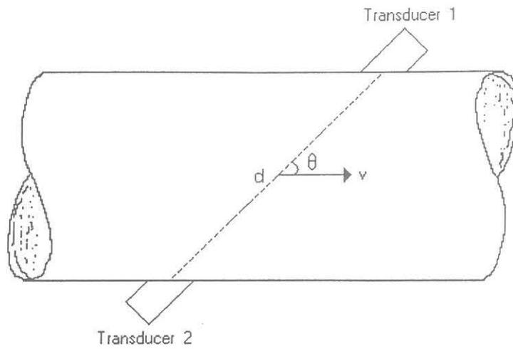
Fig. 2.3. Transducer arrangement in a transit time flowmeter
