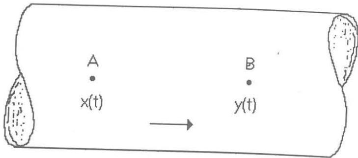
Fig. 2.2. Principle of cross correlation flowmeter
