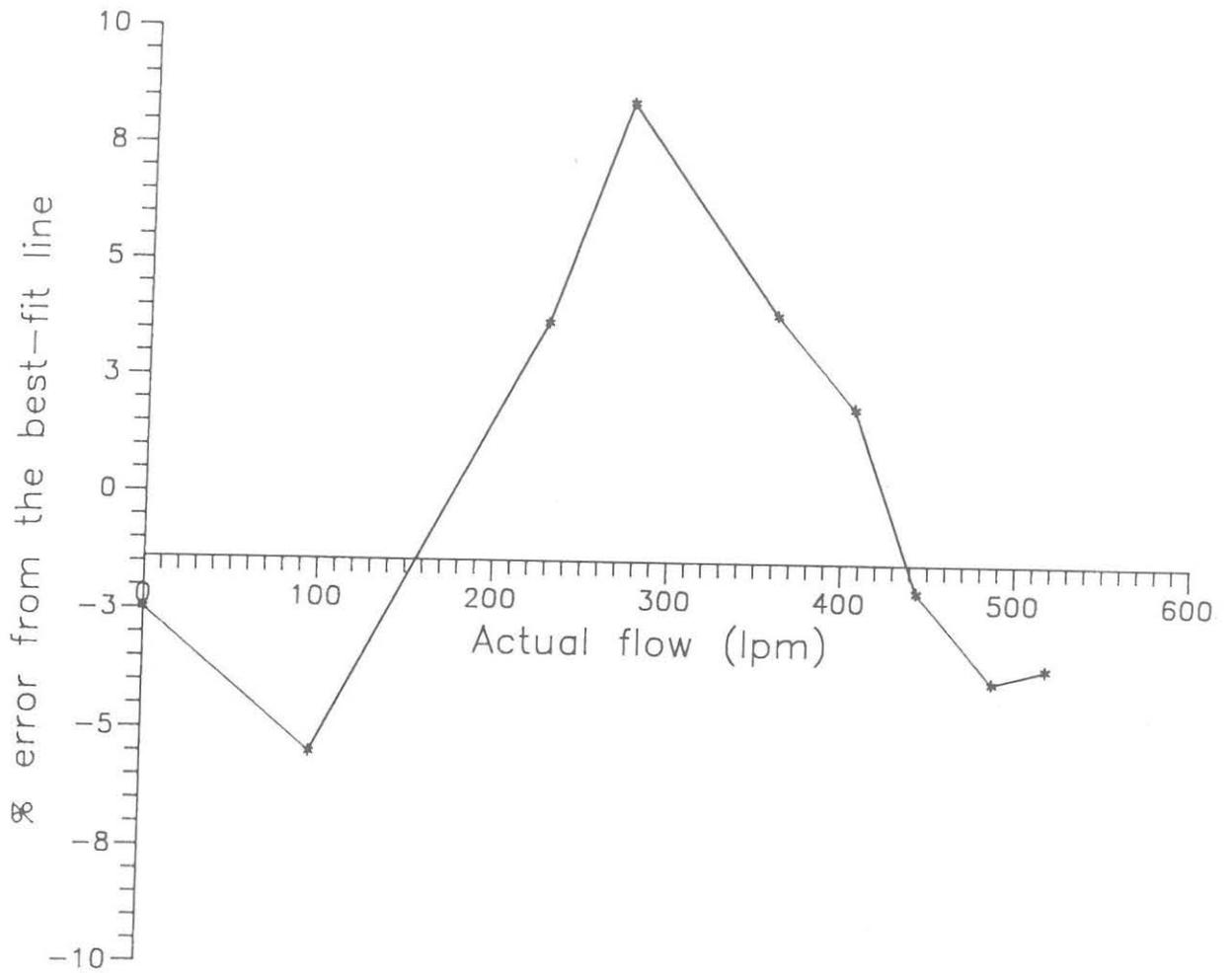
Fig. 5.4. Percentage error in the flow rate measured in single path transmission, from the best-fit line vs actual flow rate
