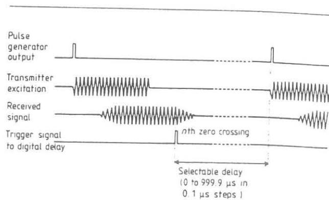
Fig. 2.6. Timing diagram of the narrow-band sing-around system
