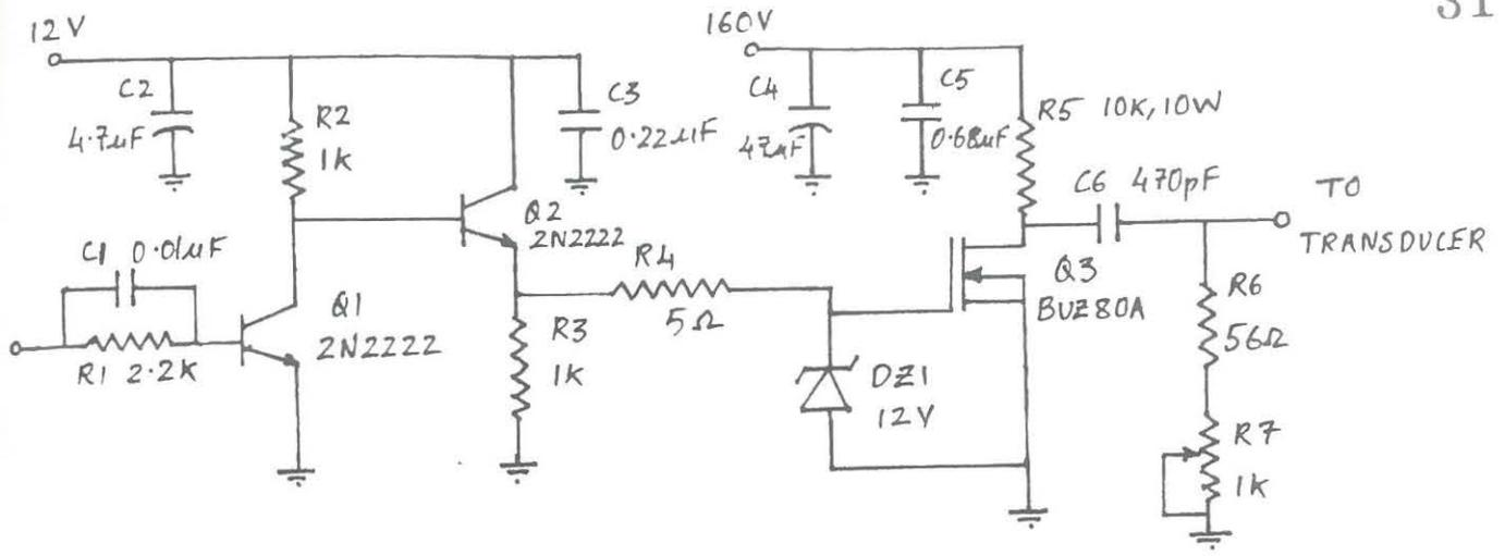
Fig. 3.6. Trigger and transmitter circuits
