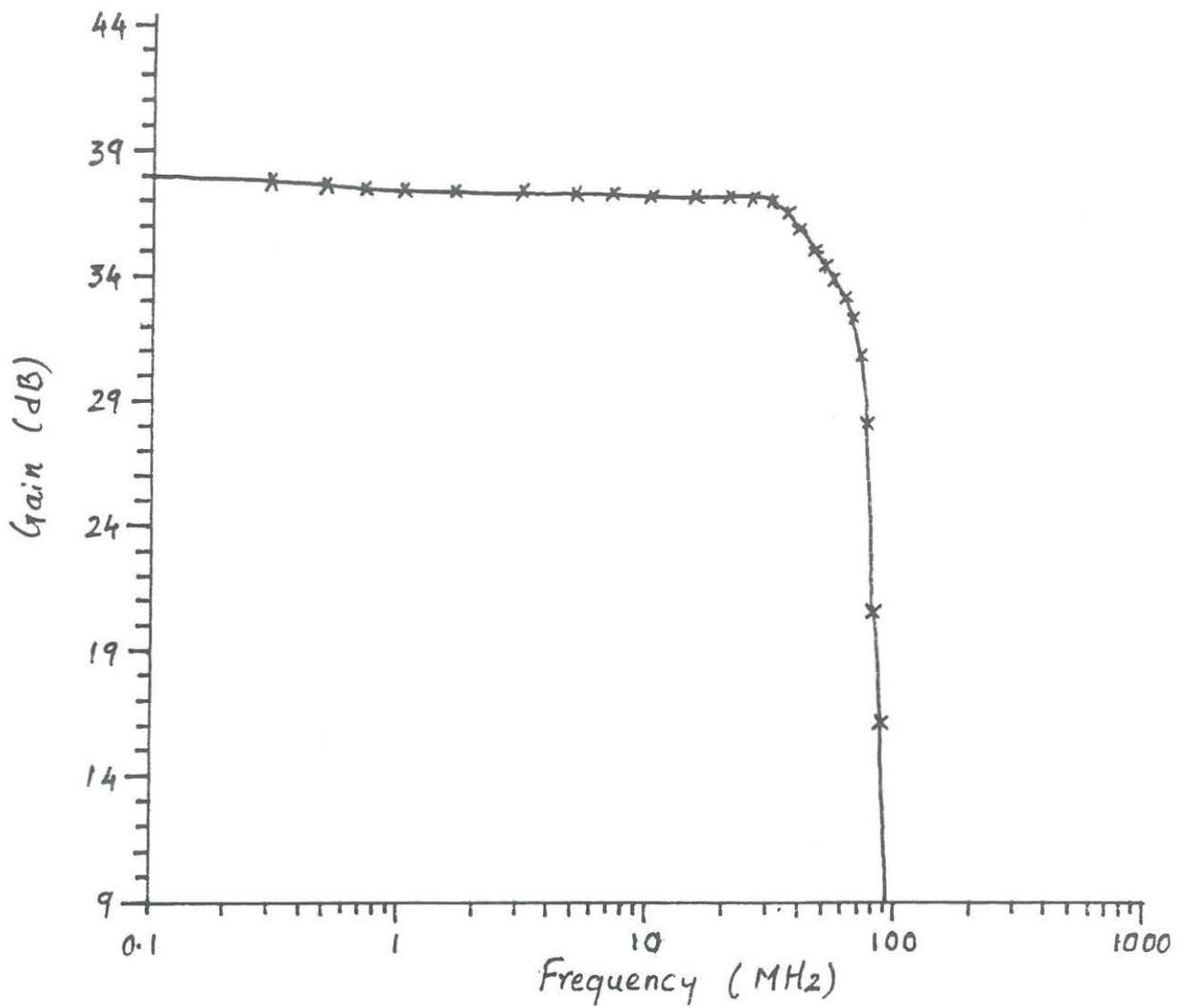
Fig. 3.11. Frequency response characteristic of receiver amplifier.
