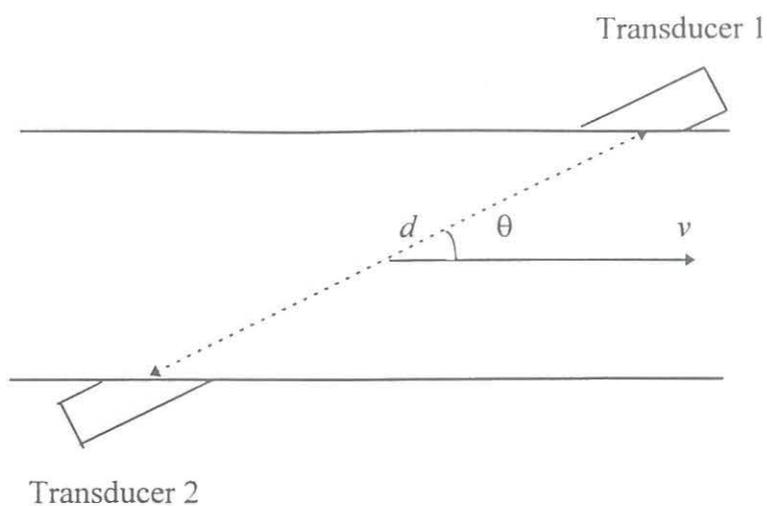
Fig. 2.1 Transducer arrangement in a transit time flowmeter
