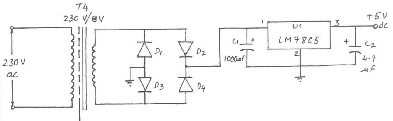
Fig. 3.21. Power supply for the measurement unit
