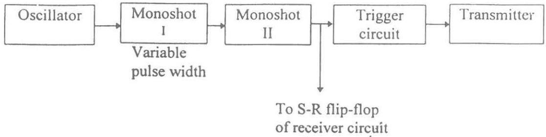
Fig. 3.4. Block diagram of the transmitter circuit
