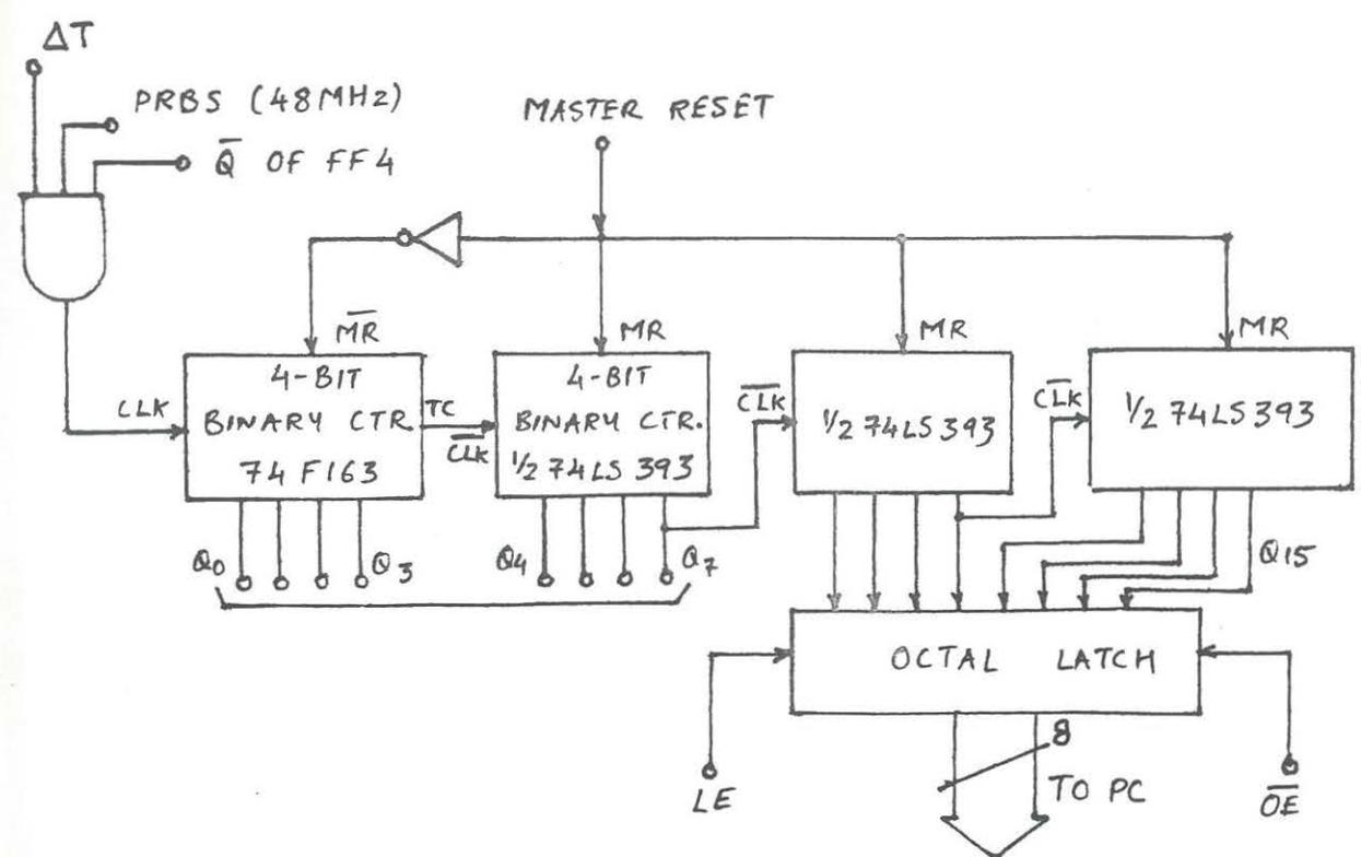
Fig. 3.16. Counter for transit time difference measurement
