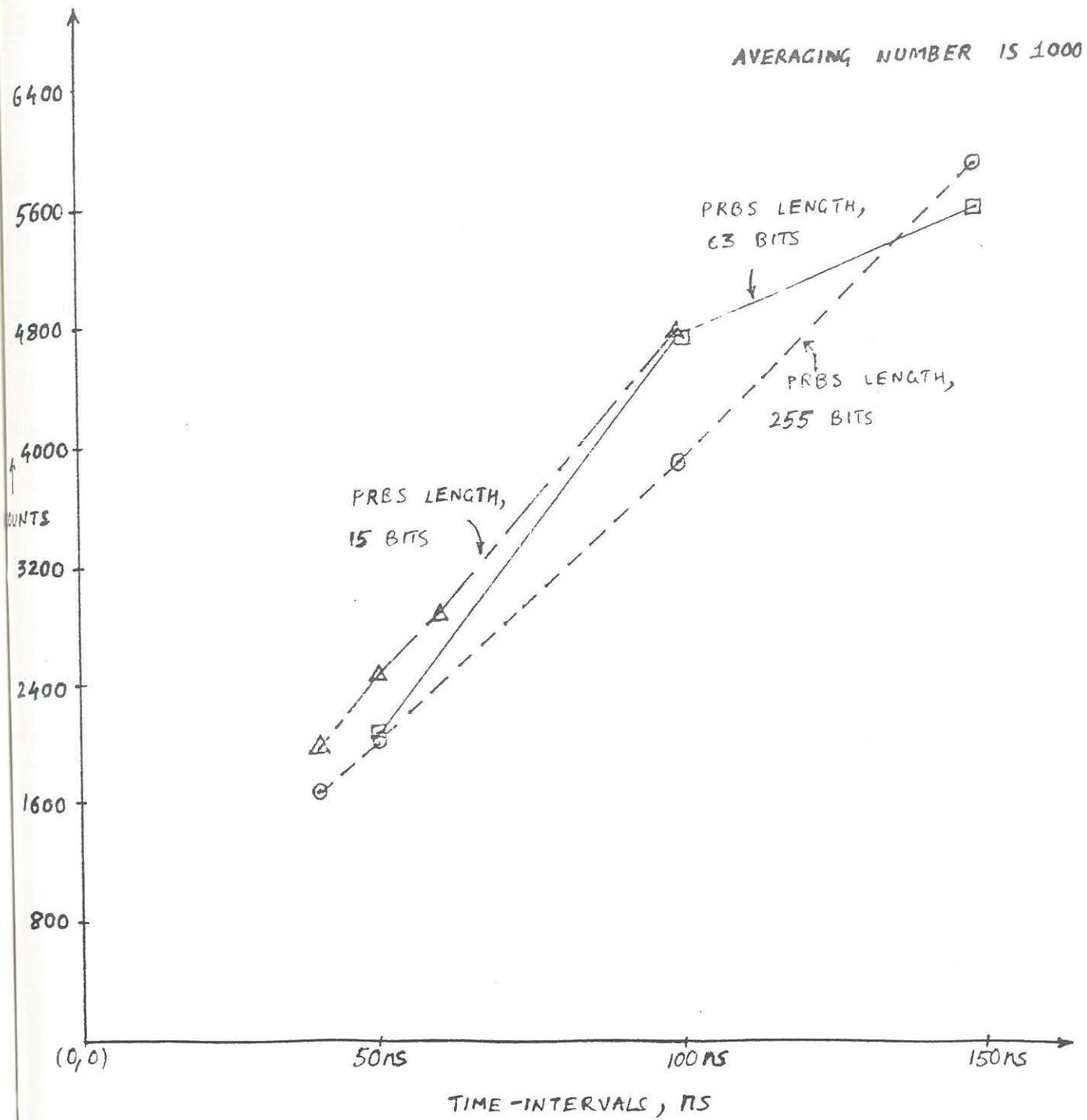
Fig. 4.2. Graph of results for different PRBSs
