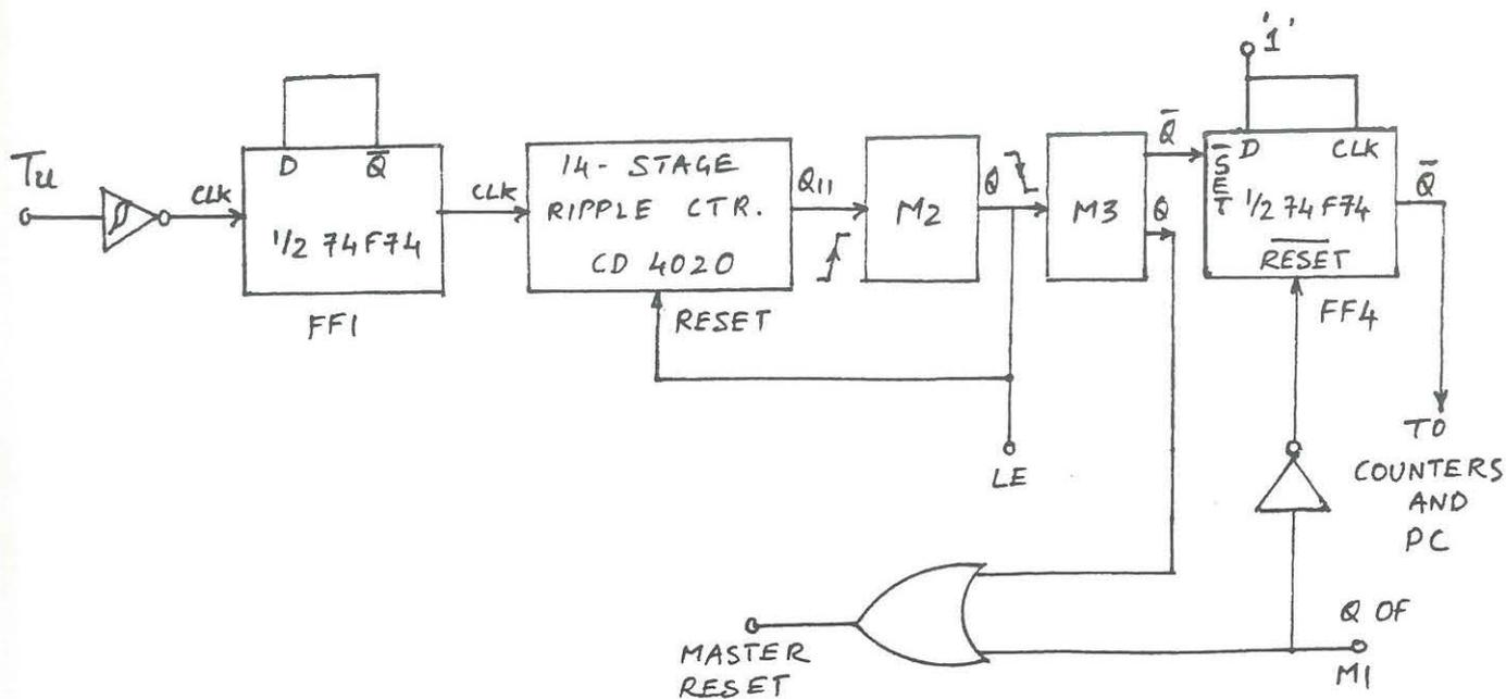
Fig. 3.18. Accumulating counter circuit
