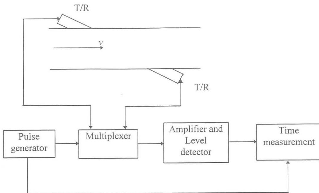
Fig. 2.3 Sequential direct transit time flowmeter scheme
