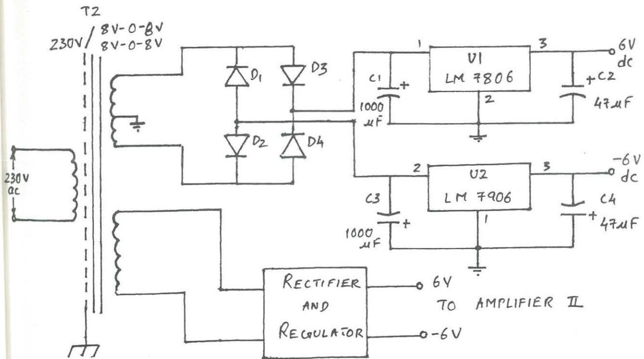
Fig. 3.10. Power supply for the amplifier circuit
