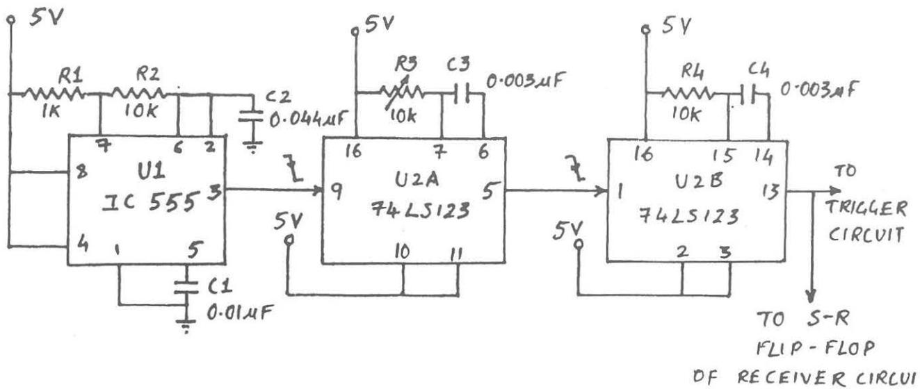
Fig. 3.5. Pulse train generator and delay circuits
