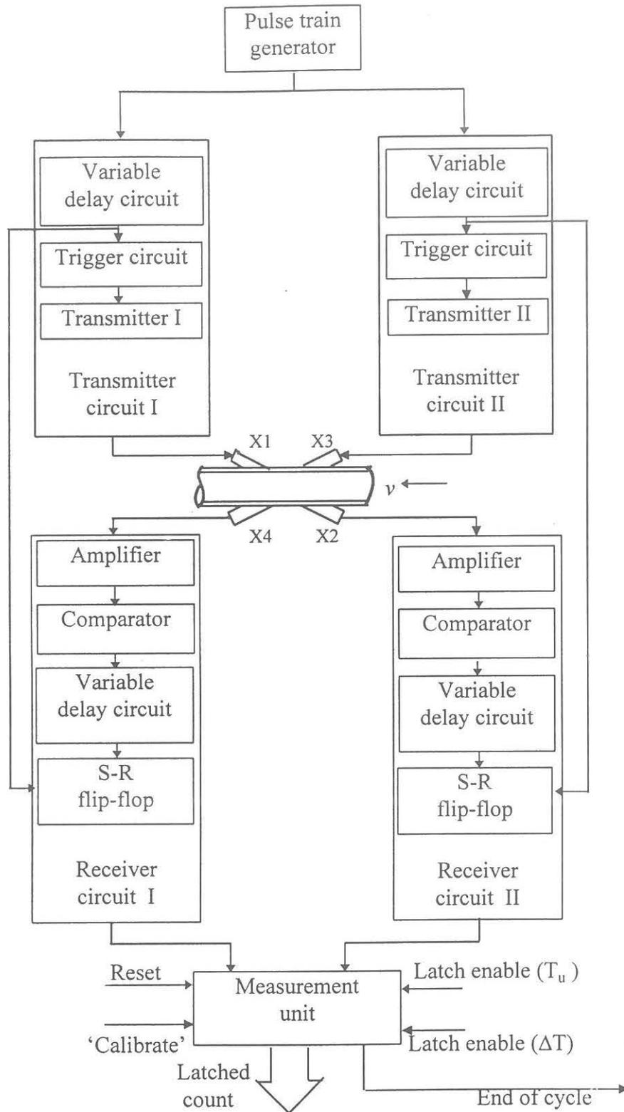
Fig. 3.2 Block diagram of the flowmeter system .
