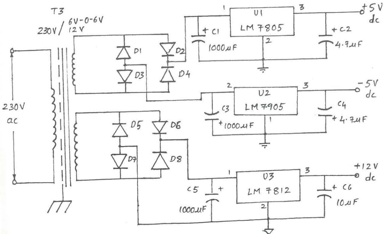
Fig. 3.13. Power supply for the comparator circuit
