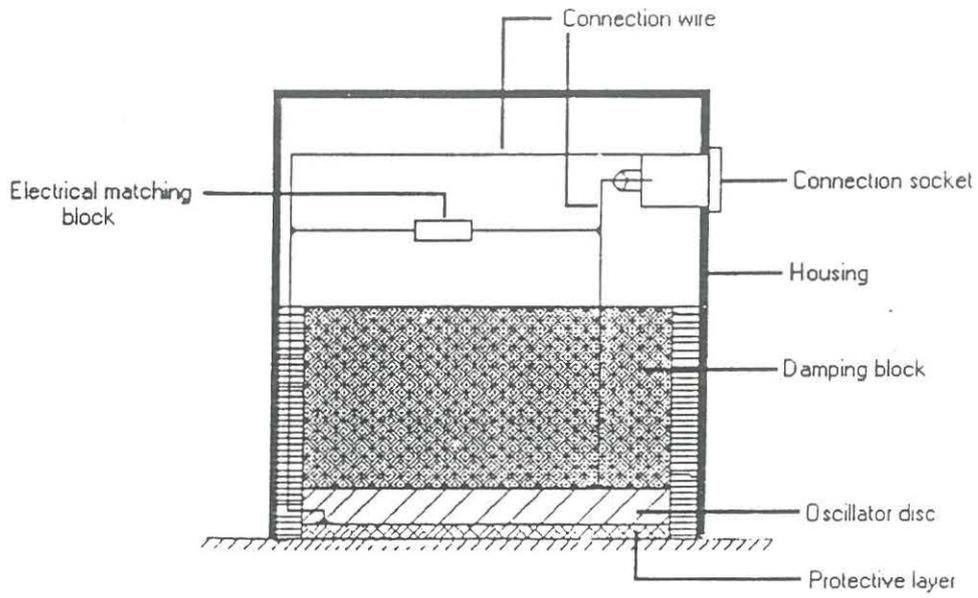
Fig. 3.3. Schematic of an ultrasound transducer
