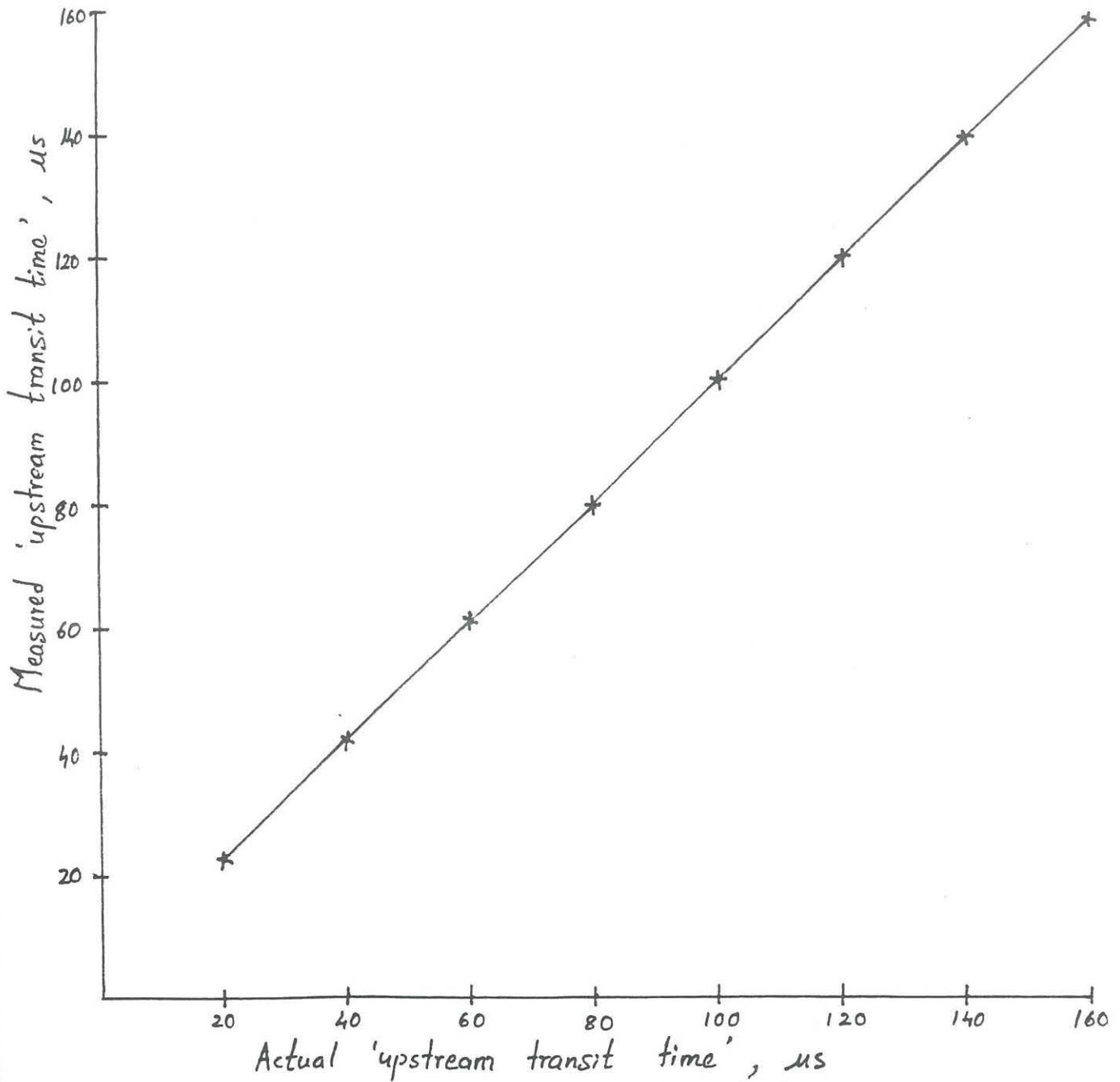
Fig. 4.4. Measured 'upstream transit time' vs Actual 'upstream transit time'.
