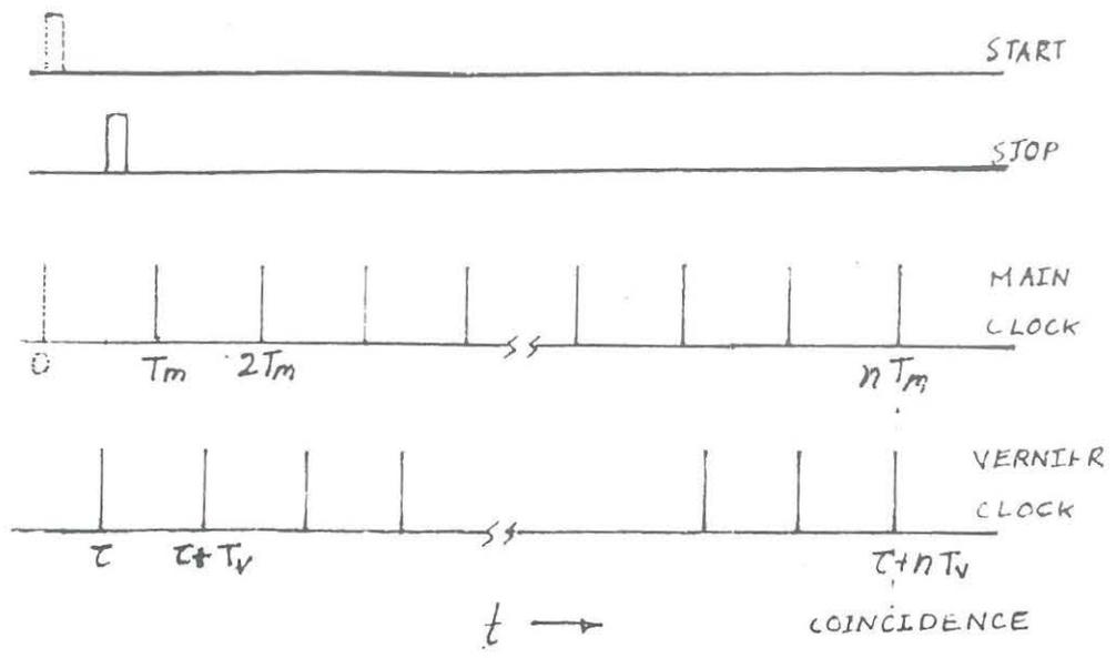
Fig. A.1. Principle of vernier technique
