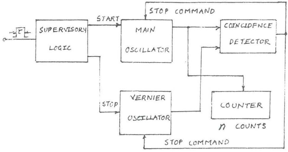
Fig. A.2. Block schematic for vernier technique
