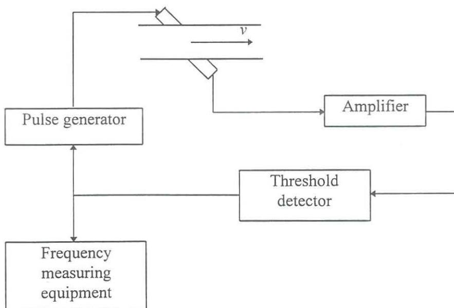
Fig. 2.2 Block diagram showing 'sing-around' principle
