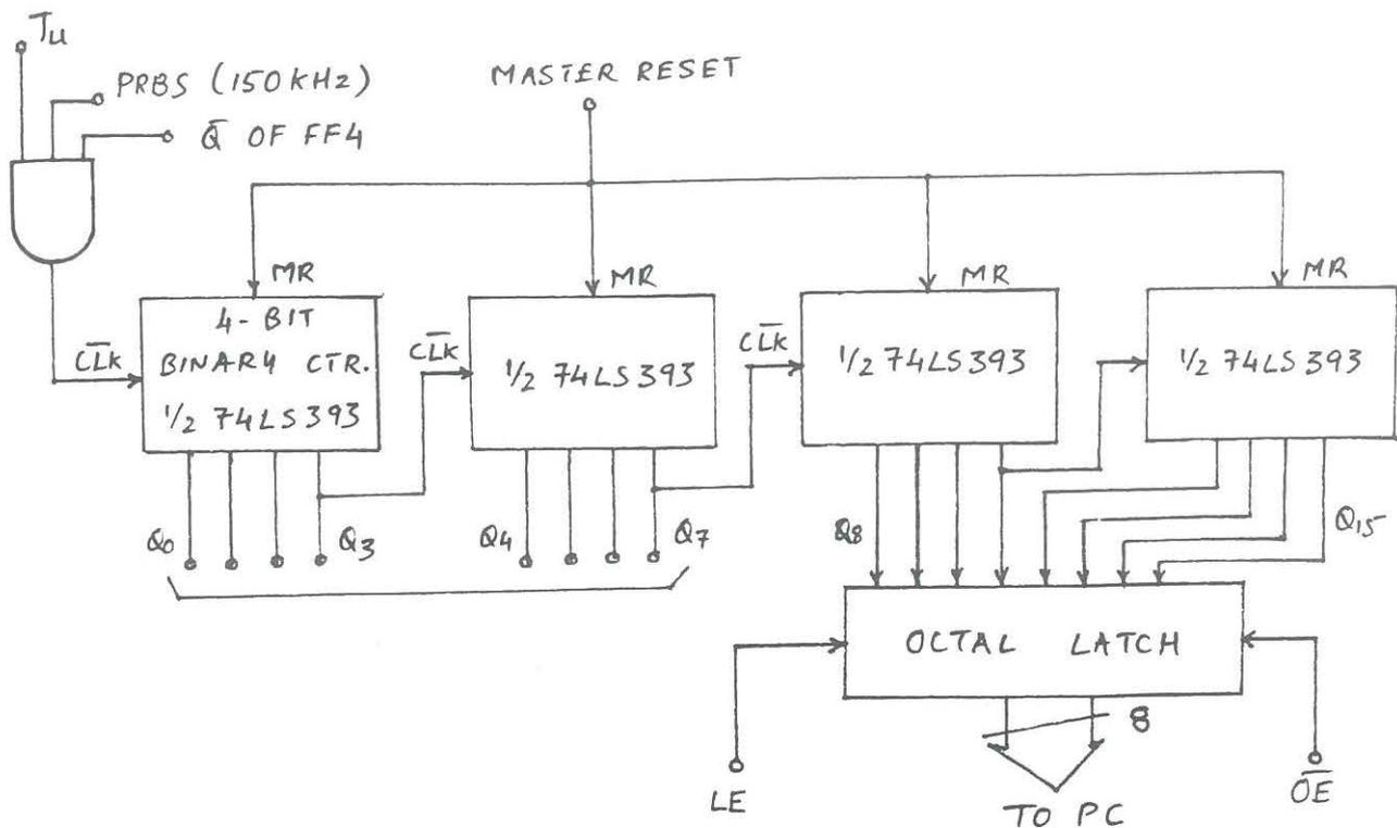
Fig. 3.17. Counter for upstream transit time measurement
