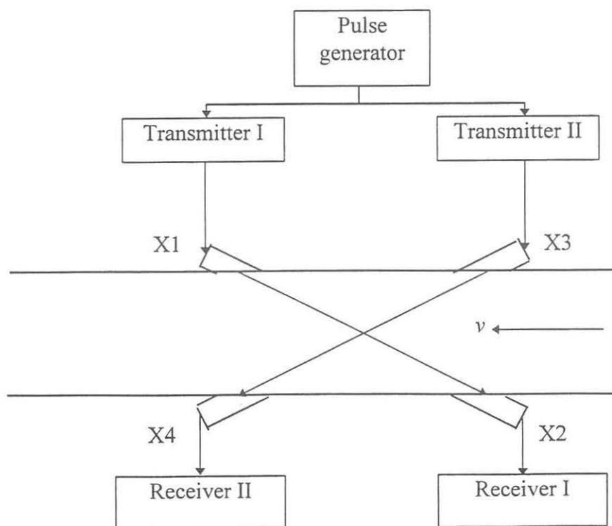
Fig. 2.4 Simultaneous direct transit time flowmeter scheme
