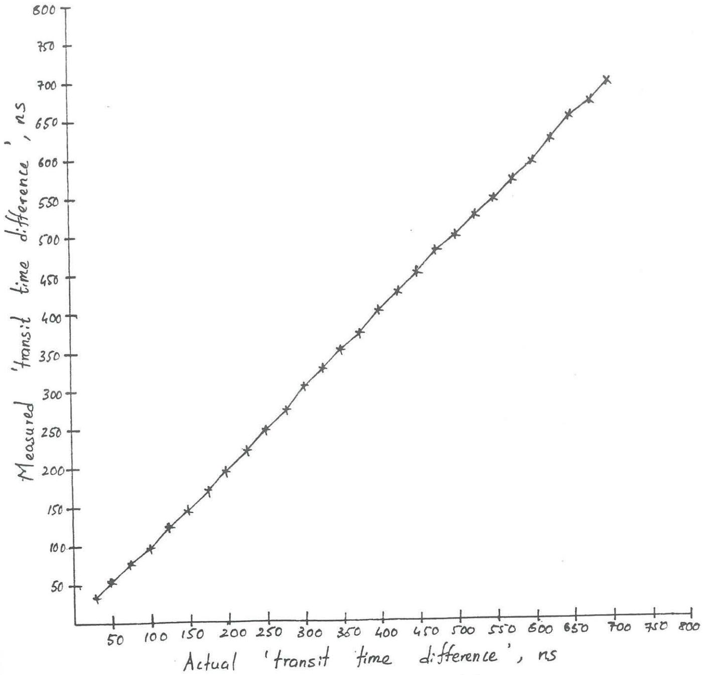
Fig. 4.3. Measured, 'transit time difference' vs Actual 'transit time difference'
