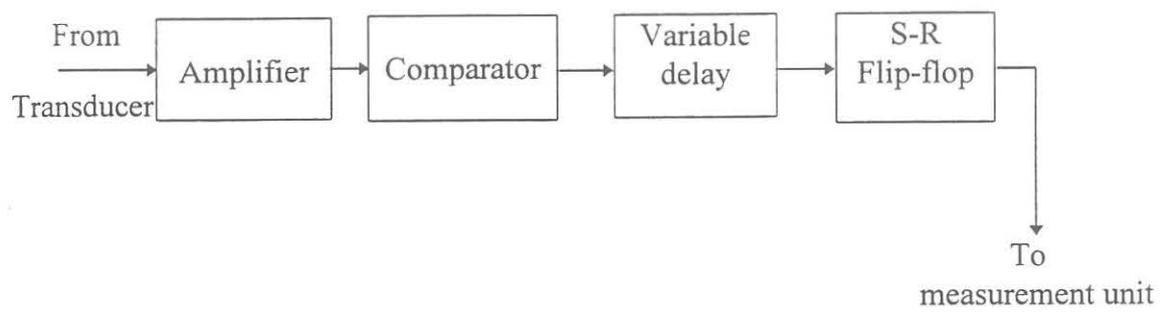
Fig. 3.8 Block schematic of receiver circuit
