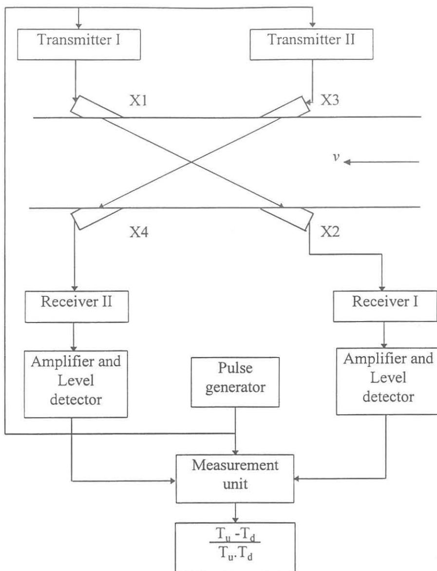
Fig. 3.1 Simultaneous transit time flowmeter scheme
