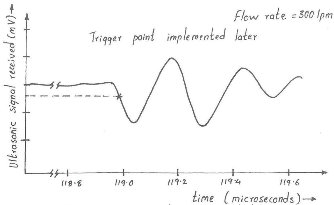
Fig. 4.6 Trigger points implemented
