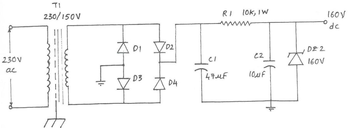
Fig. 3.7. Power supply for the transmitter
