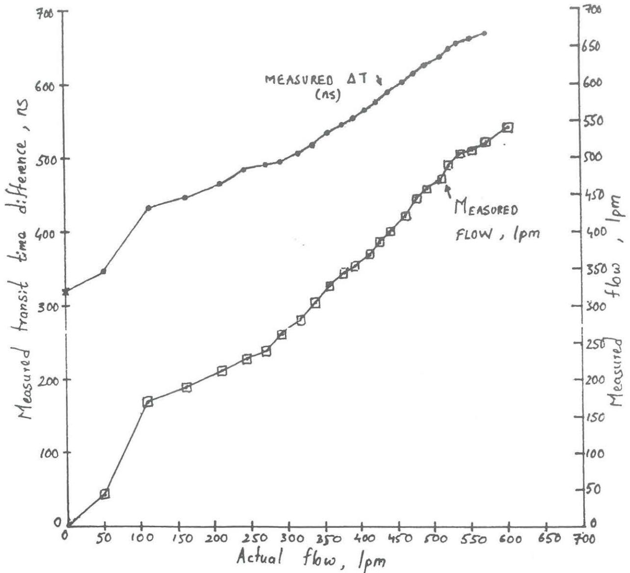
Fig. 4.8. Measured transit time difference and Measured flow rate vs Actual flow rate.
