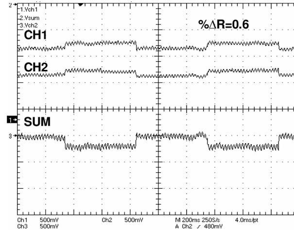
Fig. 5.8 Output waveforms of Channel-1, Channel-2, and summing amplifier for exc. freq = 100 kHz;  $R = 196 \Omega$ ,  $f = 1 \text{ Hz}$ ,  $\Delta R/R = 0.6\%$ , variation = square
