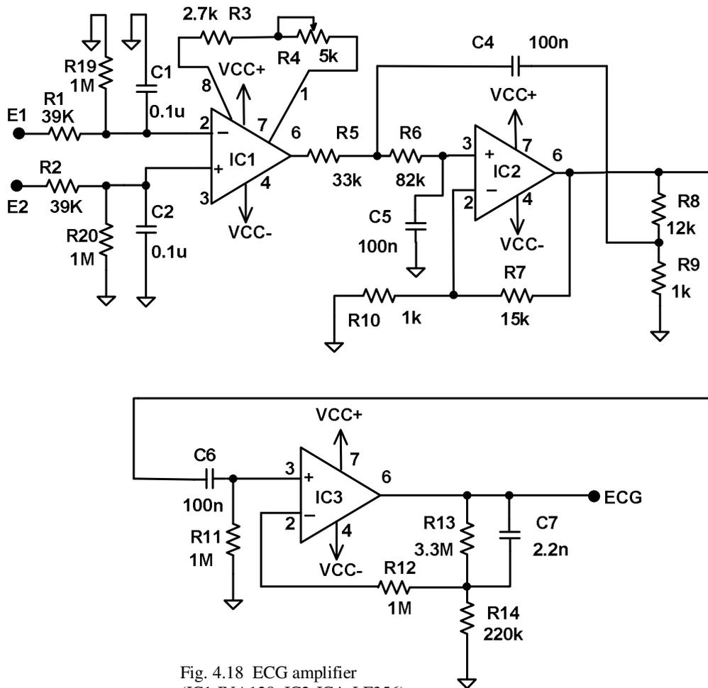
Fig. 4.18 ECG amplifier
