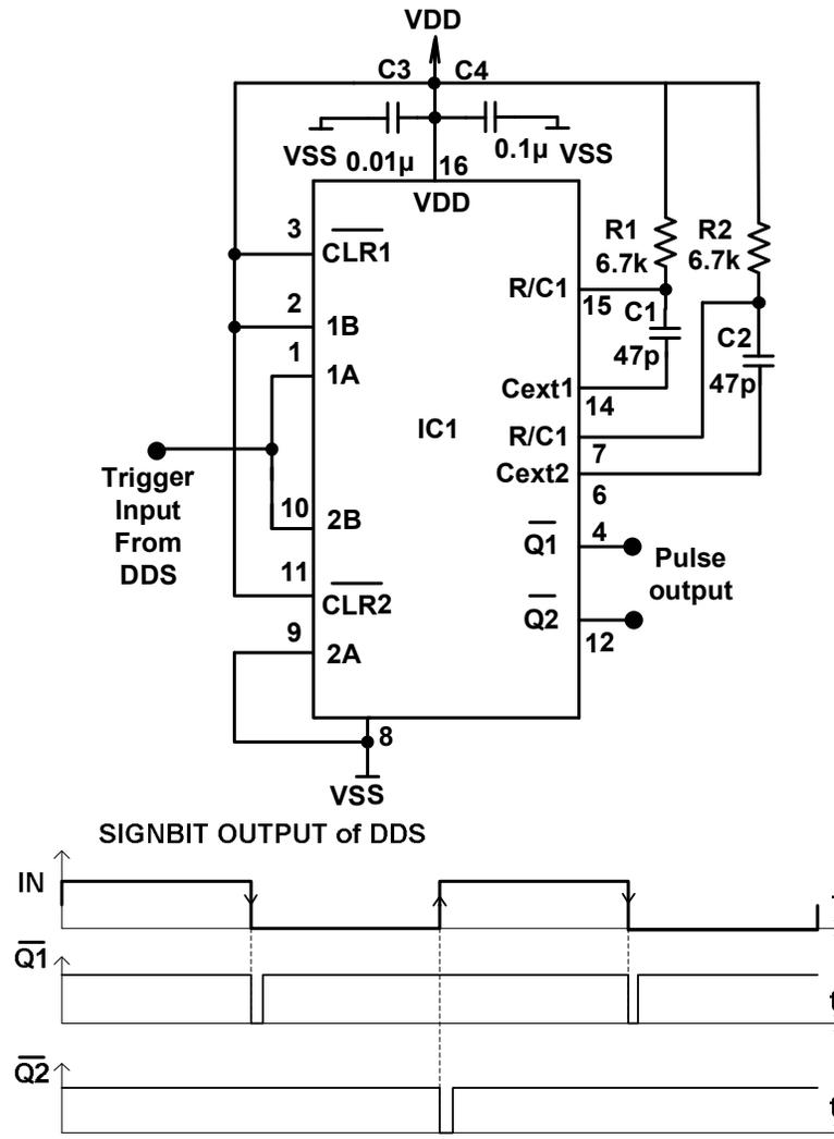
Fig. 4.16 Monostable multivibrator using IC1: SN74221 [38]
