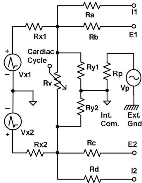
Fig.3.2 Schematic of the thorax simulator
