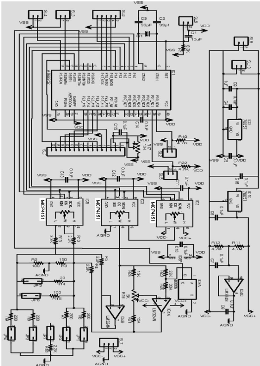
Fig. B.1 Schematic diagram of the thorax simulator
