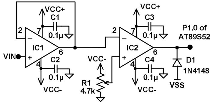
Fig. 4.21 High contact impedance indicator [16].
