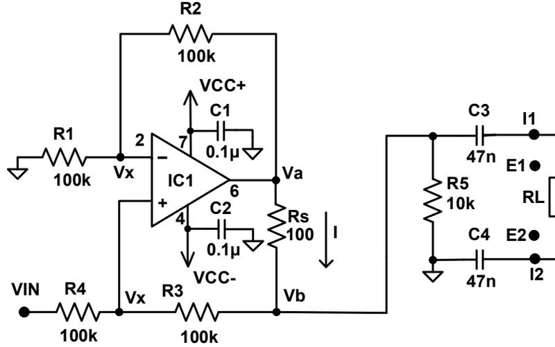
Fig. 4.7 V-to-I converter based on modified Howland current source [25], [26], [27]. (IC1: LF 356)
