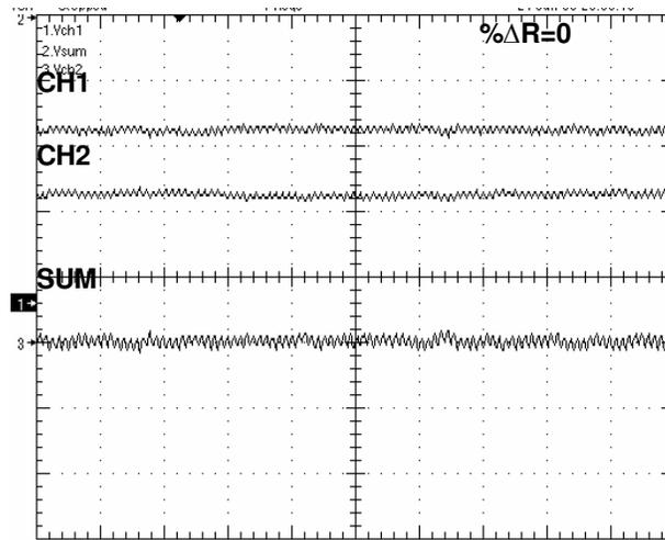
Fig. 5.10 Output waveforms of Channel-1, Channel-2, and summing amplifier for exc.  $f = 50 \text{ kHz}$ ;  $R = 196 \Omega$ ,  $f = 1 \text{ Hz}$ ,  $\Delta R/R = 0 \%$ , variation = sinusoidal
