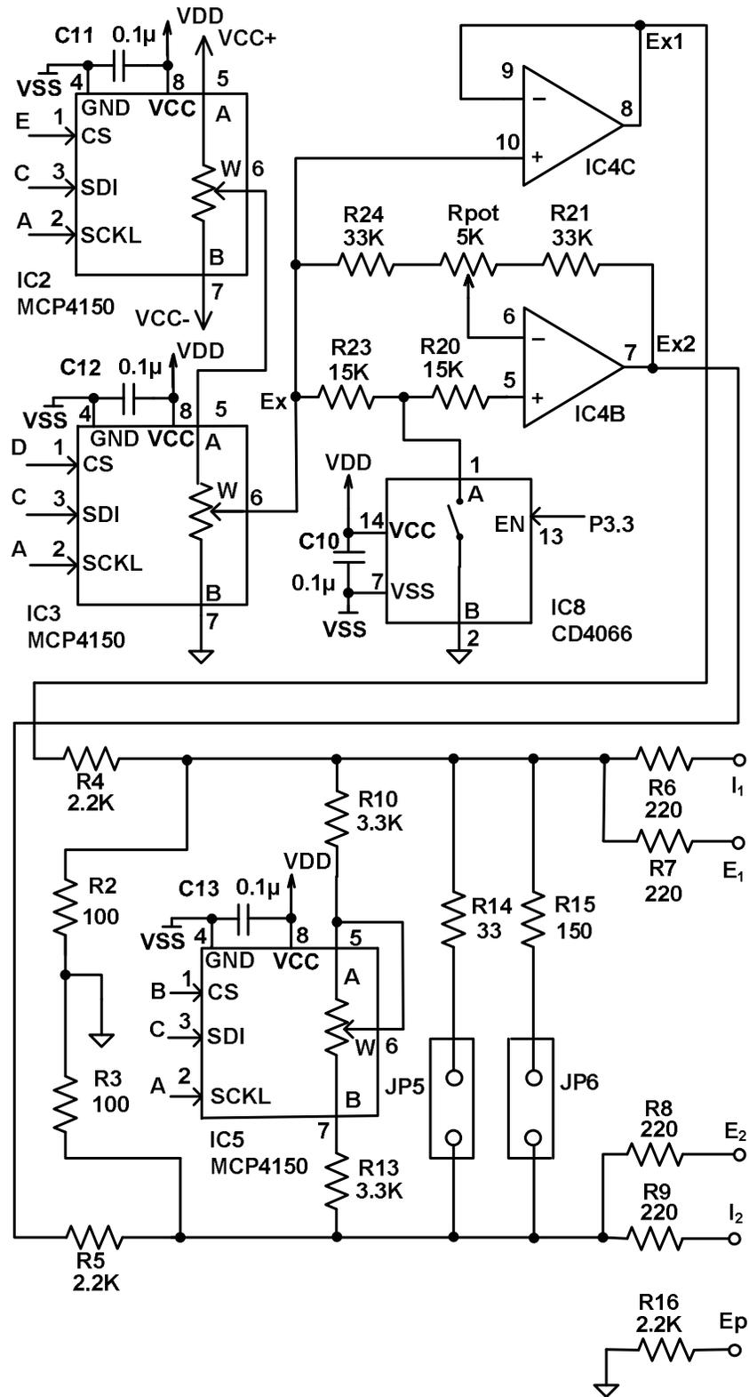
Fig. 3.3 Thorax simulator circuit
