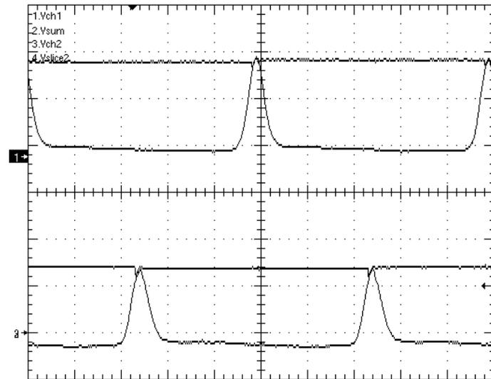
Fig. 5.3 Output waveforms of two channels of slicing and sampling for  $f = 100$  kHz
