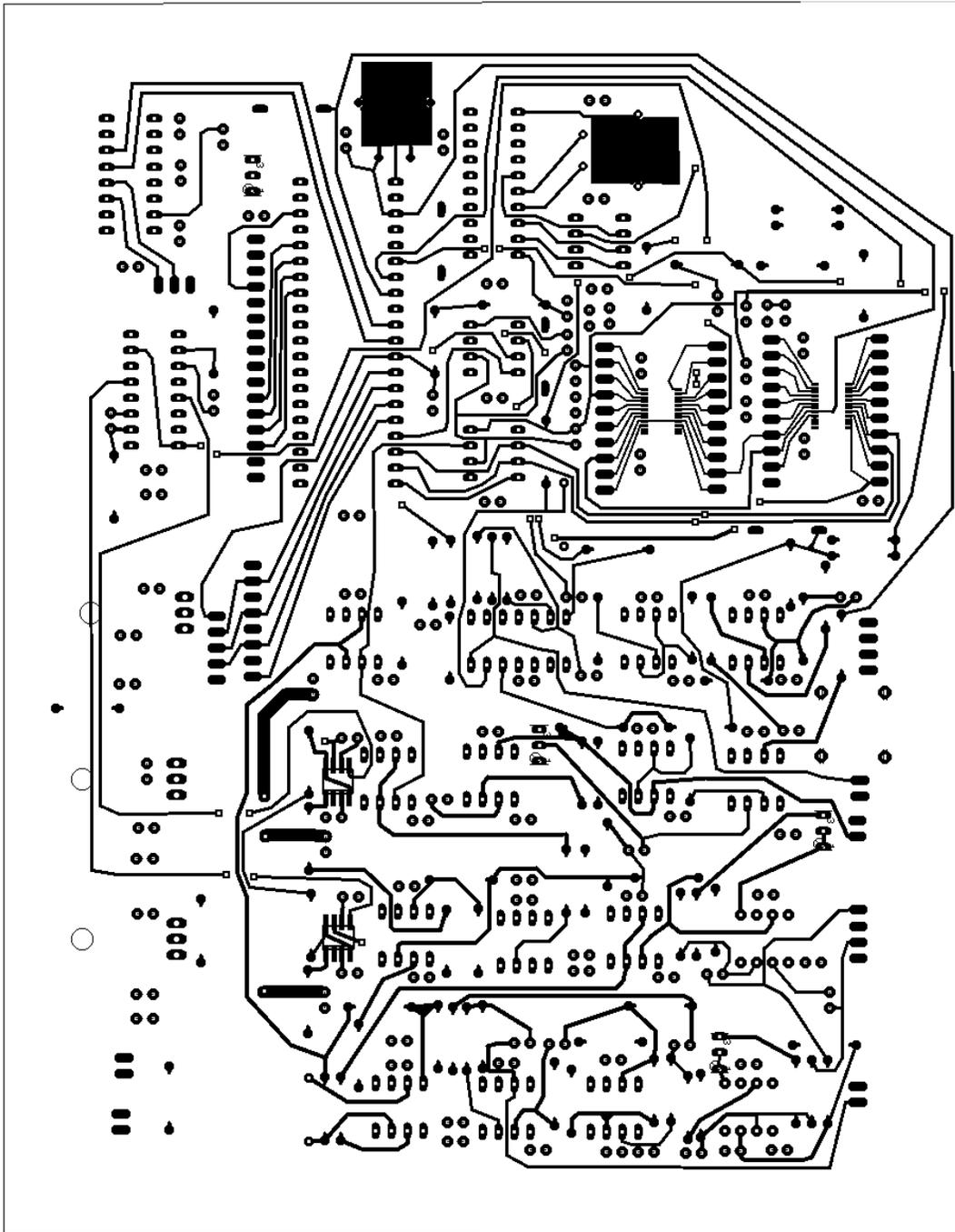
Fig. E.2 Component side of impedance cardiograph PCB (20 cm × 15 cm)
