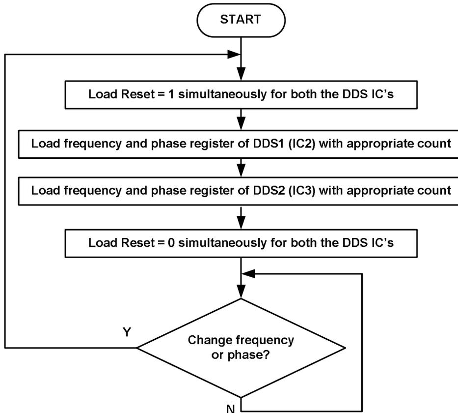
Fig. 4.4 Flowchart of the microcontroller program for DDS synchronization for phase shifted outputs
