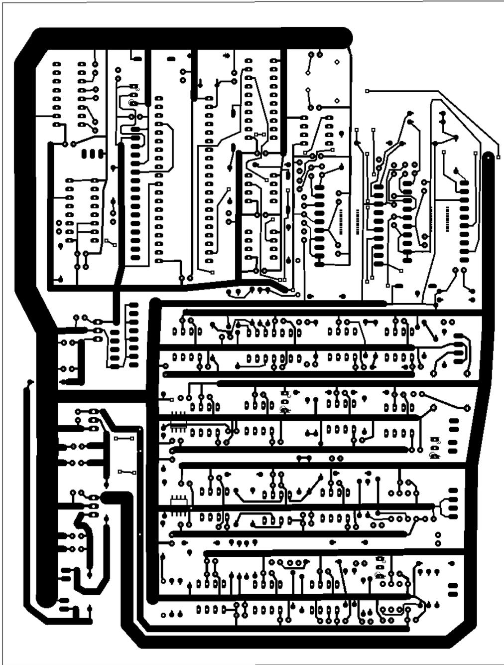
Fig. E.3 Solder side of impedance cardiograph PCB (20 cm × 15 cm)
