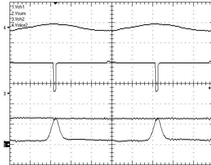
Fig. 5.2 Output waveforms of slicing amplifier using voltage clamp amplifier IC AD8037 for  $f = 100$  kHz
