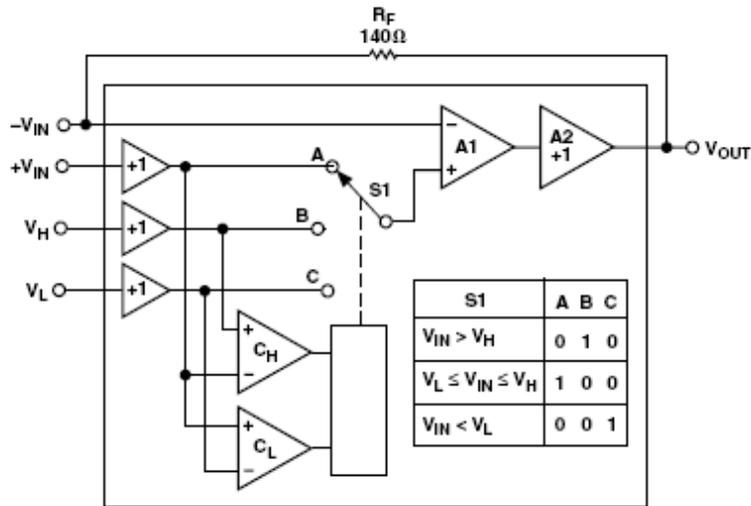
Fig. A.1 Internal block diagram of AD 8037
