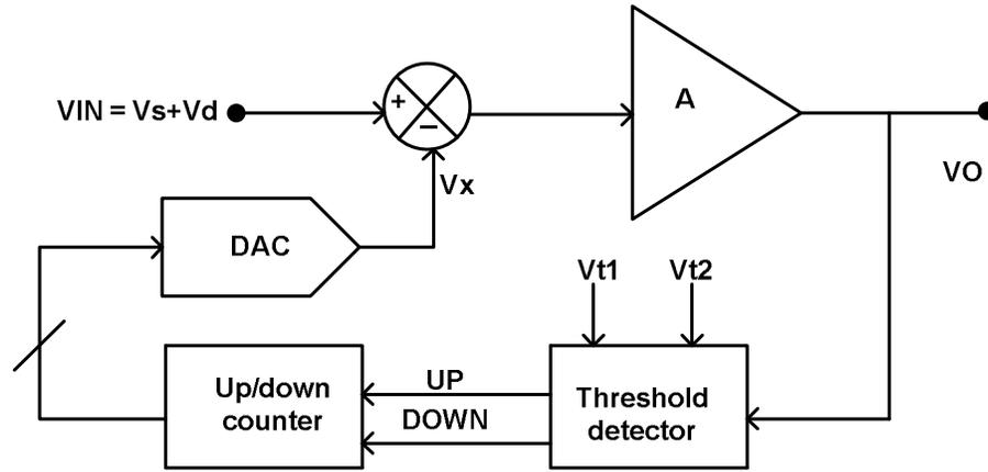
Fig. 4.19 Block diagram of tracking based baseline restoration circuit [22], [23]
