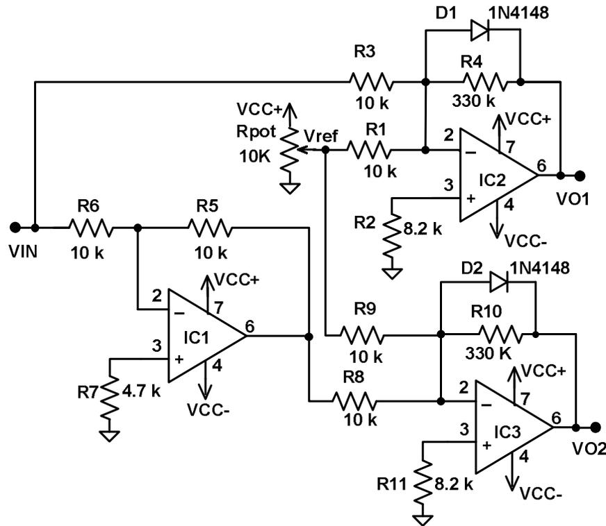
Fig. 4.9 Diode based slicing amplifier (IC1 - IC3: LF 356)
