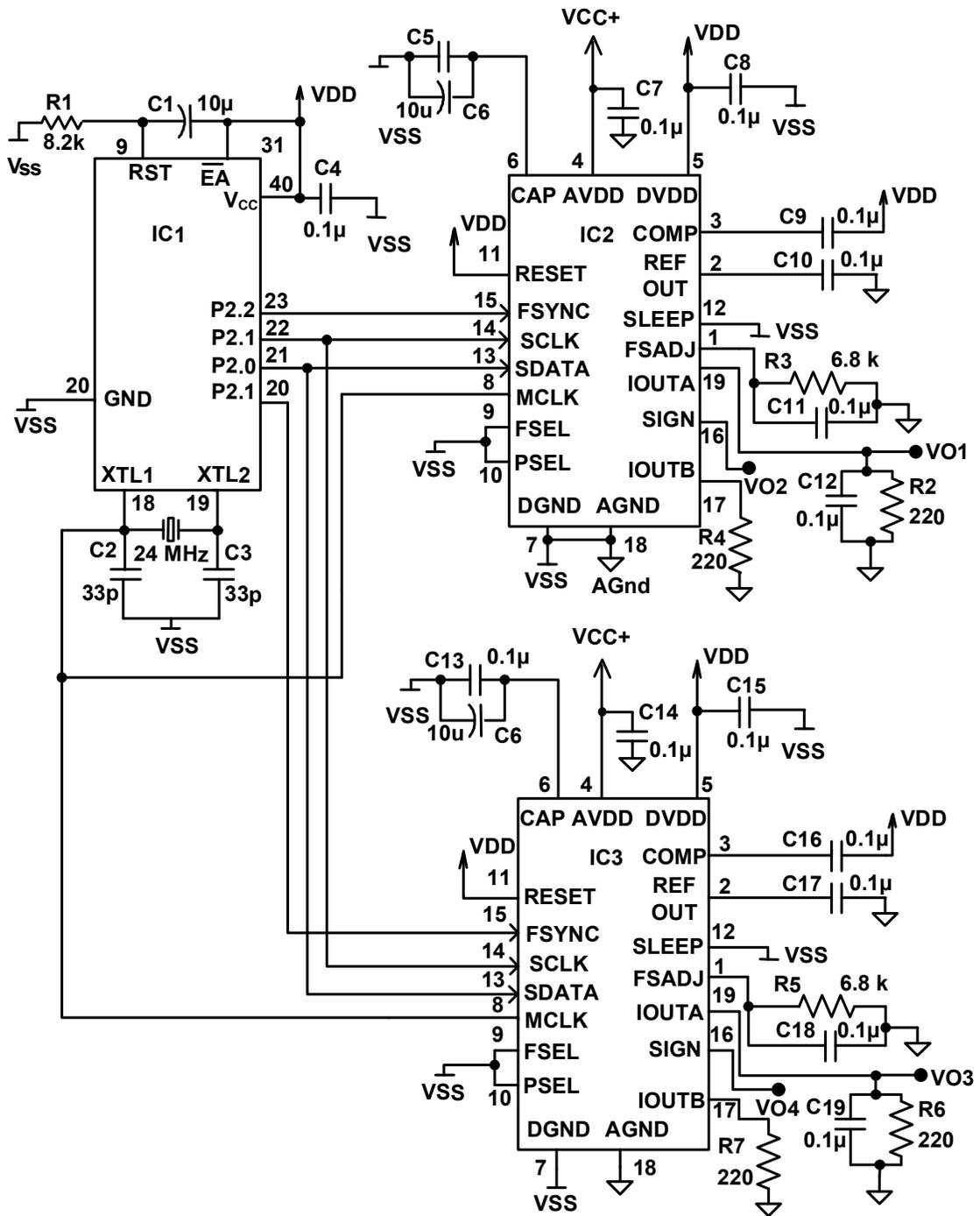
Fig. 4.3 Programmable source using AD9834 for outputs with a settable phase difference
