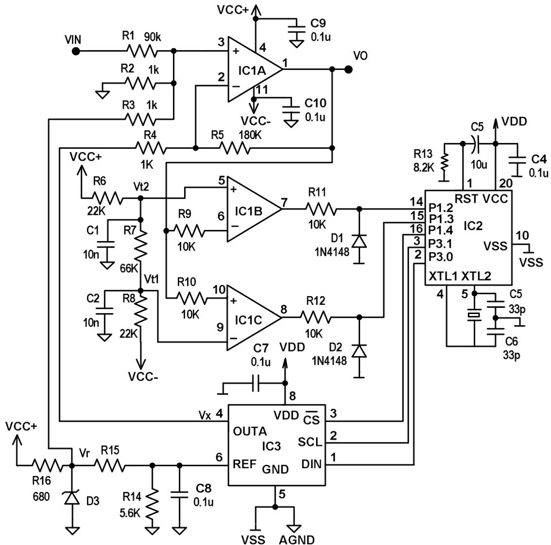
Fig. 4.20 Baseline restoration circuit [22], [23] (IC1: LM324, IC2: AT89C2051, IC3: TLV5618)
