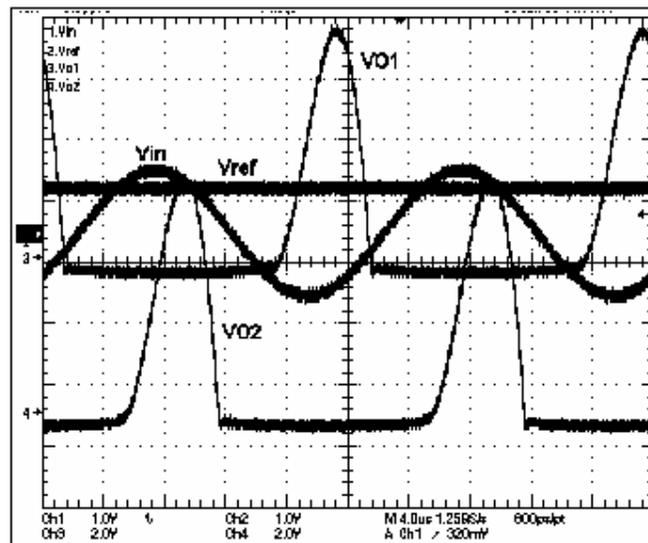
Fig. 5.1 Output waveforms of diode based slicing amplifier for  $f = 50$  kHz
