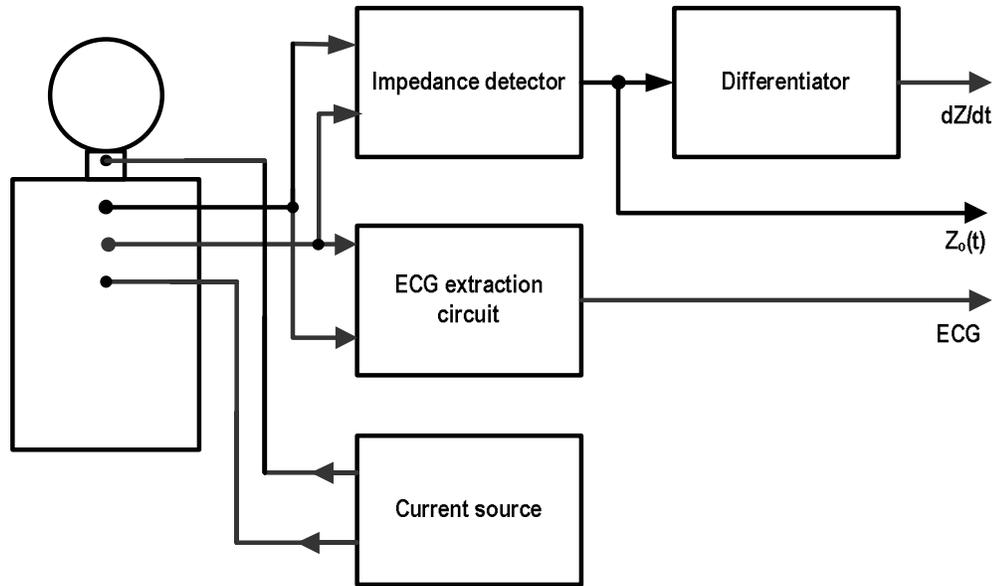
Fig. 2.4 Block diagram of impedance cardiograph
