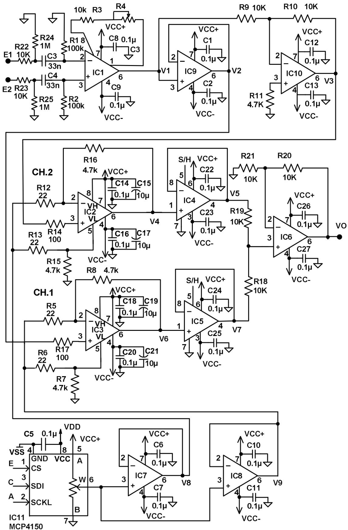
Fig. 4.17 Two-channel slicing and sampling
