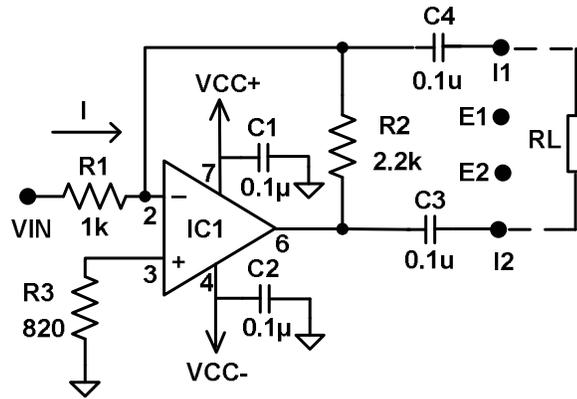
Fig. 4.5 V-to-I converter based on inverting amplifier circuit [16], [27] (IC1: LF 356)
