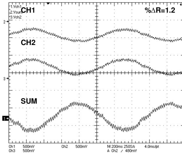
Fig. 5.5 Output waveforms of Channel-1, Channel-2, and summing amplifier for exc. freq = 100 kHz;  $R = 196 \Omega$ ,  $f = 1 \text{ Hz}$ ,  $\Delta R/R = 1.2\%$ , variation = sinusoidal
