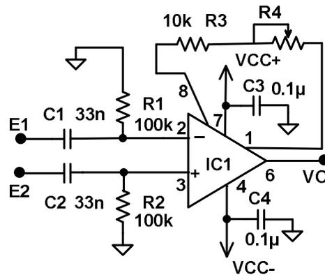
Fig. 4.8 Difference amplifier using INA 128
