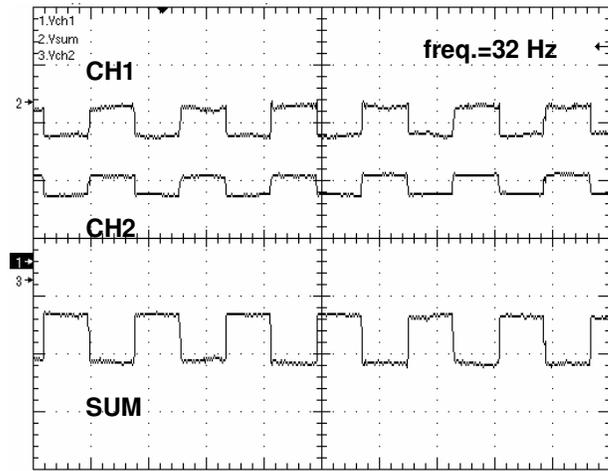
Fig. 5.9 Output waveforms of Channel-1, Channel-2, and summing amplifier, for exc.  $f = 50 \text{ kHz}$ ;  $R = 196 \Omega$ ,  $f = 32 \text{ Hz}$ ,  $\Delta R/R = 1.2\%$ , variation = square.
