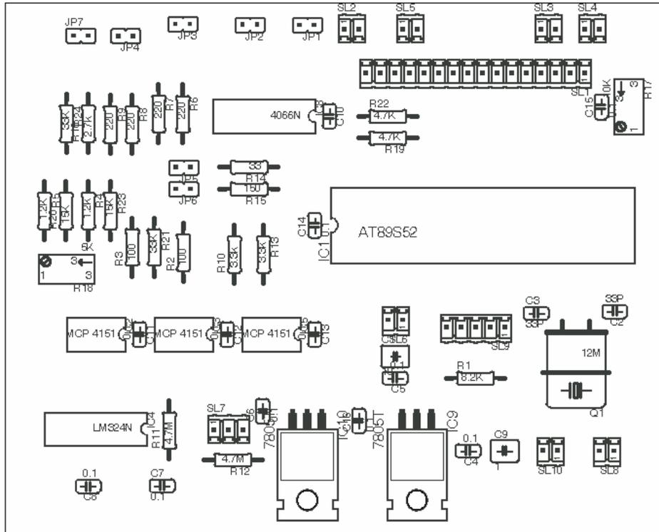
Fig. C.1 Component placement layout of thorax simulator PCB (12.5 cm x 9.5 cm)
