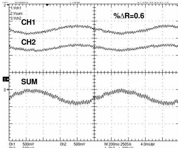
Fig. 5.7 Output waveforms of Channel-1, Channel-2, and summing amplifier for exc. freq = 100 kHz;  $R = 196 \Omega$ ,  $f = 1 \text{ Hz}$ ,  $\Delta R/R = 0.6 \%$ , variation = sinusoidal
