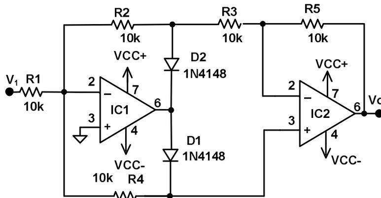
Fig. 4.11 Precision full-wave rectifier (IC1,IC2: LF356) [6], [13]-[16]
