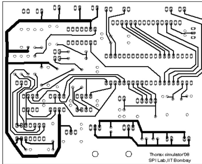
Fig. C.2 Component side of thorax simulator PCB (12.5 cm × 9.5 cm)
