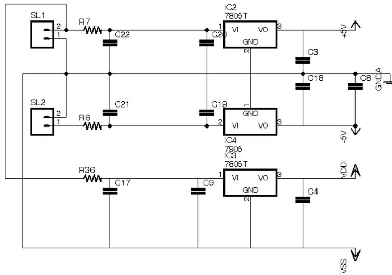
Fig. D.1 Schematic diagram of the power supply as the part of the impedance cardiography hardware
