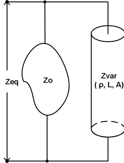
Fig. 2.2 Parallel column impedance model [1], [4]
