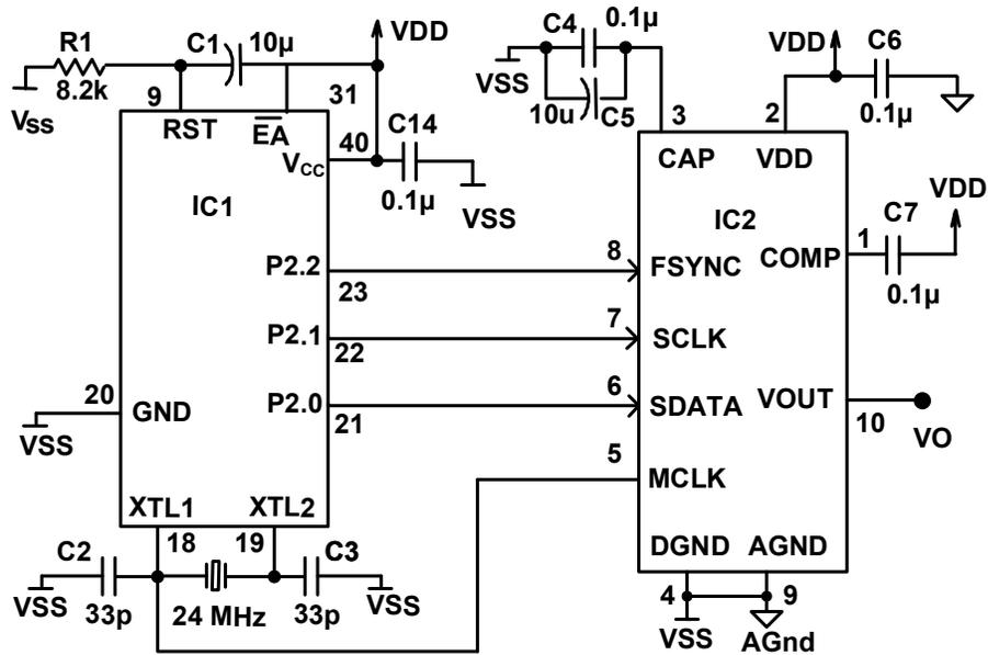
Fig. 4.1 The programmable source using DDS AD9833 [ 34]
