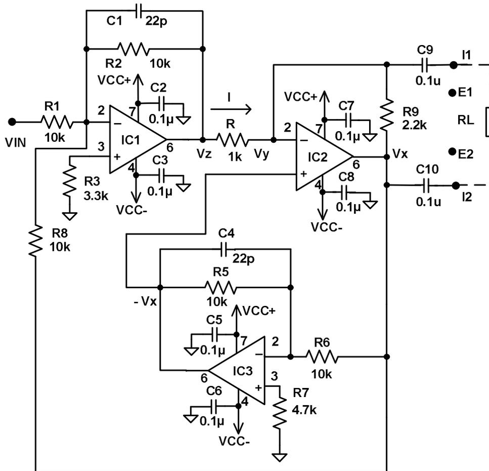
Fig. 4.6 Balanced current source [13], [14]. (IC1 - IC3: LF 356)
