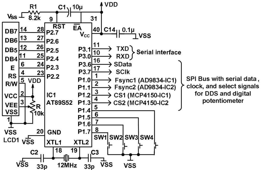
Fig. 4.22 Controller circuit
