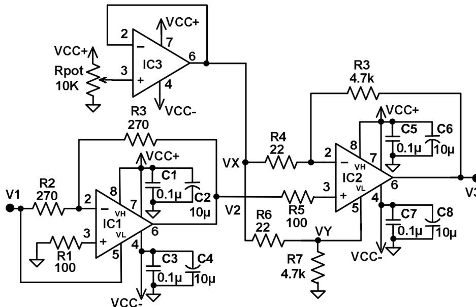
Fig. 4.13 Slicing amplifier using voltage clamp amplifier AD8037 (IC1: LF356, IC2 and IC3: AD8037)
