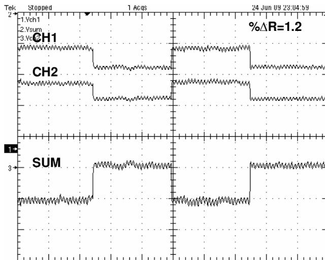
Fig. 5.6 Output waveforms of Channel-1, Channel-2, and summing amplifier for exc. freq = 100 kHz;  $R = 196 \Omega$ ,  $f = 1 \text{ Hz}$ ,  $\Delta R/R = 1.2\%$ , variation = square.
