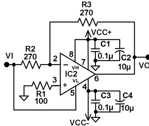
Fig. 4.12 Precision full-wave rectifier using voltage clamp amplifier IC AD8037
