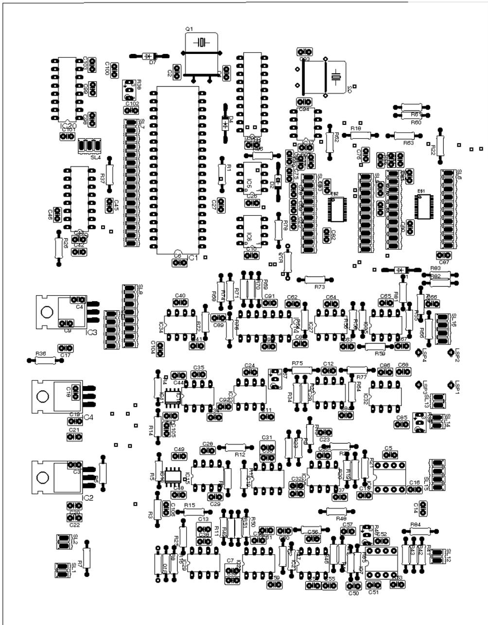
Fig. E.1 Components placement of impedance cardiography PCB (20 cm × 15 cm)
