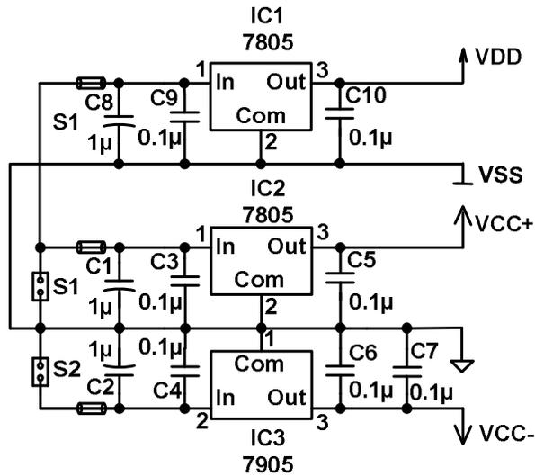
Fig. 4.23 Power supply circuit
