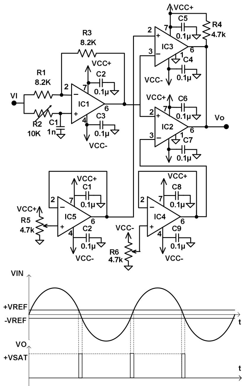
Fig. 4.15 Sampling pulse generation at zero crossing, using IC1, IC4, IC5: LF356, IC2 and IC3:LM311
