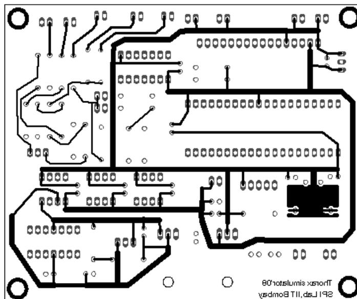
Fig. C.3 Solder side of thorax simulator PCB (12.5 cm × 9.5 cm)
