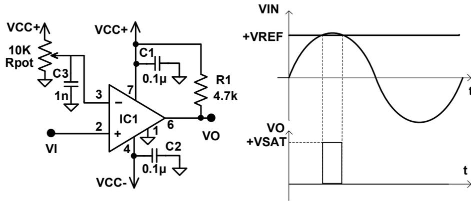
Fig. 4.14 Sampling pulse generator at the positive peak using comparator IC LM311
