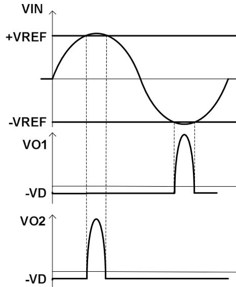
Fig. 4.10 Output waveforms VO1 and VO2 of the diode based slicing amplifier
