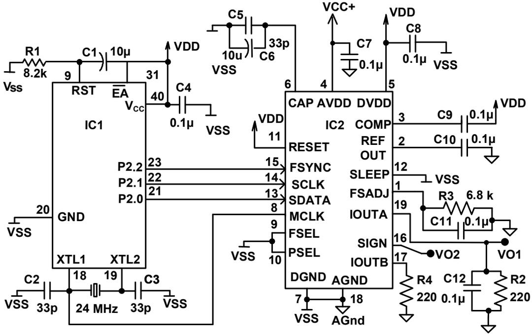
Fig. 4.2 The programmable source using DDS AD9834 [35]
