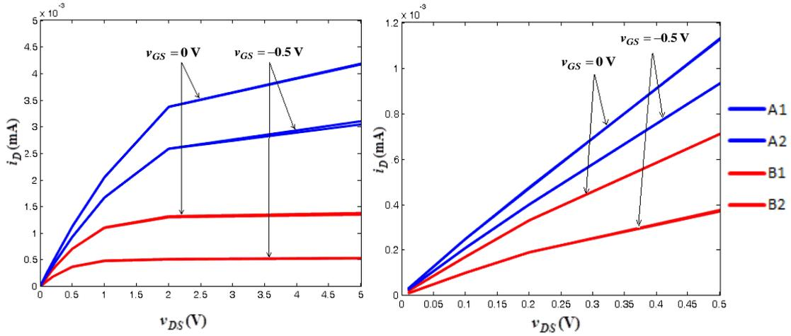
**Figure 3.24:** Drain characteristics of the JFETs on two pieces of U441 (A1 and A2: two devices on package A, B1 and B2: two devices on package B). Left panel: characteristics for  $v_{DS}$  of 0 to 2V, right panel: characteristics for  $v_{DS}$  of 0 to 0.5 V.
