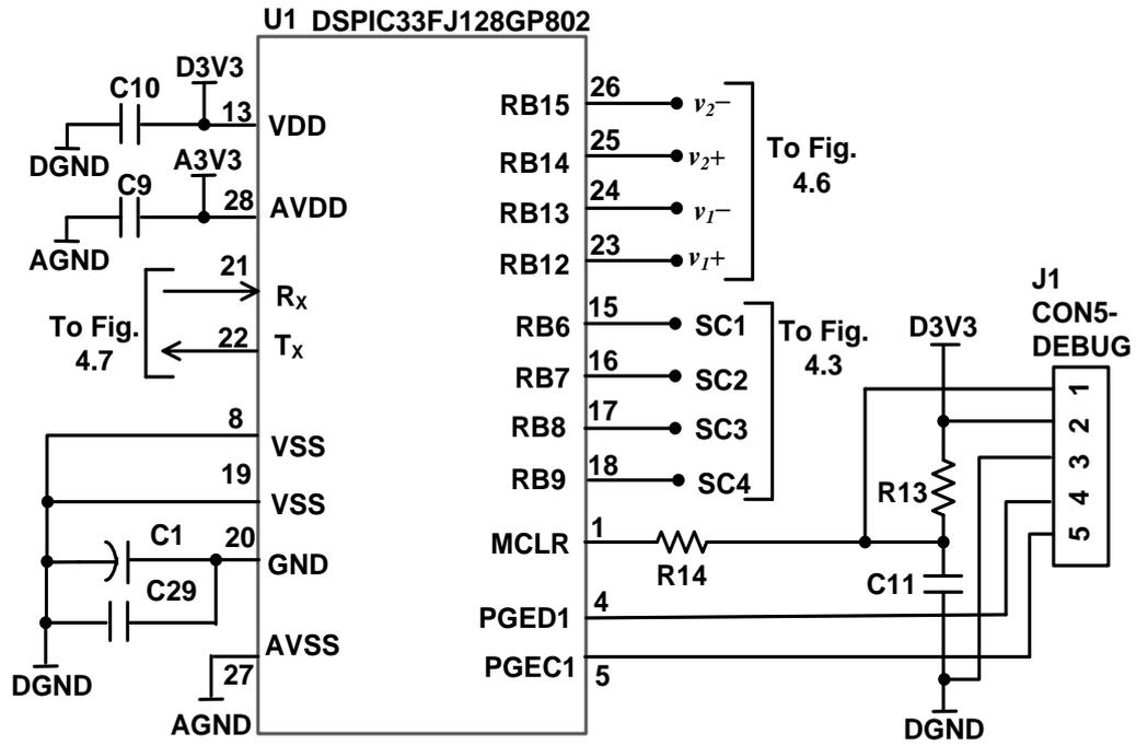
Figure 4.5: Microcontroller connections.
