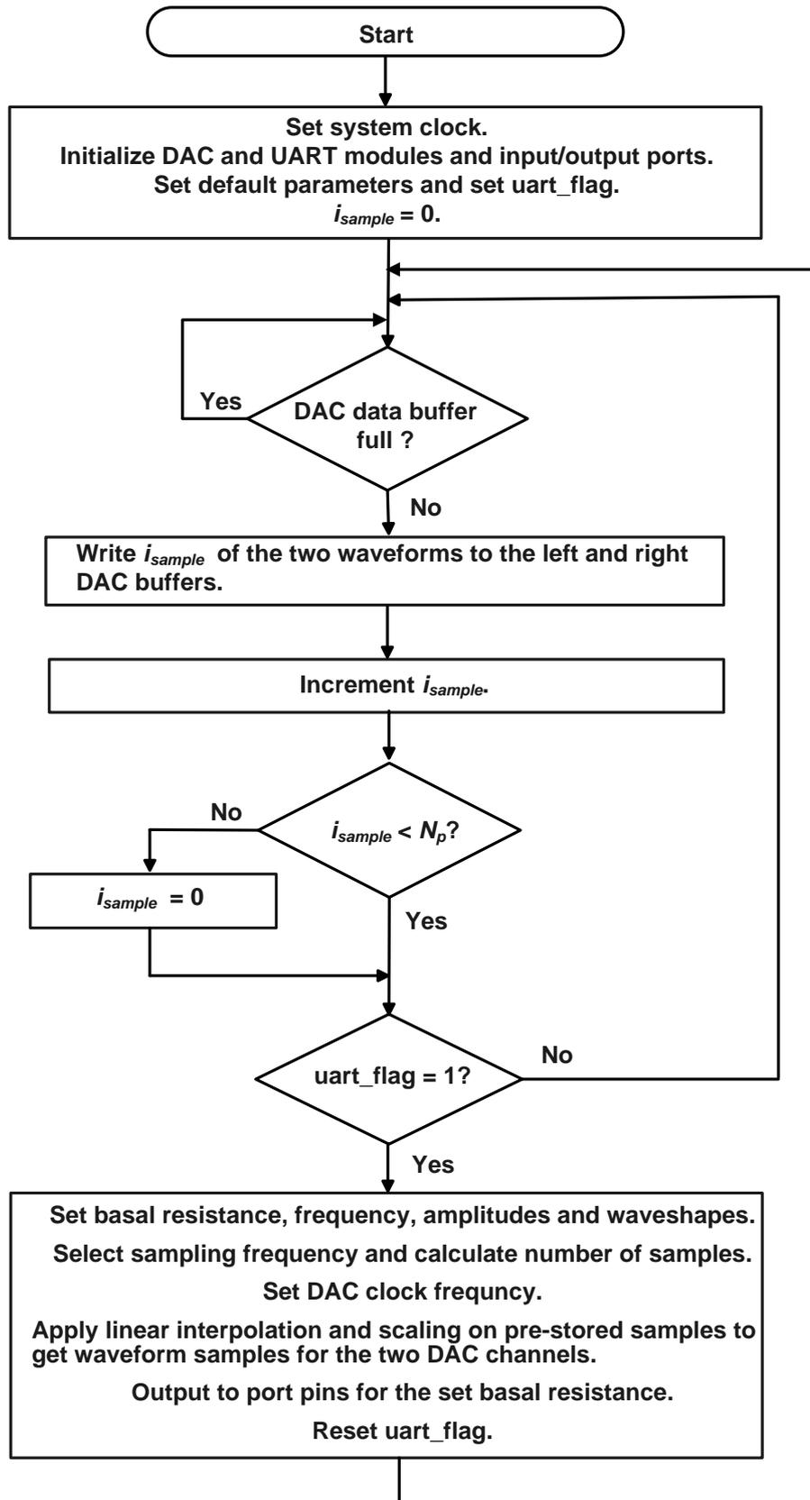
**Figure 4.10:** Flow chart of the main program of “biosim\_control”.
