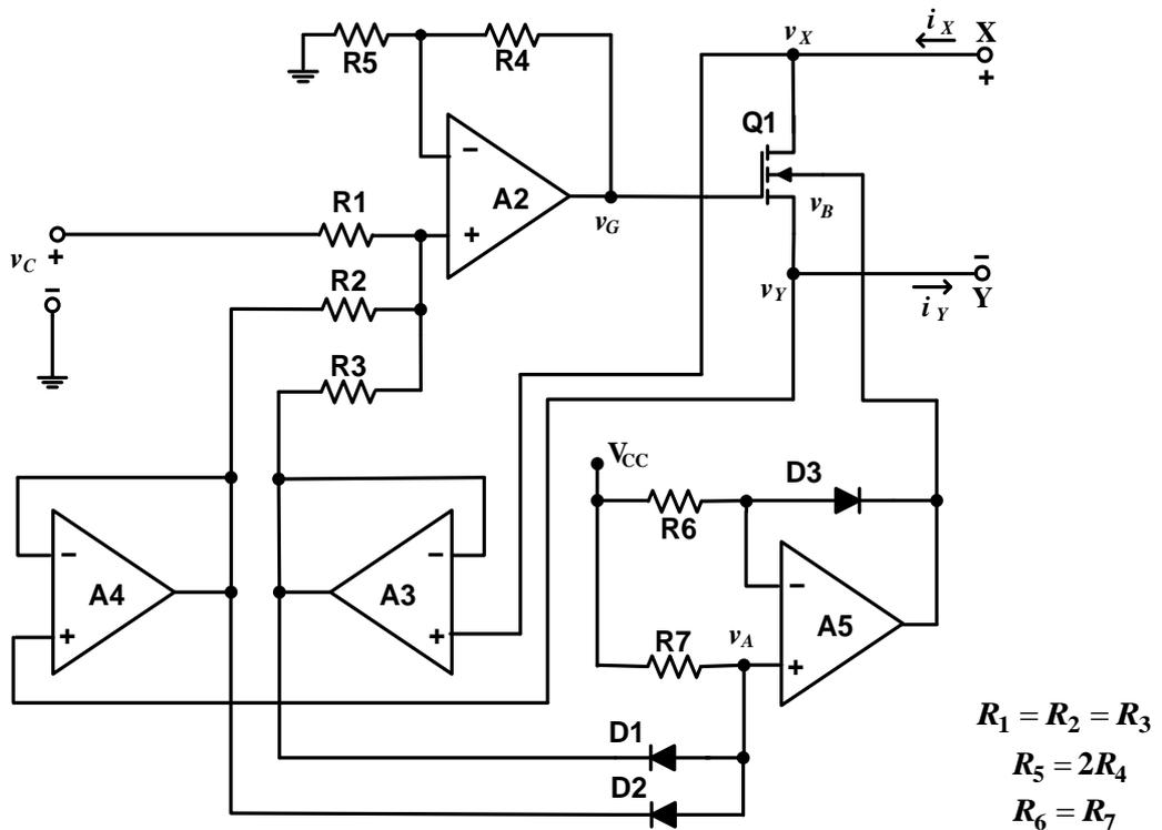
**Figure 3.9:** MOSFET-based floating VCR with SD-bootstrapped gate and S-bootstrapped substrate.
