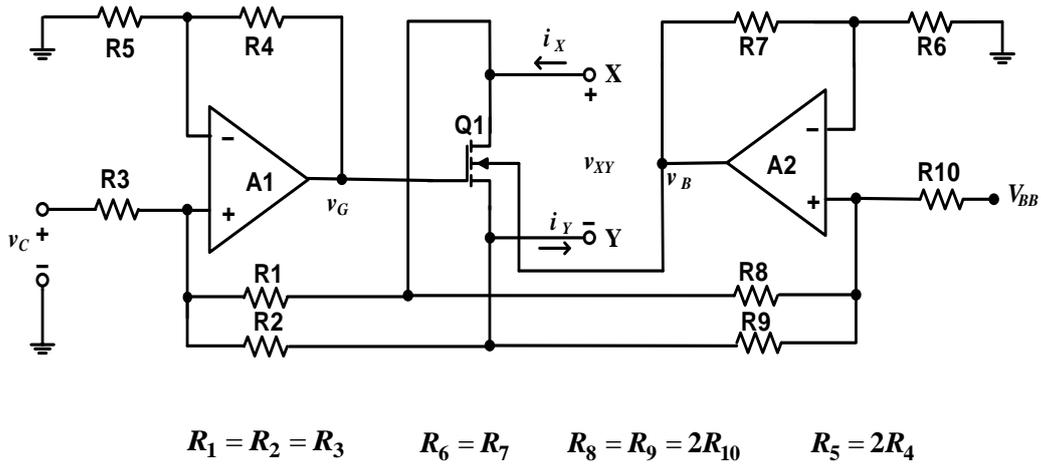
**Figure 3.8:** MOSFET-based floating VCR with SD-bootstrapped gate and SD-bootstrapped substrate.
