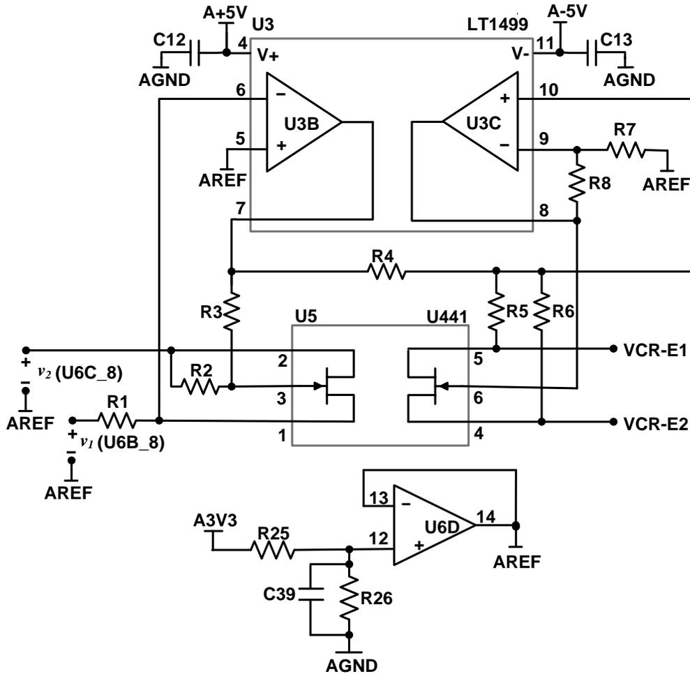
**Figure 4.4:** VCR circuit implemented using U441 and LT1499.
