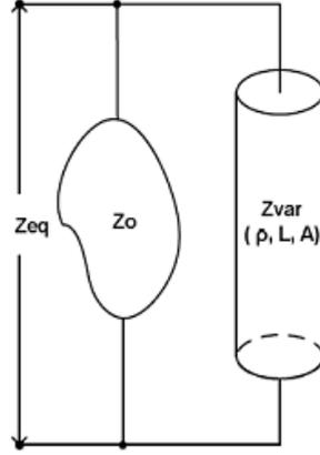
**Figure 2.3:** Parallel-column model [4].
