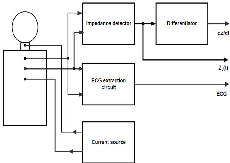
**Figure 2.1:** Block diagram of Impedance Cardiography [8].
