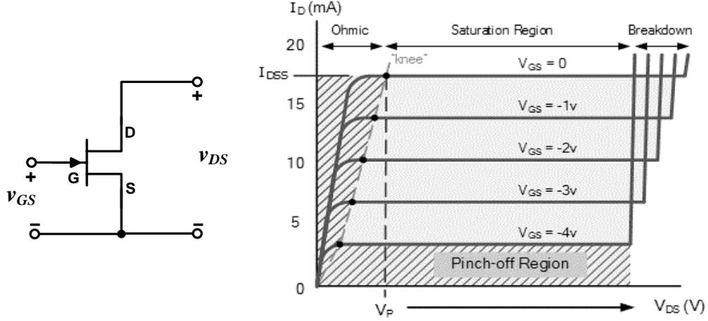
**Figure 3.1:** A n-channel JFET and its drain characteristics (adapted from Figure 14.2 in [17]).
