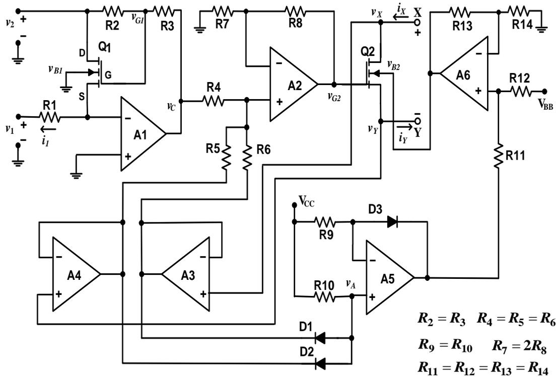
**Figure 3.17:** Matched-pair MOSFET-based floating VCR with self-tracking, SD-bootstrapped-gate, and S-bootstrapped-bias substrate.
