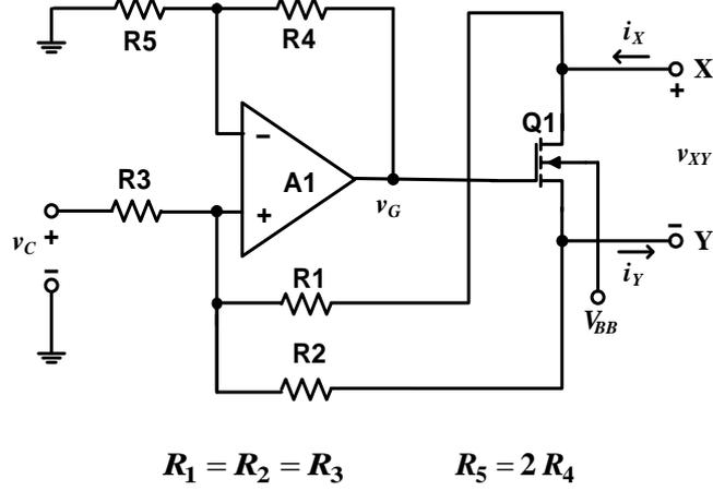
**Figure 3.7:** MOSFET-based floating VCR circuit with SD-bootstrapped gate and fixed-bias substrate.
