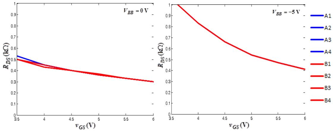
**Figure 3.30:**  $R_{DS}$  versus  $v_{GS}$  curves for four devices on two pieces of ALD1106 for  $V_{BB}$  of 0 and  $-5$  V.
