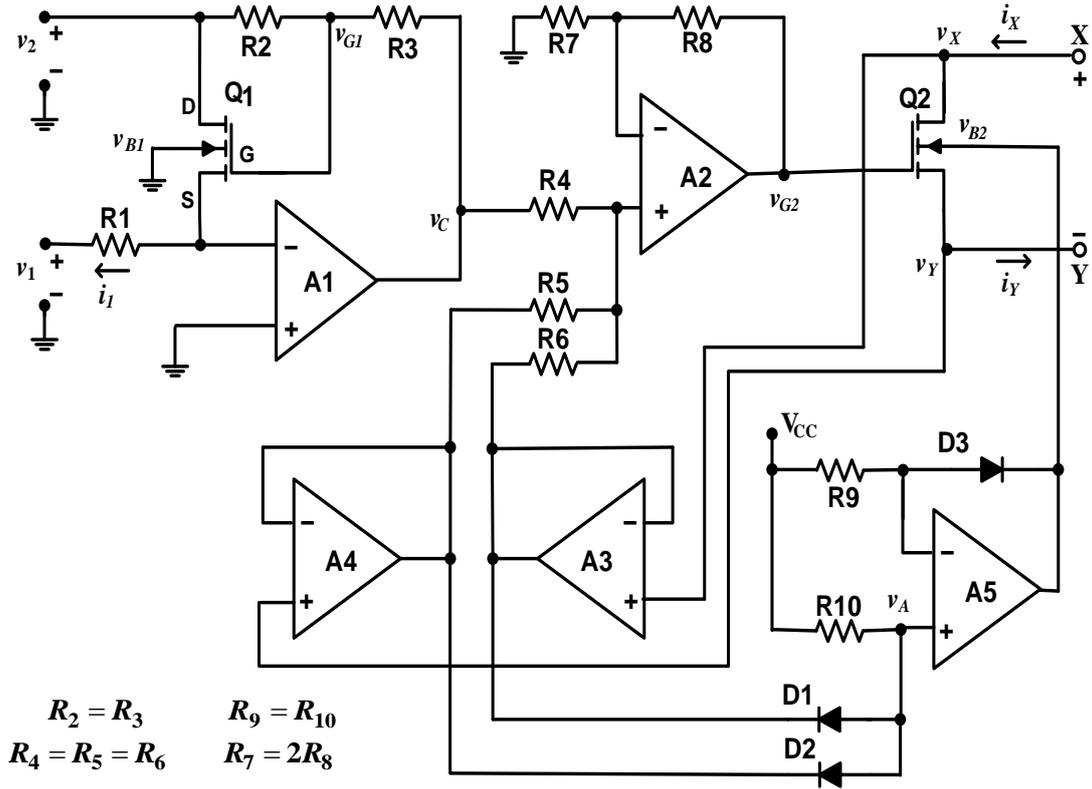
**Figure 3.16:** Matched-pair MOSFET-based floating VCR self-tracking, SD- bootstrapped gate, and S-bootstrapped substrate.
