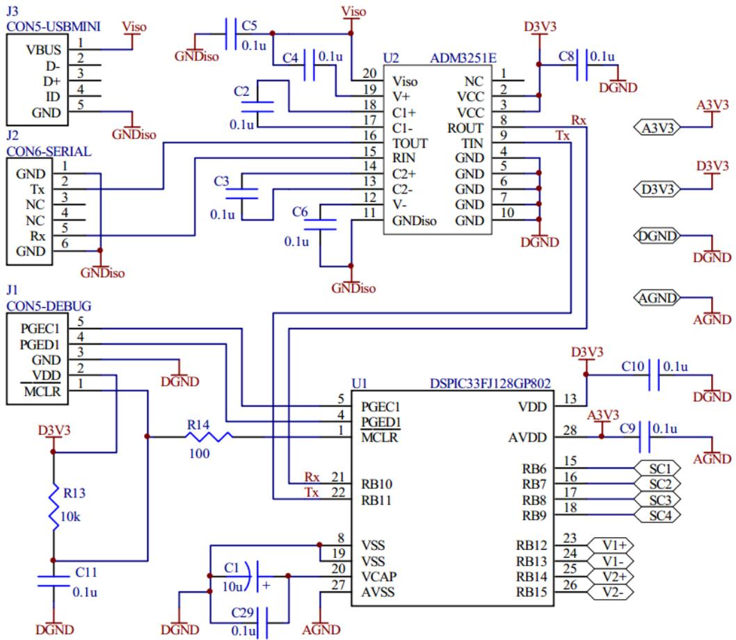
Figure A.2: Controller circuit.
