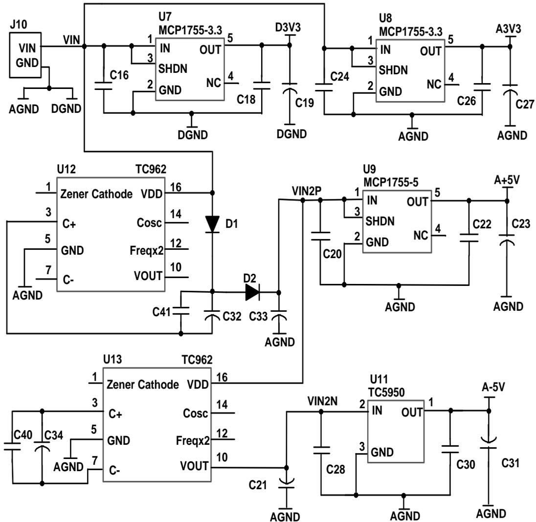
**Figure 4.8:** Power supply circuit.
