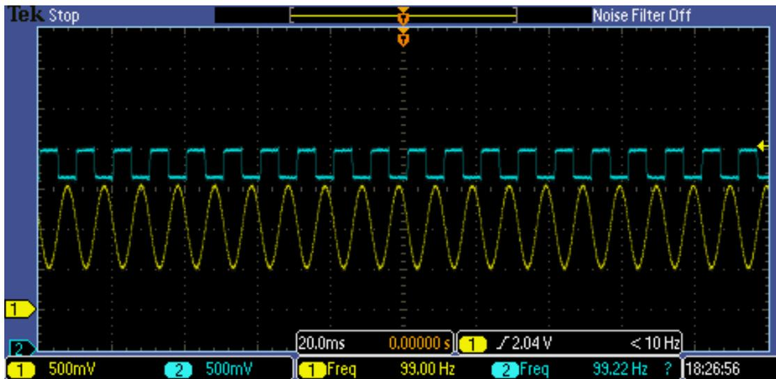
**Figure 5.2:** Output waveforms  $v_1$  (Ch. 1) and  $v_2$  (Ch. 2) for  $f = 100$  Hz,  $v_1$ : 0 V offset and 1 V p-p sine wave,  $v_2$ : 0 V offset and 0.5 V p-p square wave.
