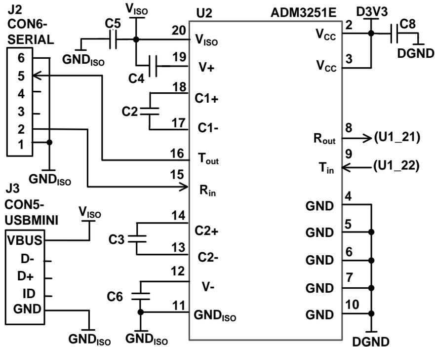
Figure 4.7: Connections of RS232 line driver.
