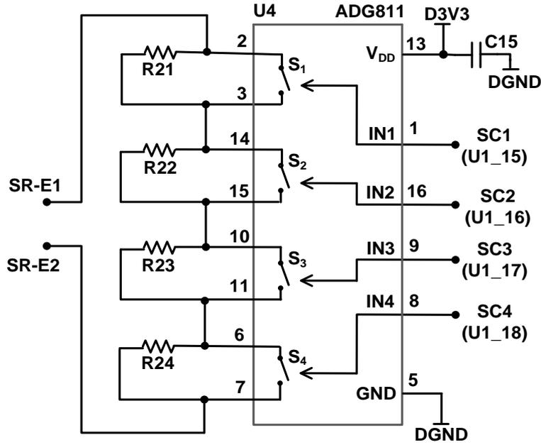
Figure 4.3: Switch-R circuit.
