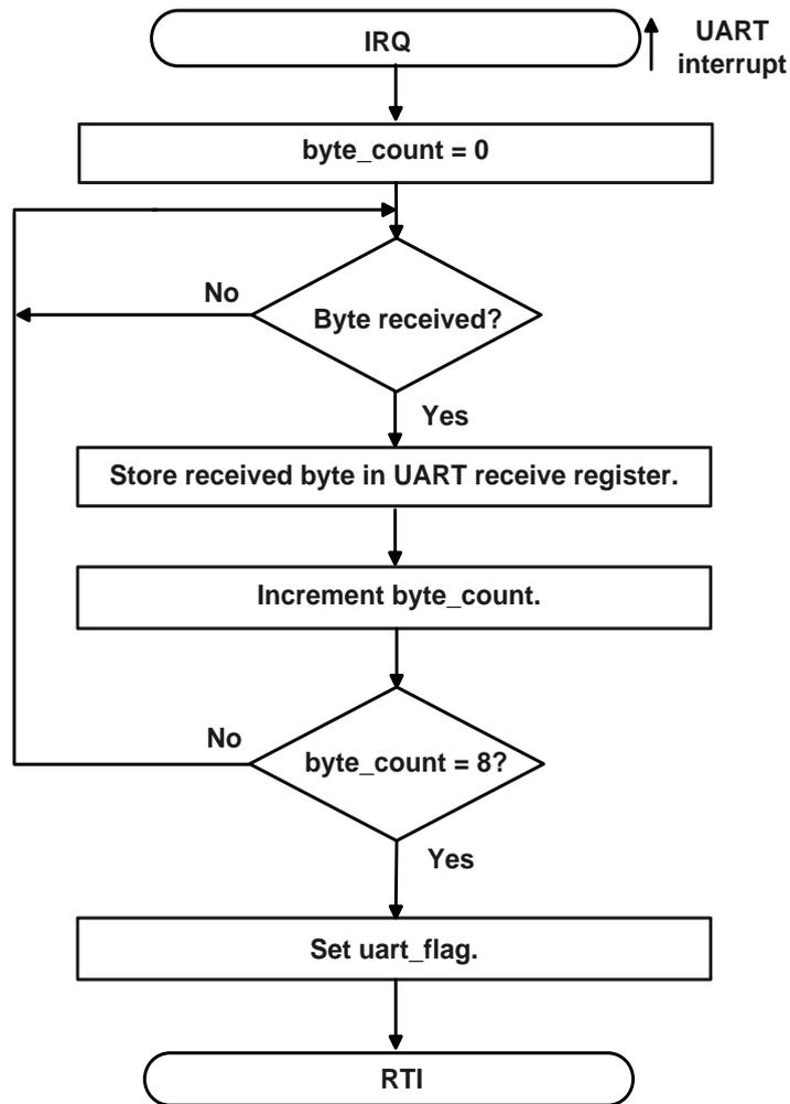
**Figure 4.11:** Flow chart for U1RXInterrupt ISR of biosim\_control.
