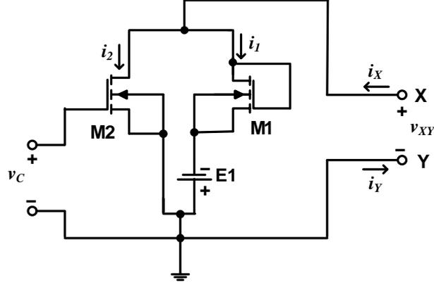
**Figure 3.3:** Enhancement-type MOSFET-based circuit for voltage-controlled linear resistor as proposed by Moon et.al. [24].
