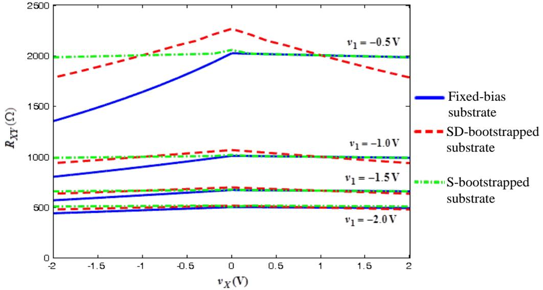
**Figure 3.22:** Simulation results for matched-pair MOSFET-based floating VCR circuits with self-tracking, SD-bootstrapped gate, and different substrate biases: (a) fixed-bias substrate, (b) SD-bootstrapped substrate, and (c) S-bootstrapped substrate.
