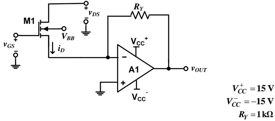
**Figure 3.26:** Current-to-voltage converter for device characteristics of MOSFET.
