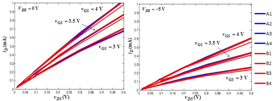
**Figure 3.28:** Drain characteristics of Figure 3.27 for small  $v_{DS}$ .
