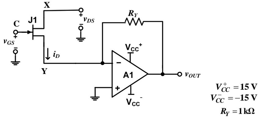
**Figure 3.23:** Current-to-voltage converter for device characteristics of JFET.
