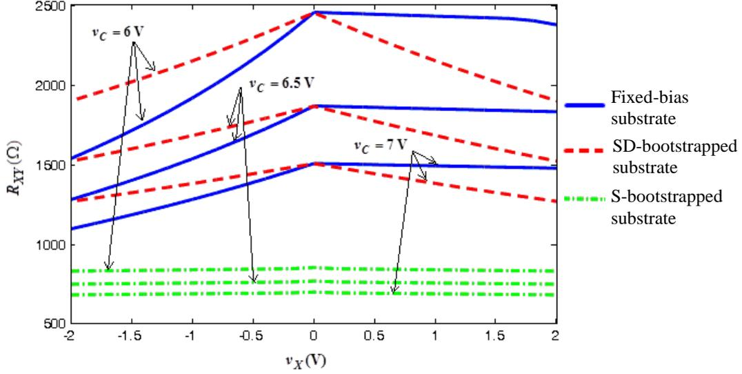
**Figure 3.20:** Simulation results for MOSFET-based floating VCR circuit with SD-bootstrapped-gate and (a) fixed-bias substrate, (b) SD-bootstrapped substrate, and (c) S-bootstrapped substrate.
