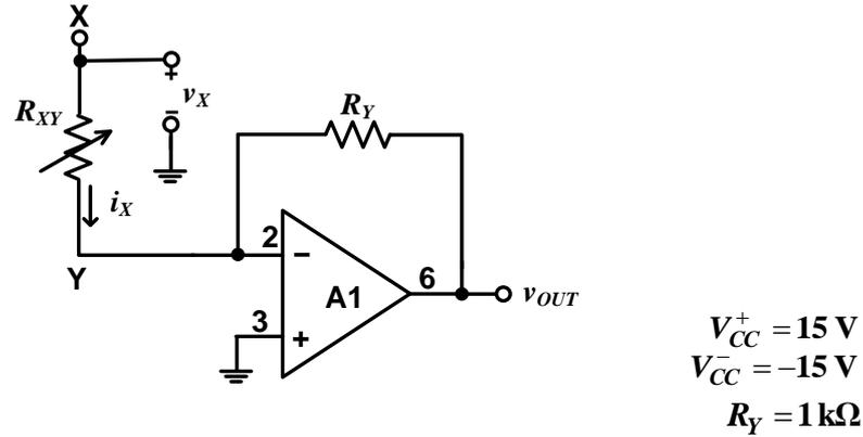
**Figure 3.25:** Current-to-voltage converter for measuring resistance of the VCR circuit.
