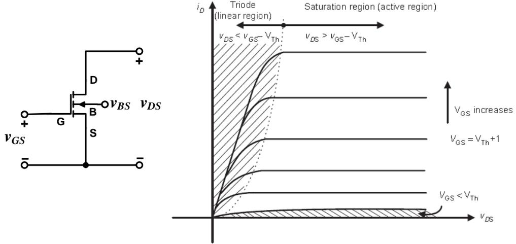
**Figure 3.2:** An enhancement-type NMOS transistor and its drain characteristics (adapted from Figure 4.11 in [19]).
