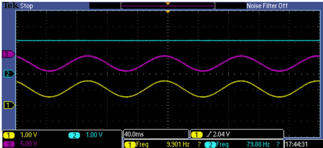
**Figure 5.4:** Output waveforms  $v_1$  (Ch. 1),  $v_2$  (Ch. 2), and  $v_{OUT}$  (Ch. 3) for  $f = 10$  Hz,  $v_X = 0.5$  V,  $v_1$ :  $-0.8$  V offset ( $0.85$  V w.r.t. AGND) and  $1$  V p-p sine,  $v_2$ :  $0.4$  V dc ( $2.05$  V w.r.t. AGND).
