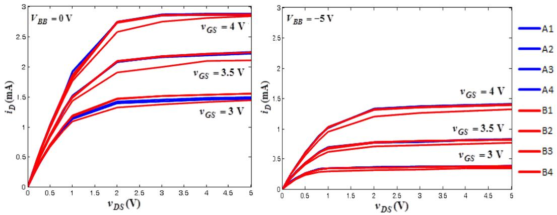
**Figure 3.27:** Drain characteristics of four devices on two pieces of ALD1106 (A, B: two ICs, A1 – A4: 4 devices on IC-A) for  $V_{BB}$  of 0 and  $-5\text{ V}$ .
