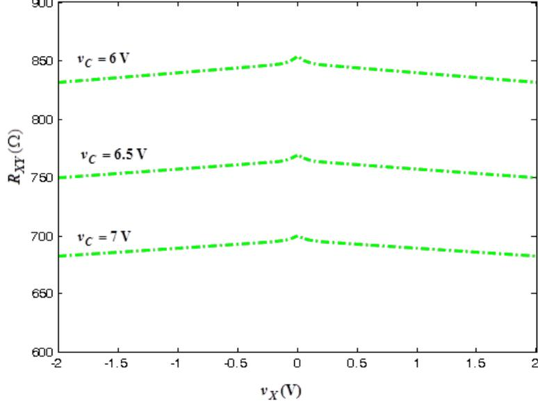
**Figure 3.21:** Simulation results for MOSFET-based floating VCR circuit with SD-bootstrapped gate and S-bootstrapped substrate.
