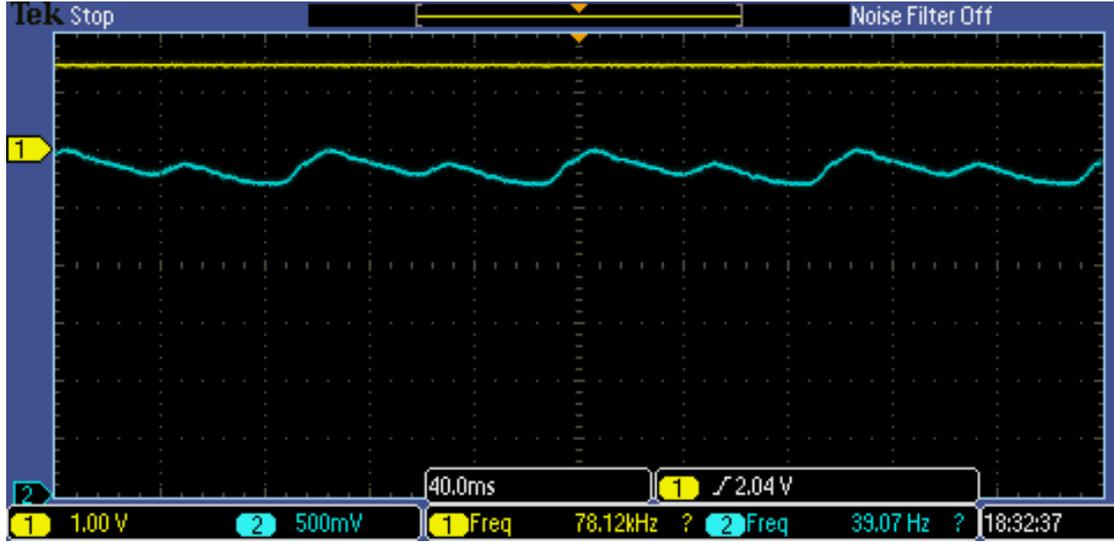
**Figure 5.3:** Output waveforms  $v_1$  (Ch. 1) and  $v_2$  (Ch. 2) for  $f = 10$  Hz,  $v_1$ :  $-0$  V dc,  $v_2$ :  $1$  V offset and  $0.5$  V p-p thoracic wave.
