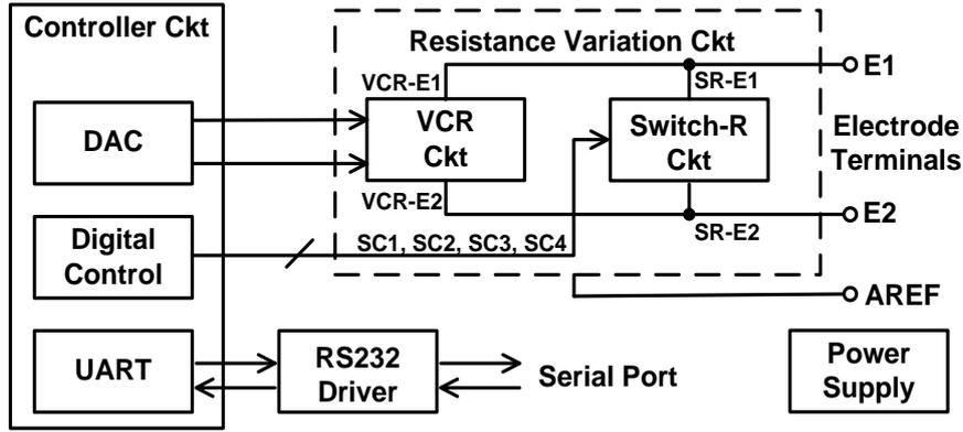
Figure 4.2: Block diagram of bioimpedance simulator.
