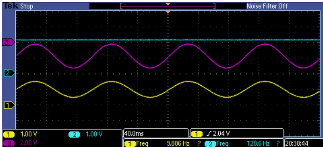
**Figure 5.5:** Output waveforms  $v_1$  (Ch. 1),  $v_2$  (Ch. 2), and  $v_{OUT}$  (Ch. 3) for  $f = 10$  Hz,  $v_X = 0.3$  V,  $v_1$ :  $-0.8$  V offset ( $0.85$  V w.r.t. AGND) and  $1$  V p-p sine,  $v_2$ :  $0.4$  V dc ( $2.05$  V w.r.t. AGND).
