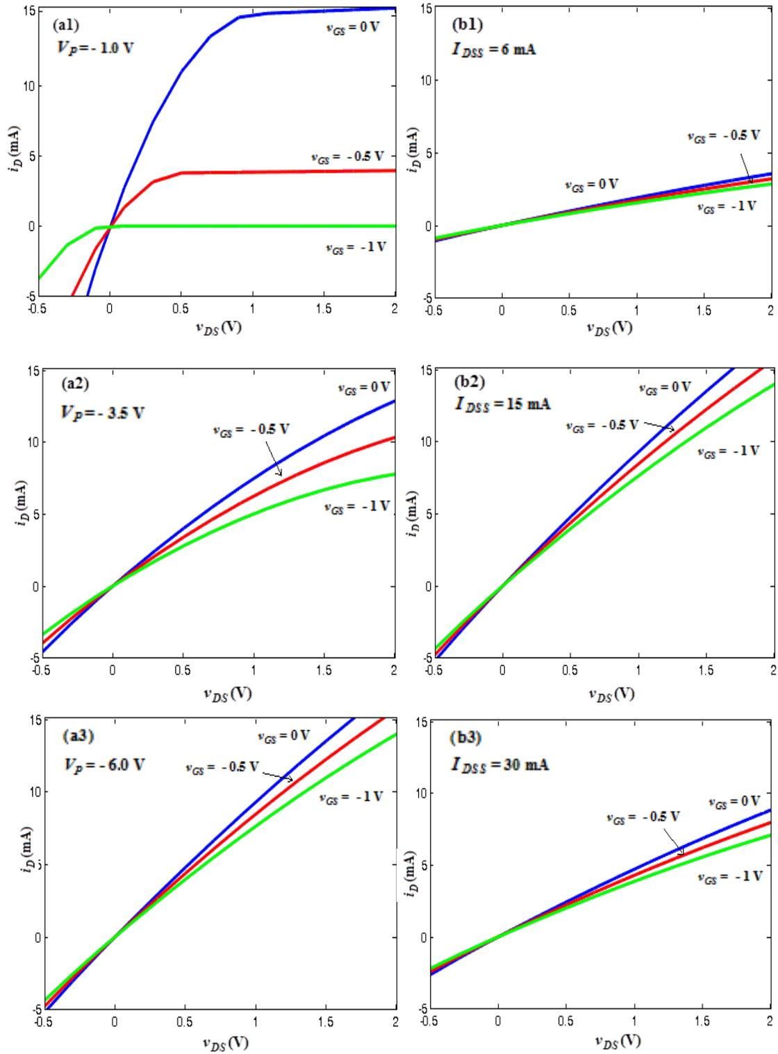
**Figure 3.18:** Drain characteristics of JFET on U441, obtained using the simulator LTspice IV for (a)  $I_{DSS} = 15$  mA and three values of  $V_P$ ; (b)  $V_P = -6$  V and three values of  $I_{DSS}$ .
