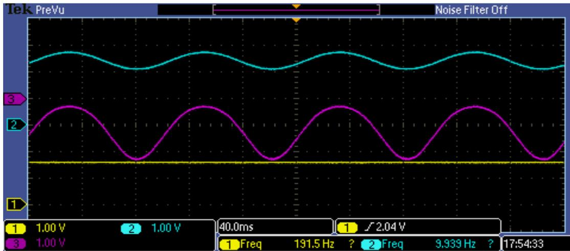
**Figure 5.6:** Waveforms  $v_1$  (Ch. 1),  $v_2$  (Ch. 2), and  $v_{OUT}$  (Ch. 3) for  $f = 10$  Hz.  $v_1$ :  $-0.1$  V dc (1.55 V w.r.t. AGND),  $v_2$ : 0.4 V offset (2.05 V w.r.t. AGND) and 0.4 V p-p sine.
