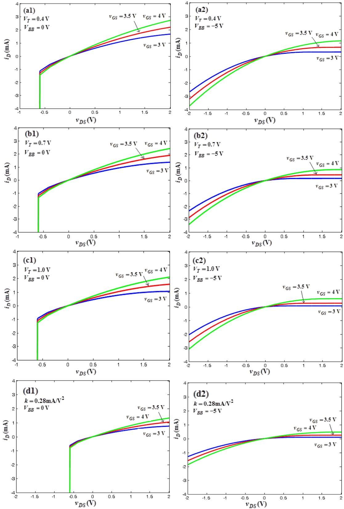
**Figure 3.19:** Drain characteristics of MOSFET on ALD1106, obtained using the simulator LTspice IV for (a), (b), and (c):  $k = 0.52$  mA/V<sup>2</sup> and different values of  $V_T$  (d)  $V_T = 0.7$  V and different values of  $k = 0.28$  mA/V<sup>2</sup>.
