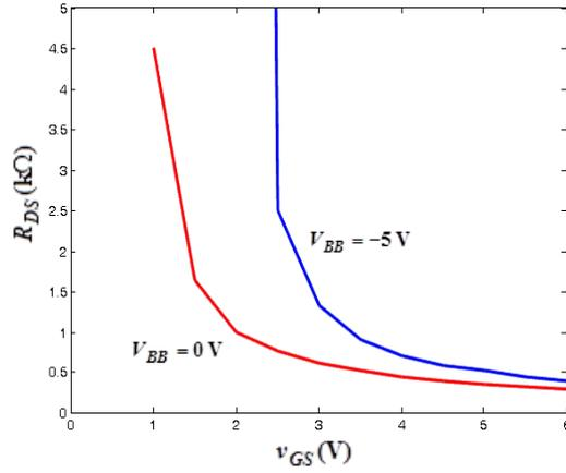
**Figure 3.29:**  $R_{DS}$  versus  $v_{GS}$  curve for one of the devices on ALD1106 for  $V_{BB}$  of 0 and  $-5$  V.
