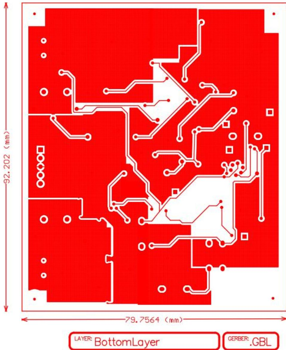
**Figure B.3:** Bottom layer of PCB.
