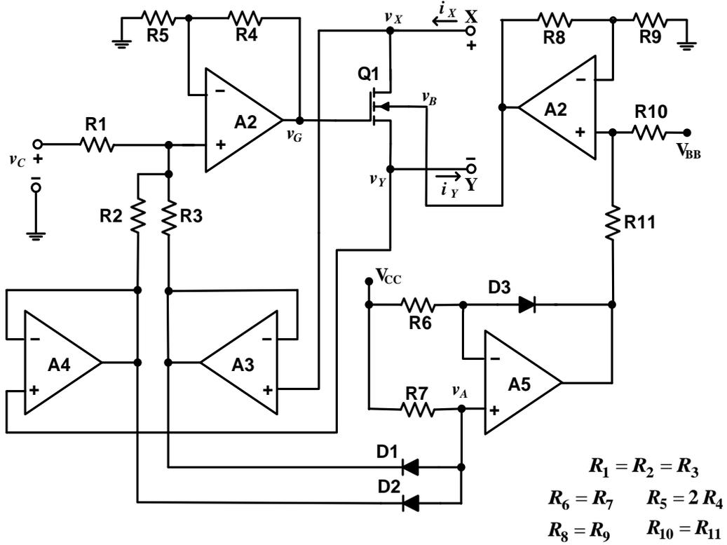
**Figure 3.10:** MOSFET-based floating VCR with SD-bootstrapped gate and S-bootstrapped-bias substrate.
