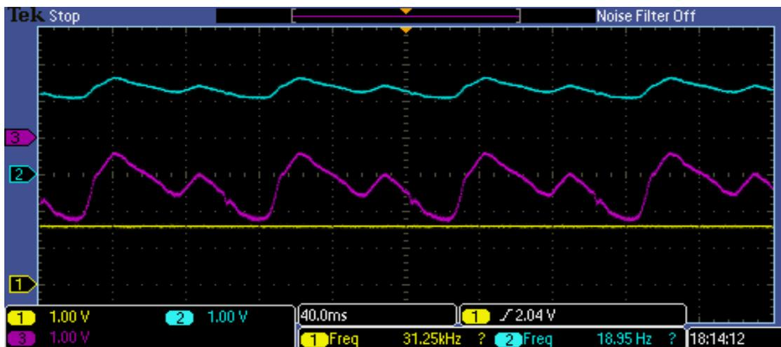
**Figure 5.7:** Waveforms  $v_1$  (Ch. 1),  $v_2$  (Ch. 2), and  $v_{OUT}$  (Ch. 3) for  $f = 10$  Hz.  $v_1$ :  $-0.1$  V dc (1.55 V w.r.t. AGND),  $v_2$ : 0.4 V offset (2.05 V w.r.t. AGND) and 0.4 V p-p thoracic wave.
