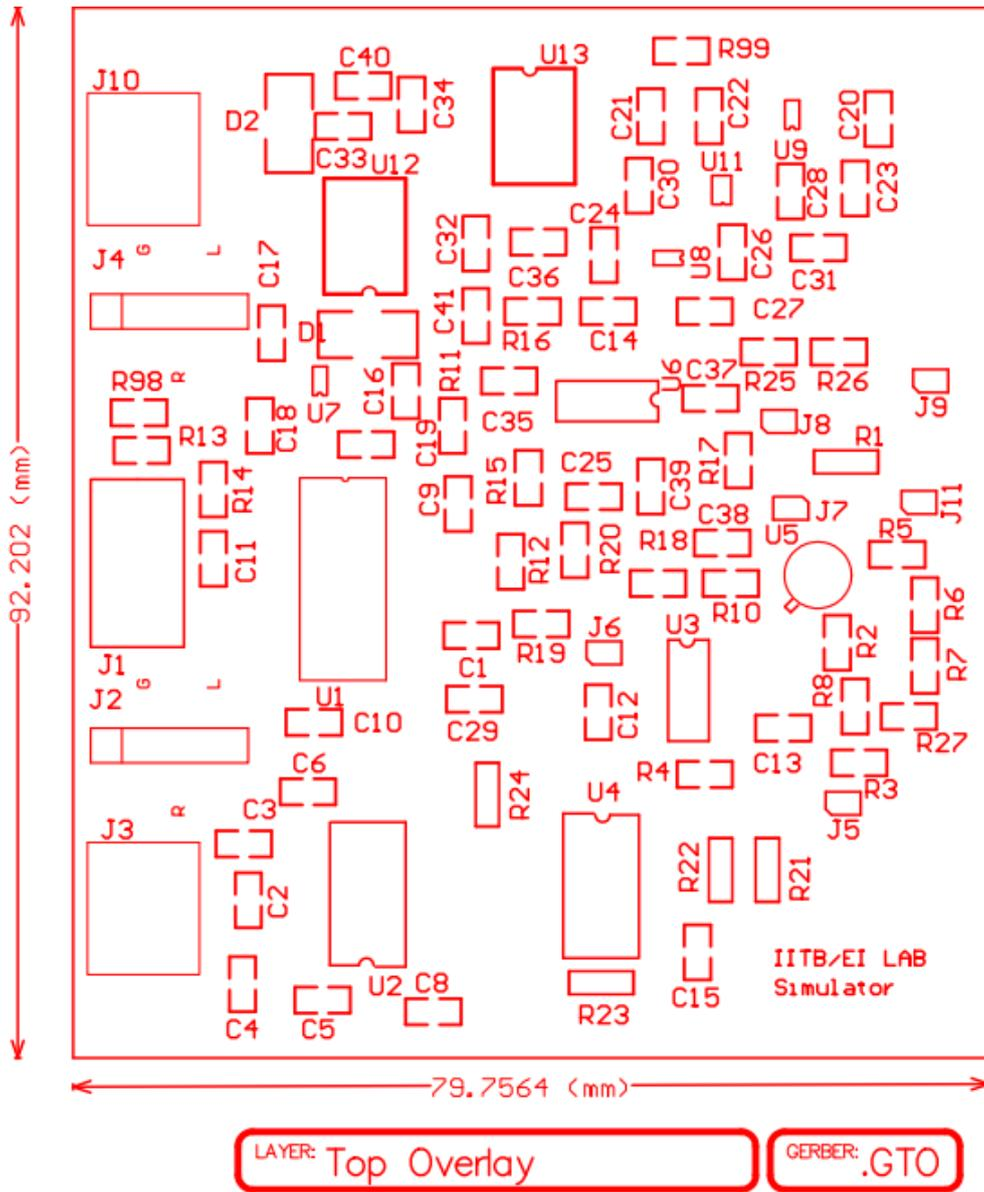
Figure B.1: Top overlay of PCB.
