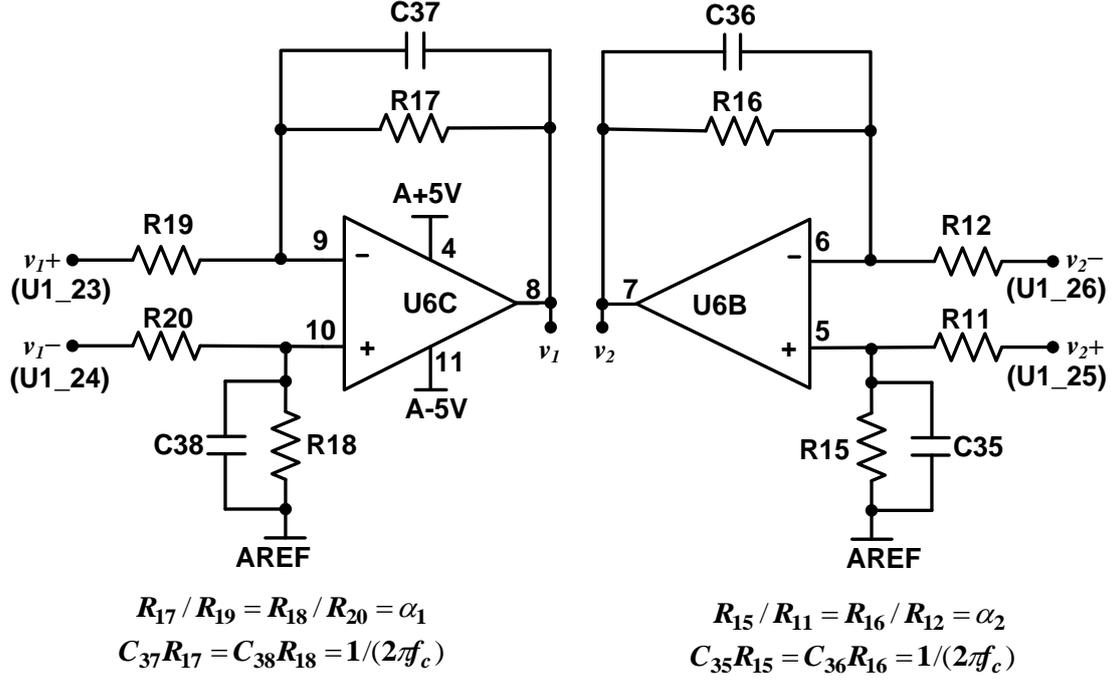
**Figure 4.6:** Differential amplifiers for generating  $v_1$  and  $v_2$  from the two DAC channels of the microcontroller U1.
