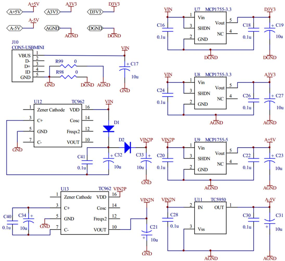
**Figure A.1:** Power supply circuit.
