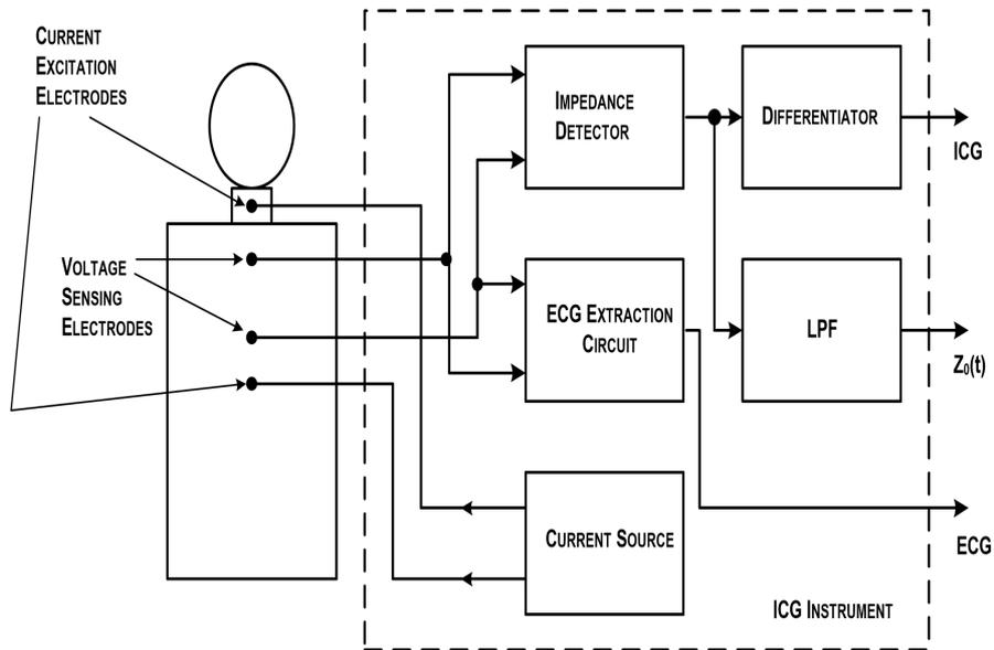
Figure 2.3: Block diagram for impedance cardiography
