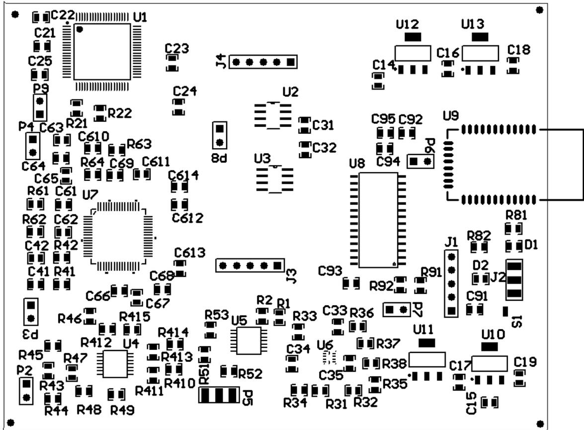
Figure. B.1: Top overlay of the assembled PCB.
