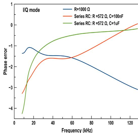
Figure 4.4: Relative error in phase for I/Q
