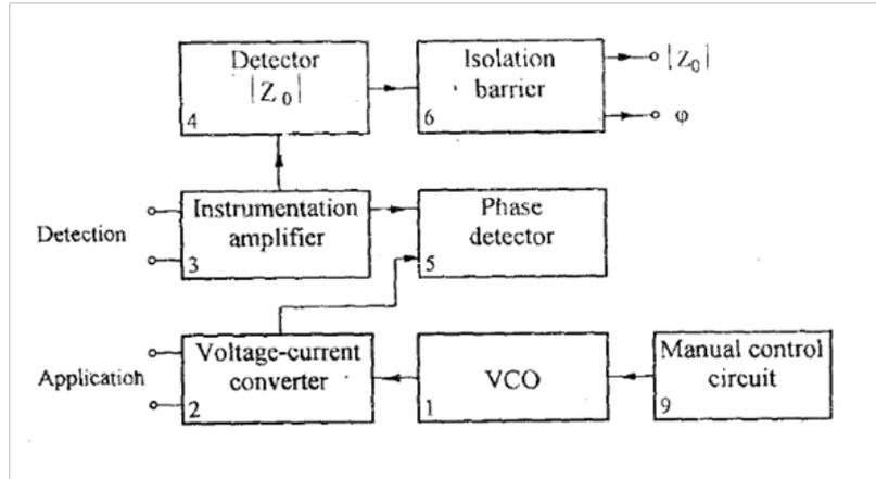
Figure 2.6: Block diagram of bio-impedance monitor as reported by Palko et al. [15]
