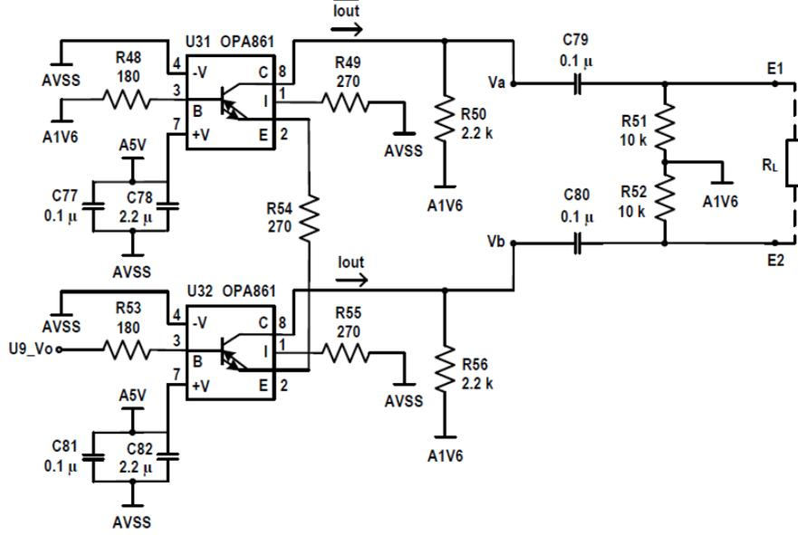
Figure 2.12: V/I converter using trans-conductance amplifier [24]
