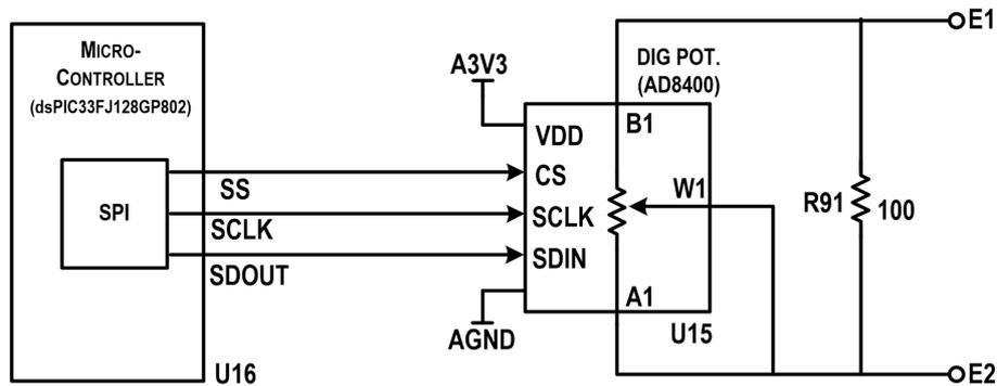
Figure 4.7: Test setup for generating impedance variations.
