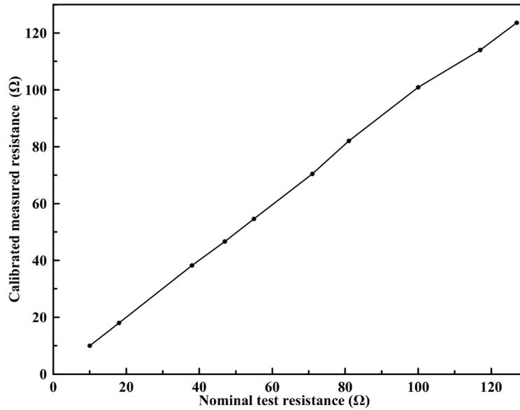
Figure 4.1: Plot of the measured value using the chip vs the resistance value measured using a multimeter.
