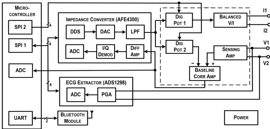
Figure 3.2: Block level schematic of the impedance cardiograph.
