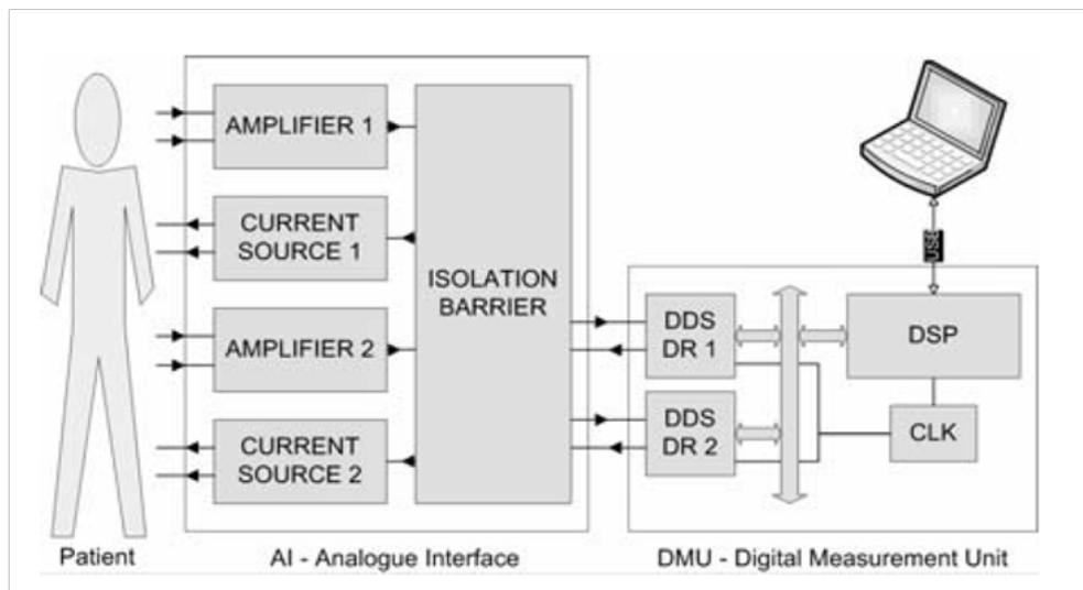
Figure 2.7: Block diagram of two channel bio-impedance monitor reported by Vondra et al. [16]
