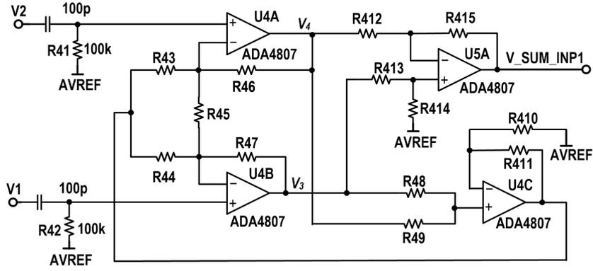
Figure 3.9: Voltage sensing amplifier
