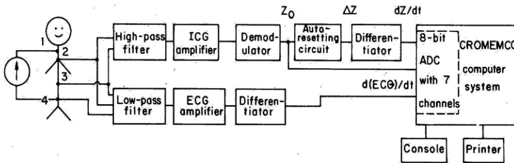
Figure 2.5: Block diagram of the ICG system as developed by Qu et al. [6]
