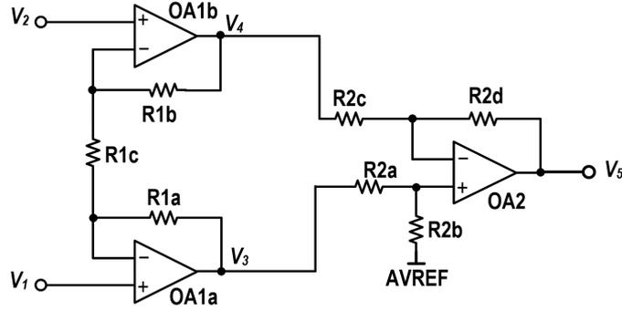
Figure 3.7: Two-stage instrumentation amplifier
