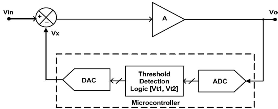
Figure 2.15: Tracking based baseline correction [31]
