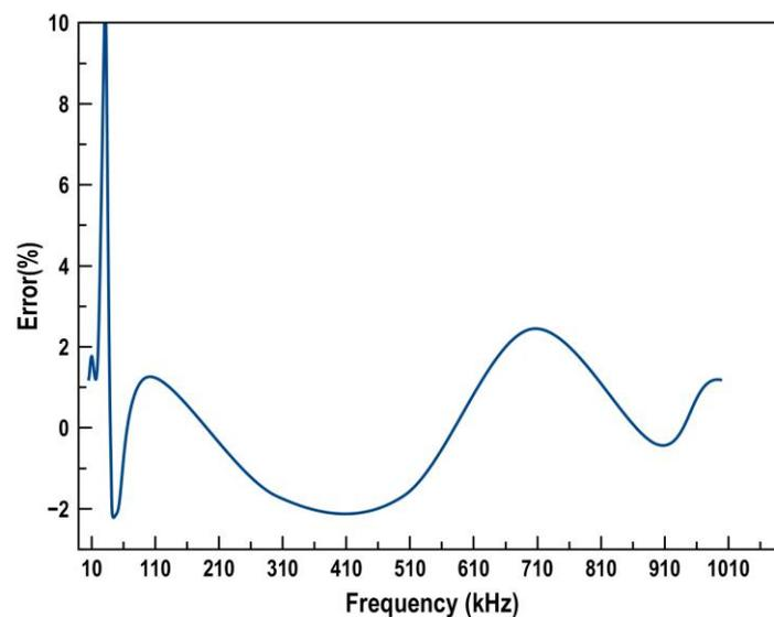
Figure 4.6: Relative error in magnitude for I/Q mode at different interfering frequencies
