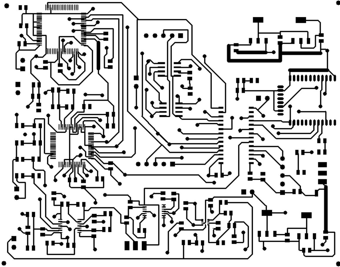
Figure. B.2: Top layer of the assembled PCB.
