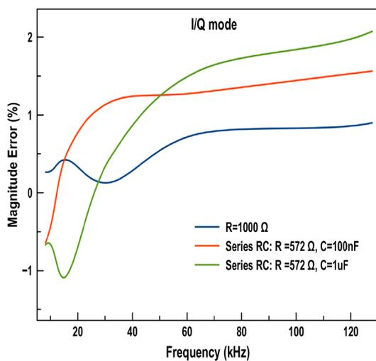
Figure 4.3: Relative error in magnitude for I/Q mode
