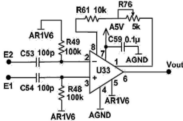
Figure 2.13: Voltage sensing amplifier using INA155 [24]
