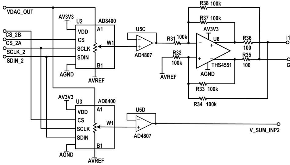
Figure 3.6: Amplitude control using digital potentiometers and op amp based balanced current source.
