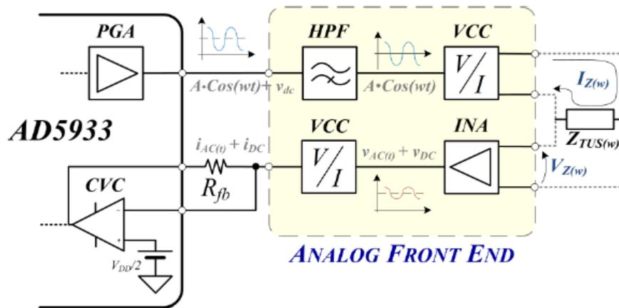
Figure 2.8: Block diagram of Analog front end (AFE) [19]
