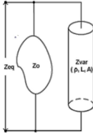
Figure 2.2: Parallel column model for thorax [5]
