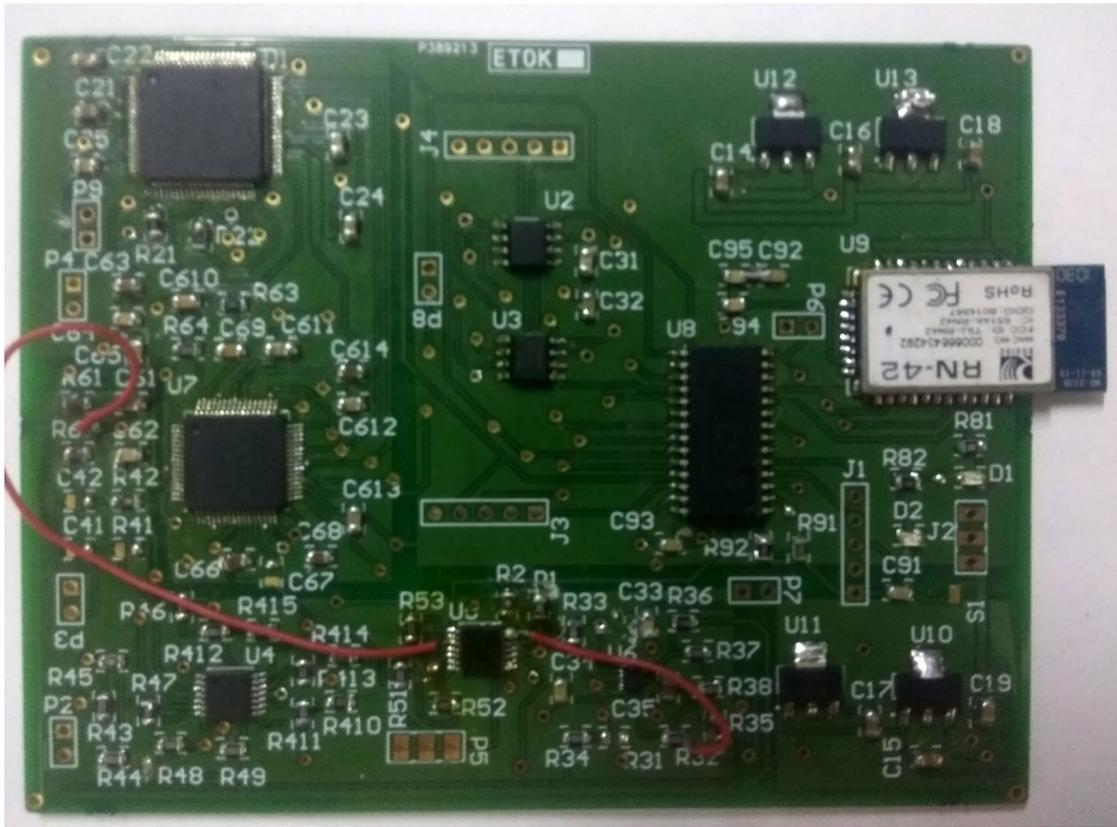
Figure. B.4: Top view of the assembled PCB.
