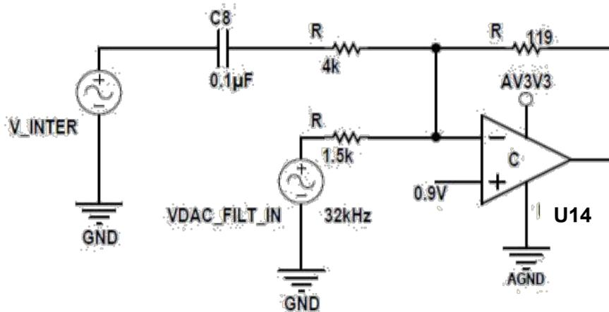
Figure 4.5: Noise rejection testing circuit
