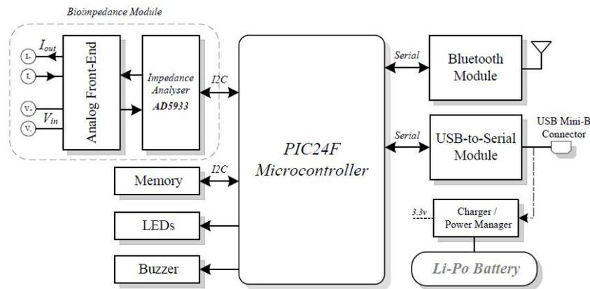
Figure 2.9: Functional block diagram of portable bio-impedance monitor as reported by Ferreira et al. [19]
