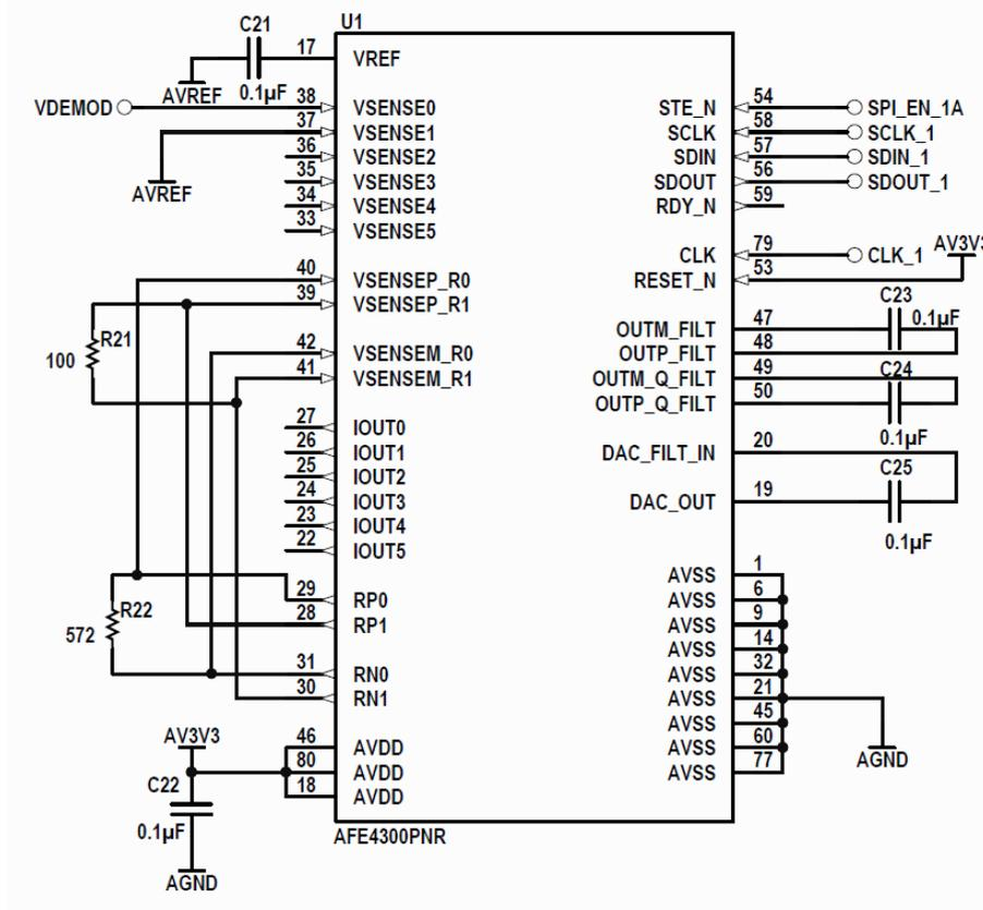
Figure. 3.4: Impedance converter IC AFE4300 connections
