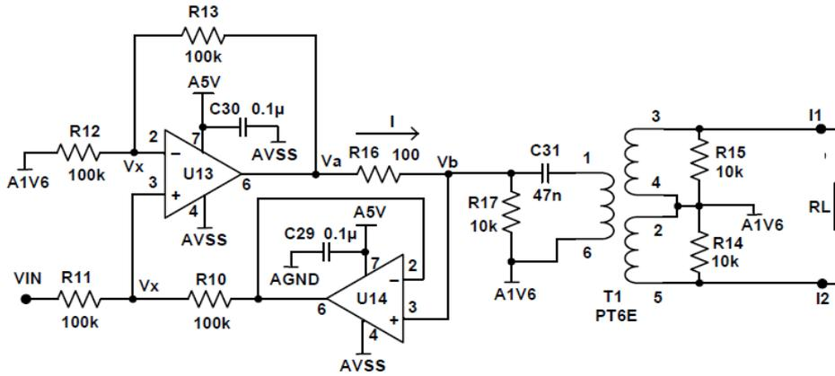
Figure 2.11: Modified Howland current source with centre tapped pulse transformer [24]
