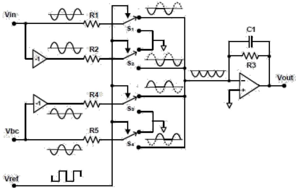
Figure 2.14: Synchronous demodulation using current steering with base line correction [24]
