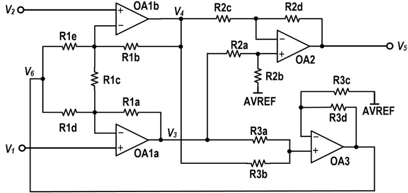
Figure 3.8: Voltage sensing amplifier with common-mode feedback
