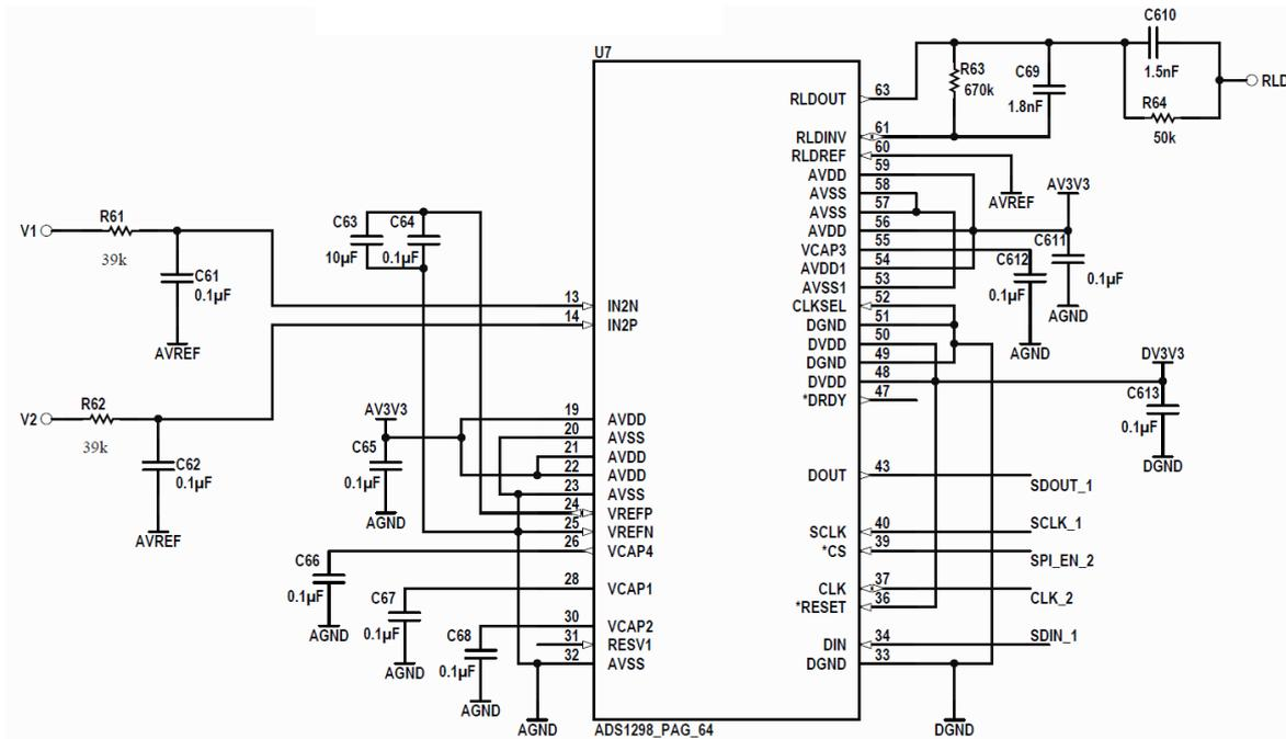
Figure 3.11: ECG extractor using ADS1298 connections
