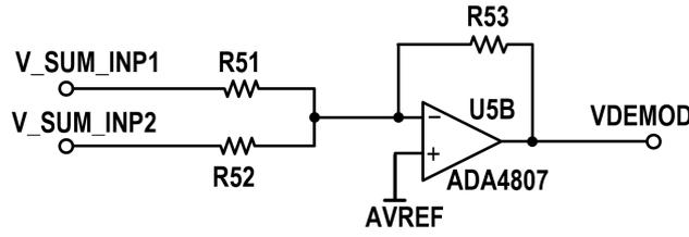
Figure 3.10: Summing amplifier for baseline correction
