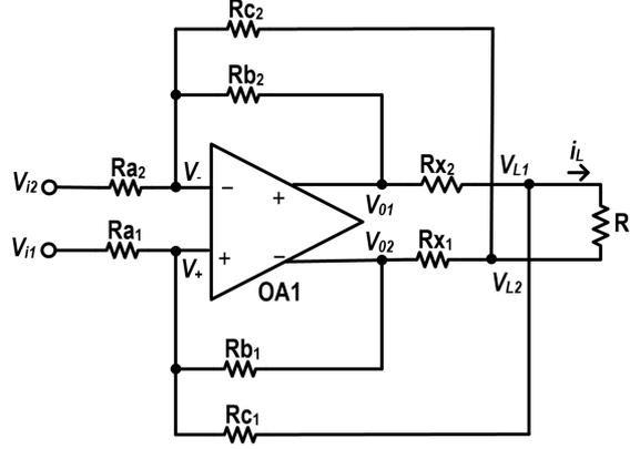
Figure 3.5: Balanced V/I converter using a BTL amplifier
