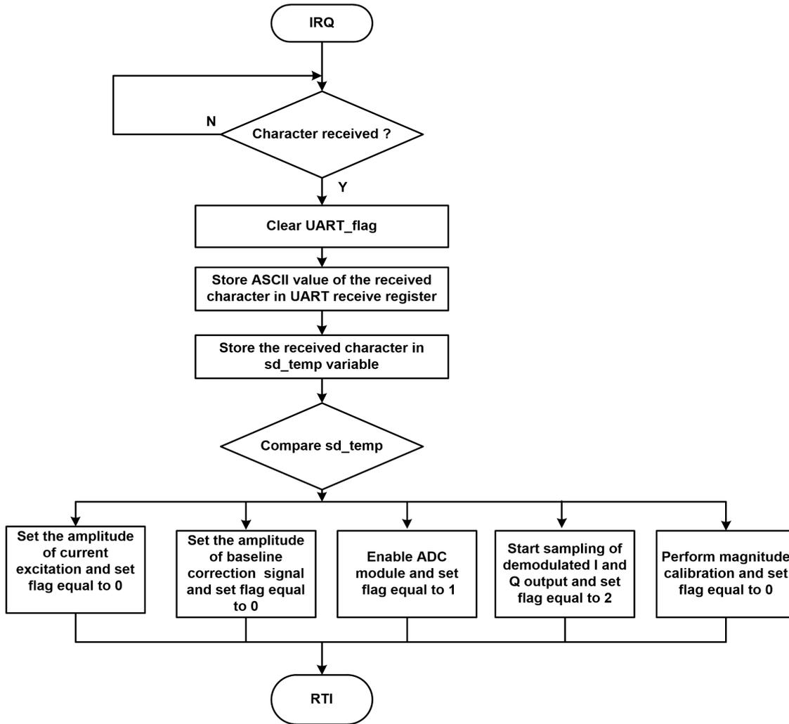
Figure 3.16: Flowchart of UIRX interrupt ISR
