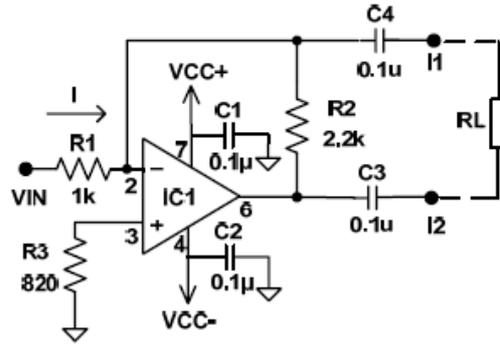
Figure 2.10: V/I converter with the load connected in feedback [25]
