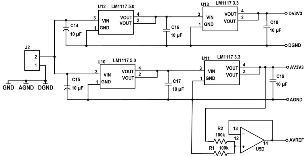
Figure 3.14: Power circuit
