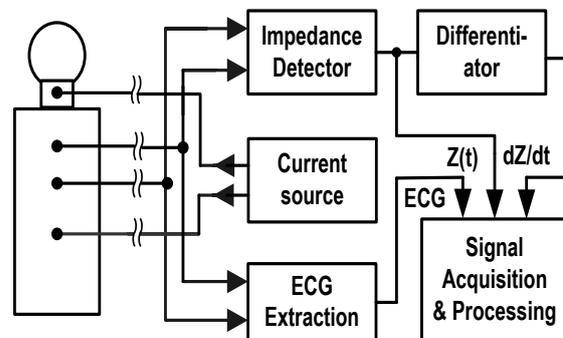
Fig. 1 Block diagram of instrumentation for impedance cardiograph
