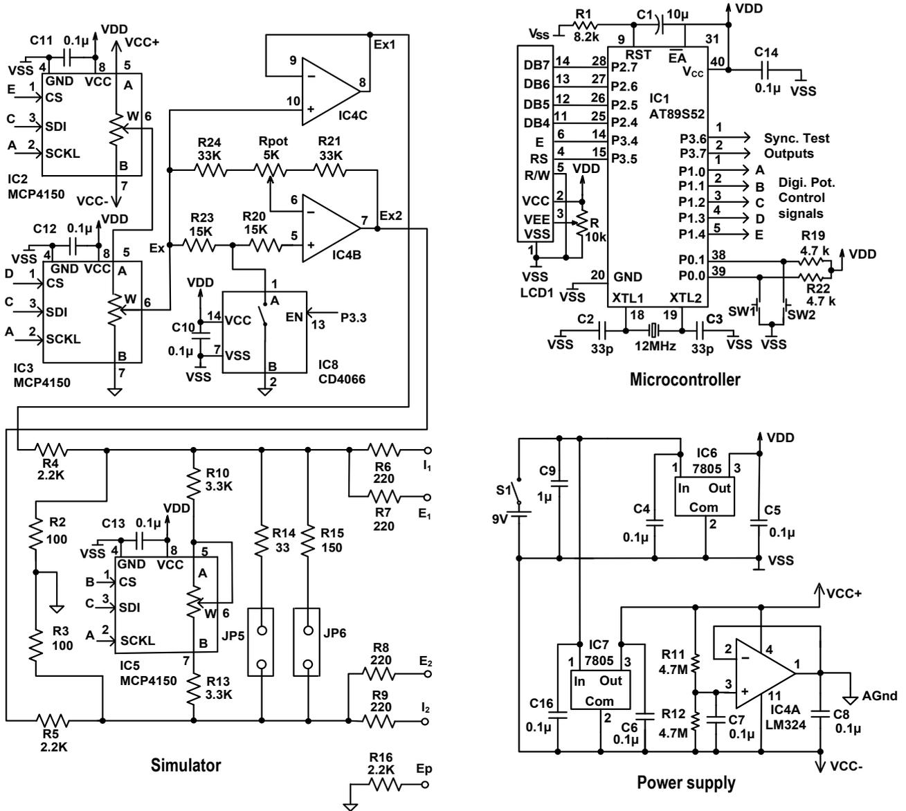
Fig.5 Thorax simulator for testing of the bioimpedance detector
