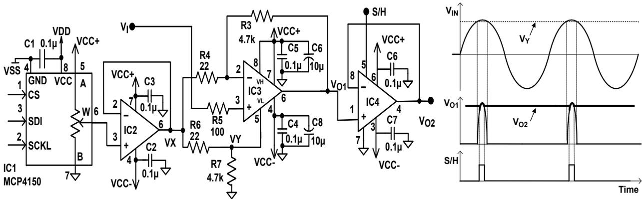
Fig. 2 Demodulator using slicing amplifier and sample-and-hold circuit (IC1: MCP4150, IC2: LF356, and IC3: AD8037, IC4: HA5351) and the output of the slicing amplifier.
