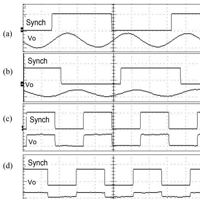
Fig. 6 Waveforms from measurements on the thorax simulator. Upper trace: synchronization test output of simulator, Lower trace: output of the impedance detector (excitation frequency = 100 kHz and current = approx. 1 mA) for  $f = 8$  Hz,  $R = 196 \Omega$  and resistance variations of (a) 1.2 % sinusoidal, (b) 0.6 % sinusoidal, (c) 1.2 % square, (d) 0.6 % square. Time scale: 40 ms/div, Ch1 scale: 5 V/div, Ch2 scale: 500 mV/div.
