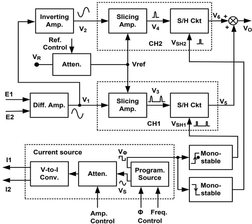
Fig. 3 Bioimpedance detector with two channel slicing amplifier and sample-and-hold circuit
