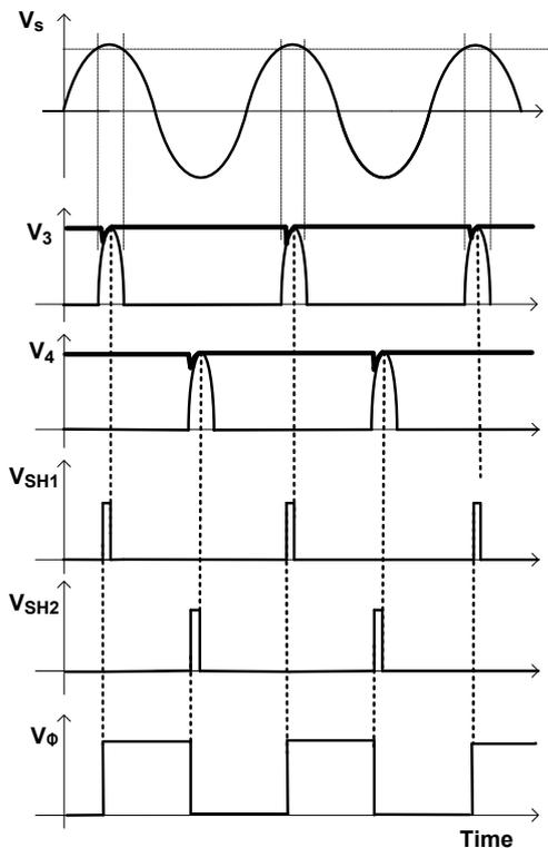
Fig. 4 Waveforms in the bioimpedance detector circuit of Fig. 3.
