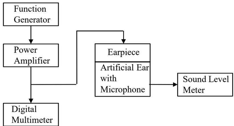
FIG. D.1 Experimental set-up for measuring the electroacoustic response of headphone TDH-39P
