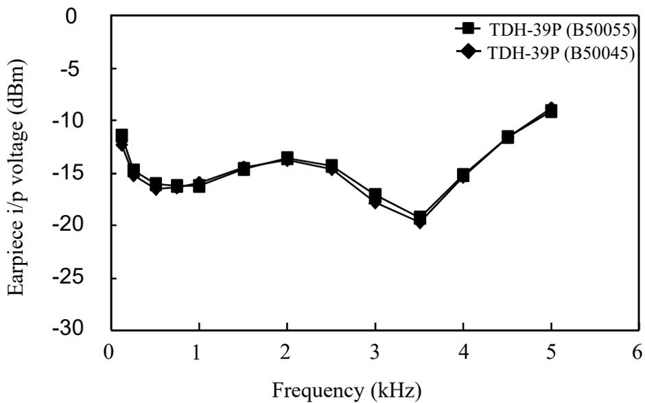
FIG. D.2 Earpiece input voltage versus frequency for 100 dB SPL at earpiece output. The earpiece input voltage was measured in dBm with  $V_{ref} = 224$  mV (corresponding to 1 mW power in 50 ohm load resistance)
