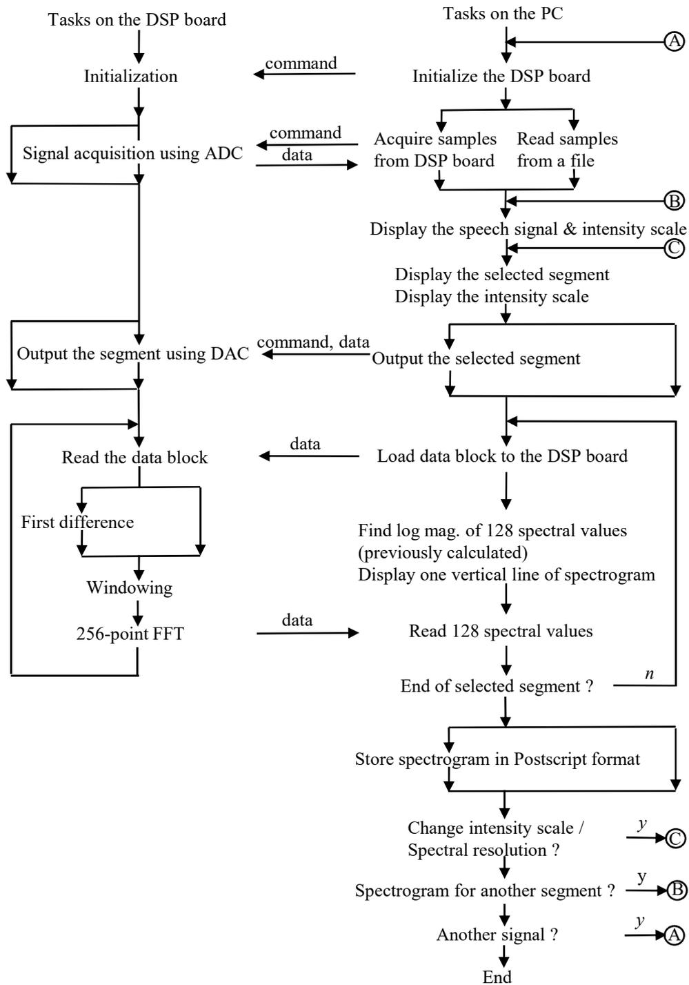
FIG. A. 1 Flowchart of task allocation, between the DSP board and the PC for spectrographic analyzer
