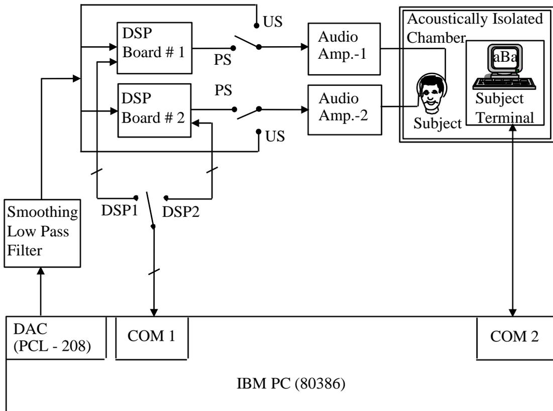
FIG. 5.8 Experimental set-up for the computerized test administration of listening tests for the evaluation of real-time processing implementation.
