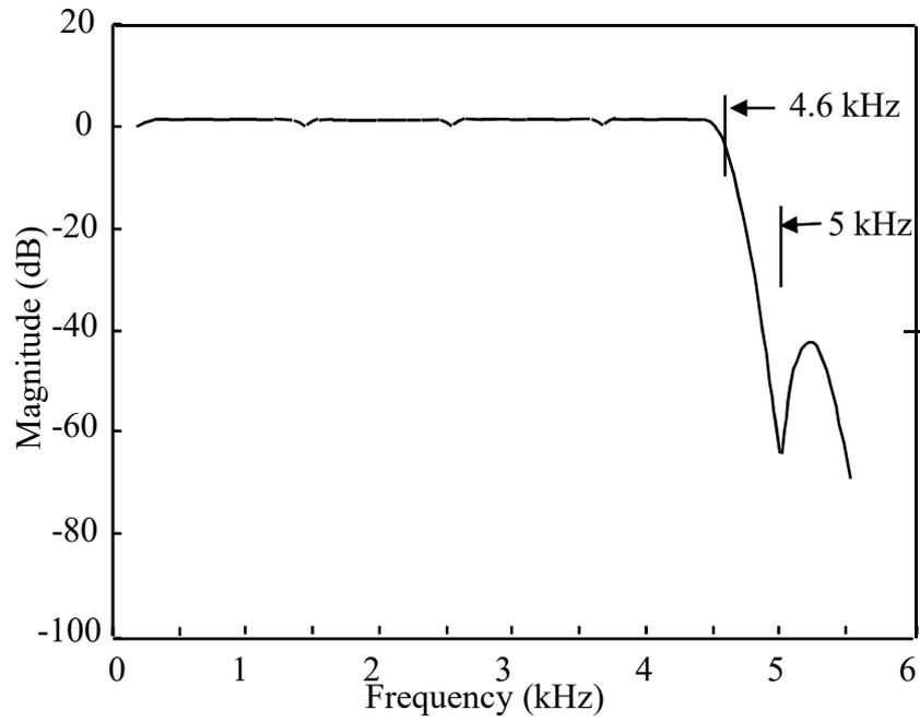
FIG. B.1 The measured magnitude response of the 7<sup>th</sup> order active elliptic low pass filters. The pass band ripples  $< 0.3$  dB. The stop band attenuation  $> 40$  dB.
