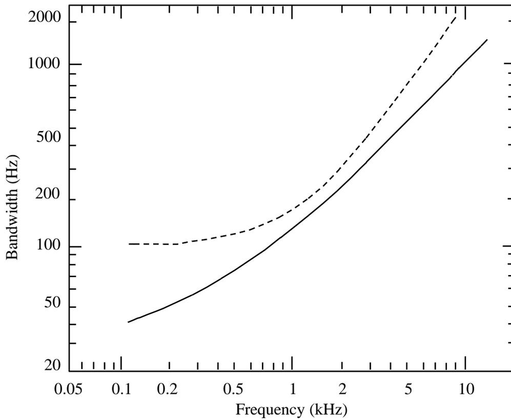
FIG. 2.6 Critical bandwidth as a function of center frequency of auditory filter. The dashed curve shows the traditional estimate (Zwicker, 1961), the solid curve gives more recently obtained estimate of equivalent rectangular bandwidth. Adapted from Moore 1997 Fig. 3.10.
