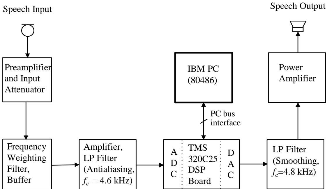
FIG. 4.9 Experimental setup for acquisition and analysis of speech segments.
