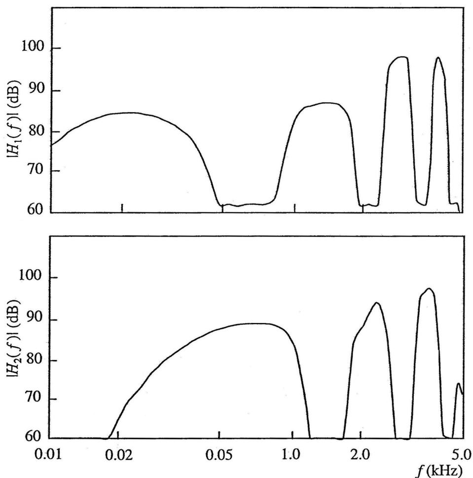
FIG. 3.2 A schematic diagram and magnitude response of the digital processor for dichotic presentation developed by Lunner *et al.* (1993). Schematic is based on the description given in Lunner *et al.* (1993) and Lunner and Hellgren (1991). Waveform  $s(n)$  is the input and  $s_1(n)$  and  $s_2(n)$  are the output waveform for presenting to the two ears.  $|H_1(f)|$  and the  $|H_2(f)|$  are the magnitude responses for the two channels.
