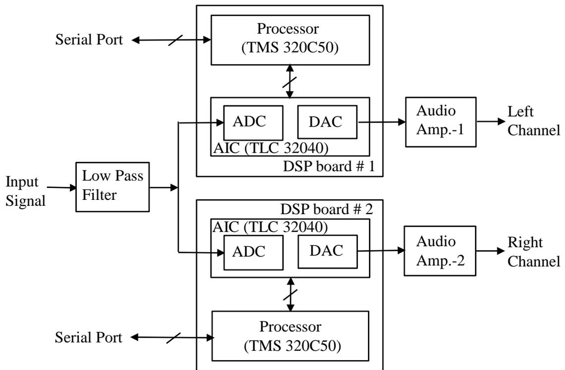
FIG. 5.1 Speech processing set-up using two TI/TMS320C50 based DSP boards for dichotic presentation.
