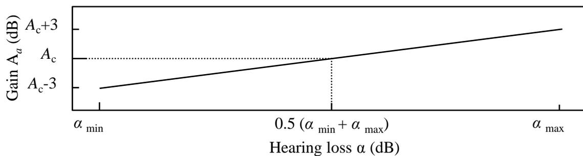
FIG. 5.2 Relationship between filter gain and hearing loss, used for frequency dependent gain compensation in PS-AG implementation.
