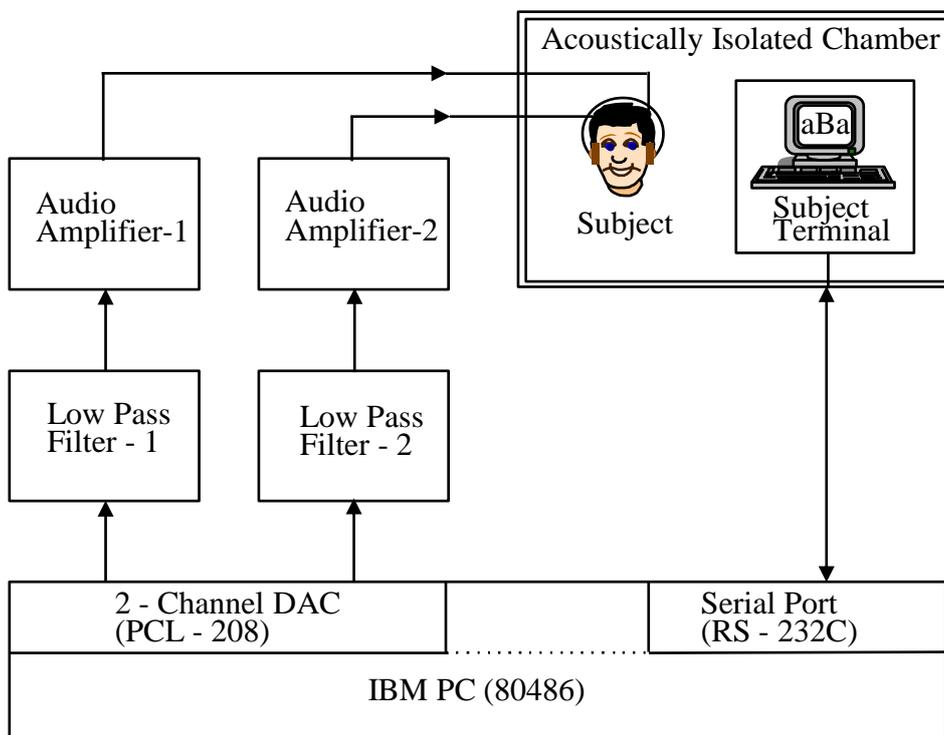
FIG. 4.10 Experimental setup used in the computerized test administration system for listening tests in off-line processing.
