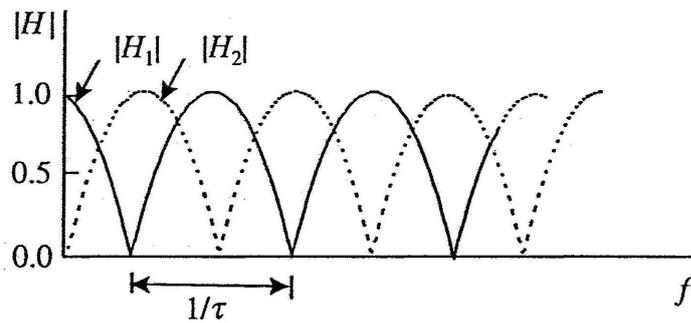
FIG. 3.1 A schematic of the comb-filtering scheme and magnitude response of the filter used by Lyregaard (1982). Waveform  $s(t)$  is the input and  $s_1(t)$ ,  $s_2(t)$  are the output waveform for presenting to the two ears.  $|H_1(f)|$  and  $|H_2(f)|$  are the magnitude responses for the two channels.
