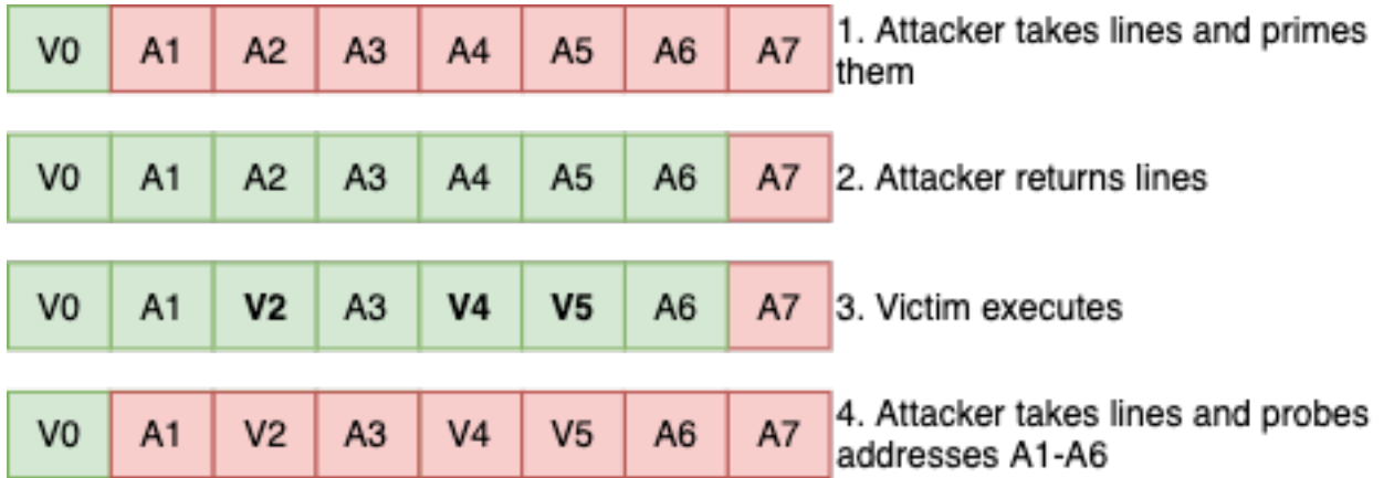
Figure 6.12: Mechanism for Prime+Probe attack
