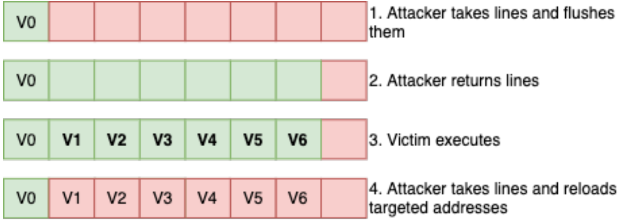
Figure 6.11: Mechanism for Flush+Reload attack
